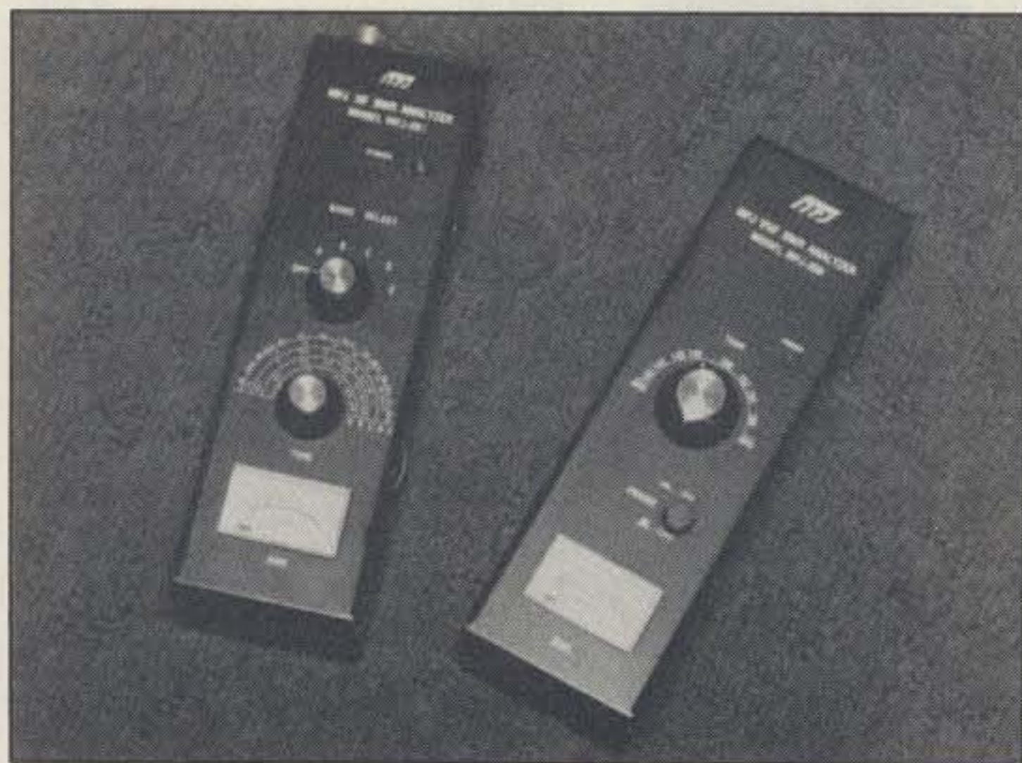
Both units look similar, except the MFJ-207 is bandswitched to cover the bands from 160 to 10 meters.
