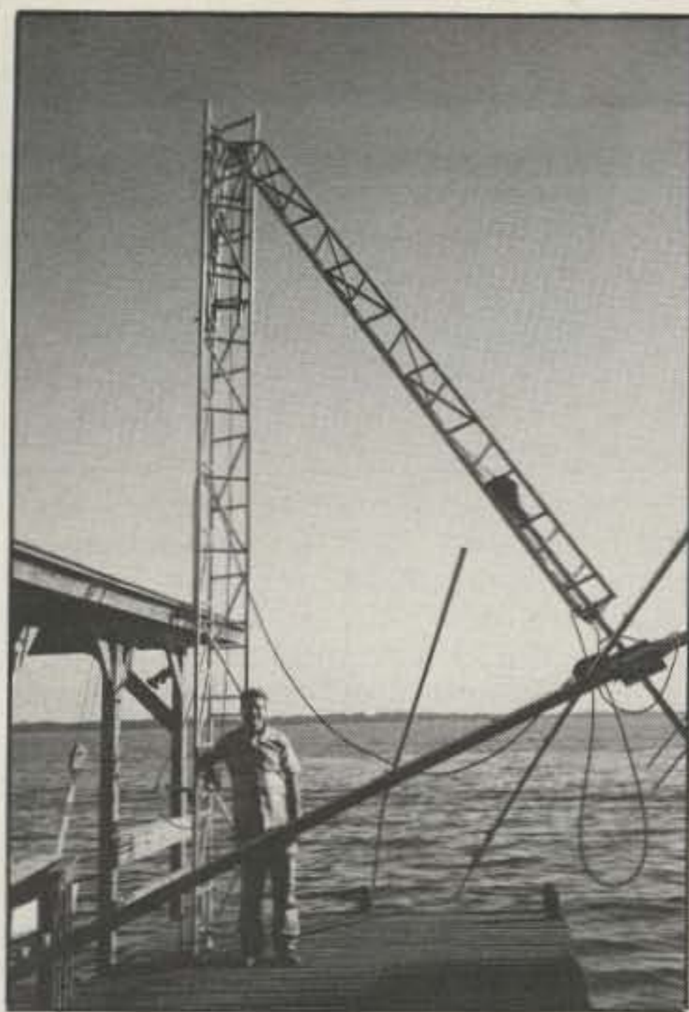
Here's one unlucky amateur, Henry Fehrmann, N4EDQ. Henry arrived home to see his tower was folded in half and twisted, with his tribander and rotor ending up in Lake Eustis. Fortunately, little damage was done to the homes in the area and no injuries were reported from the twister that visited its wrath around the lake. (Photo courtesy N4EDQ)
