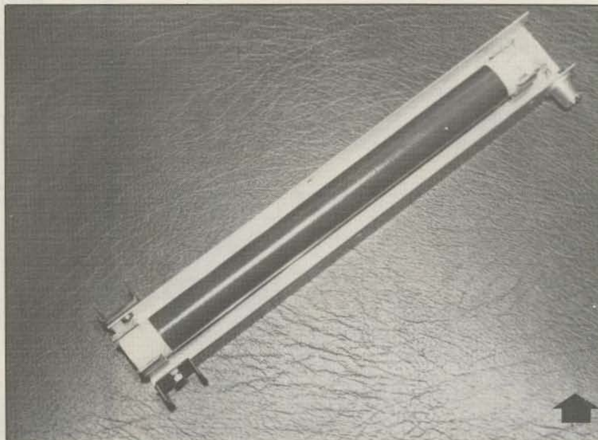
Details are covered in the text, but the dummy load consists of little more than a 12 inch long RF noninductive carbon resistor mounted in a standard-size piece of aluminum channel stock.
