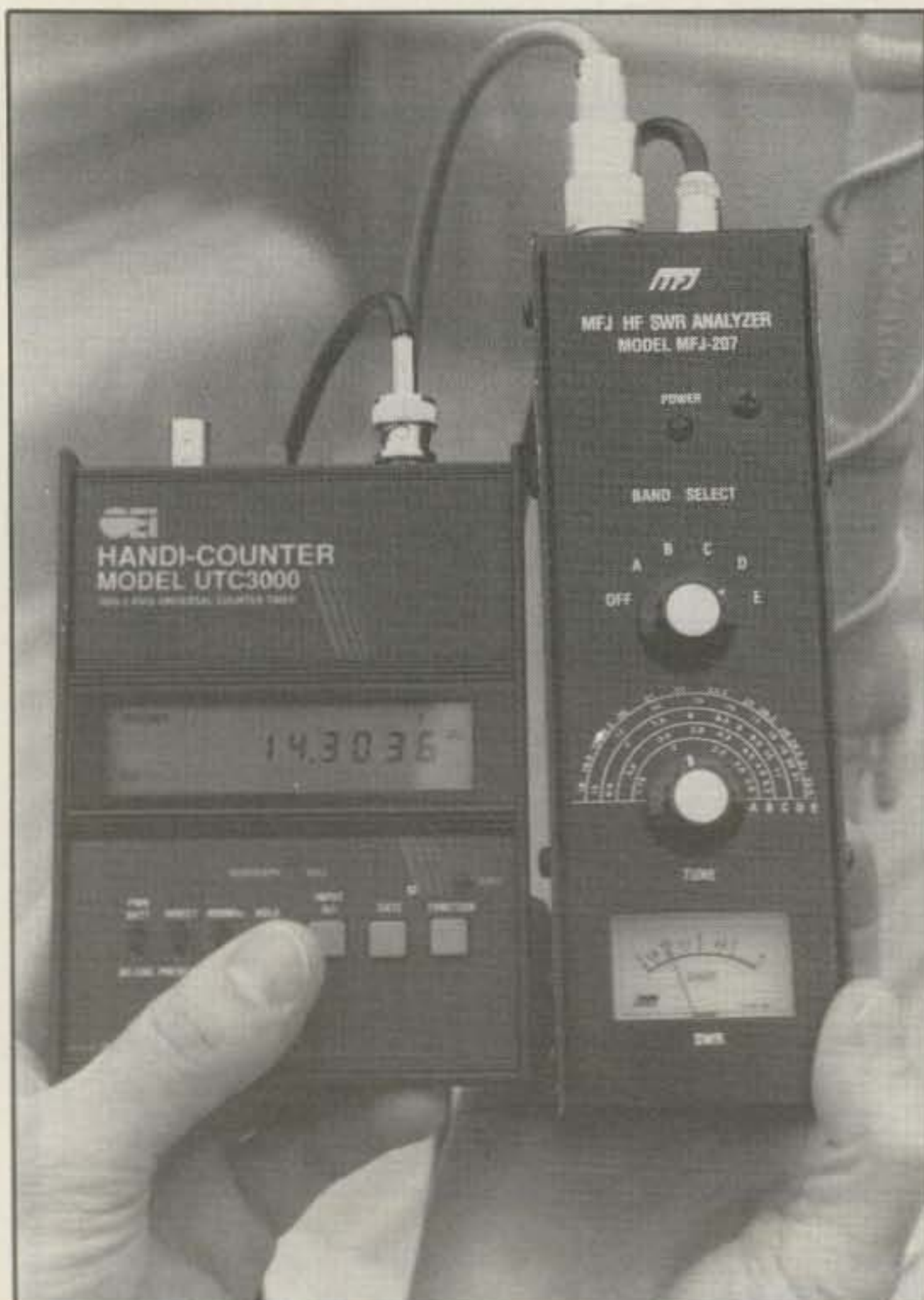
The MFJ SWR analyzer sends out a signal to be read by the Optoelectronics frequency counter.
