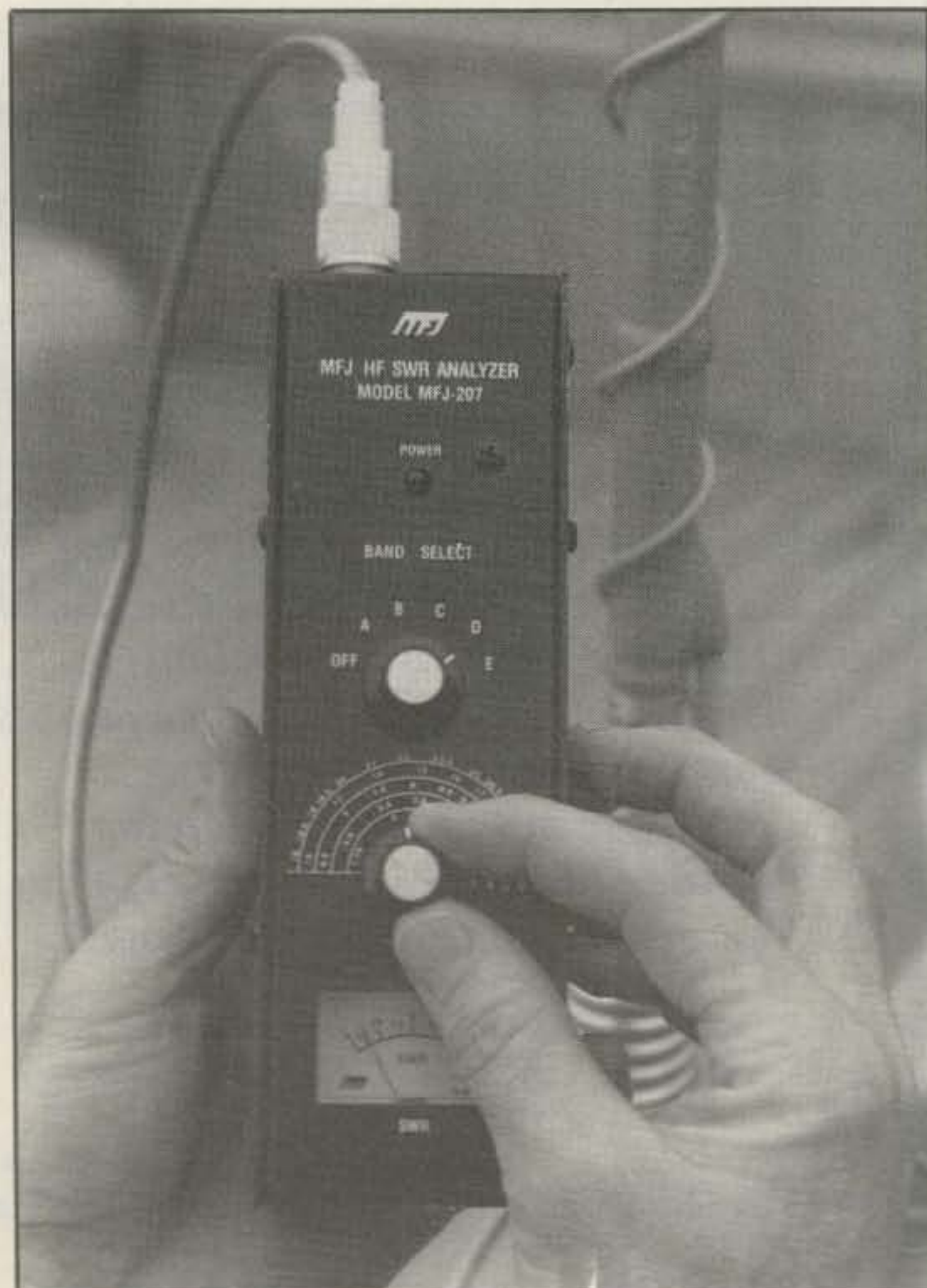
Changing the frequency on the MFJ unit lets you check to see where your HF whip is cut.
