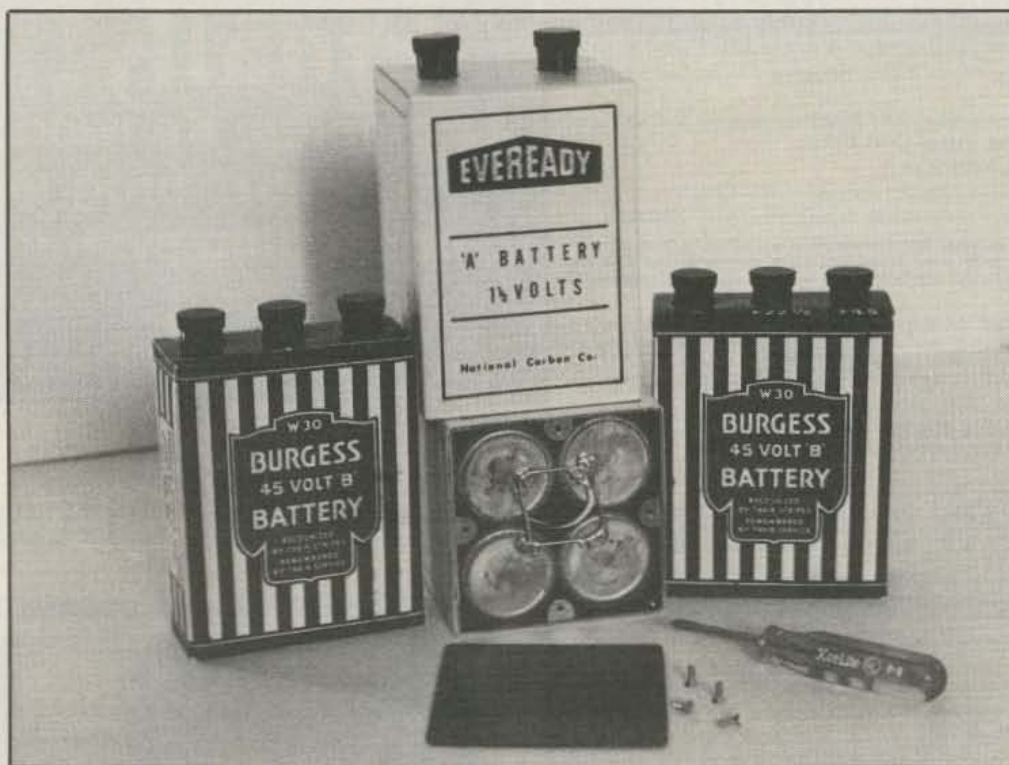
Fig. 3—Arnold Sayre's homebrewed batteries for Crystal Hartley and other rigs. Standard 1.5 and 9 volt batteries are mounted in cases with slip-off covers made with photocopies of original-era items.
