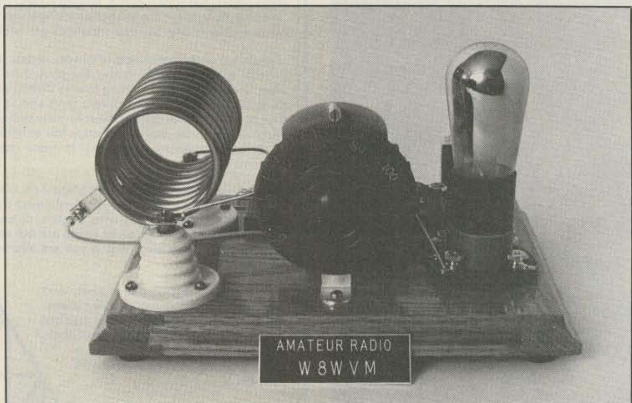
Fig. 2—Front view of W8WVM's Crystal Hartley transmitter. Copper tank coil sits on beehive insulators, clip connects to antenna terminal on rear, tuning condenser is hidden by large dial, and crystal is in the right back corner. This beautiful gem runs 2 watts on 30 or 40 meters.
