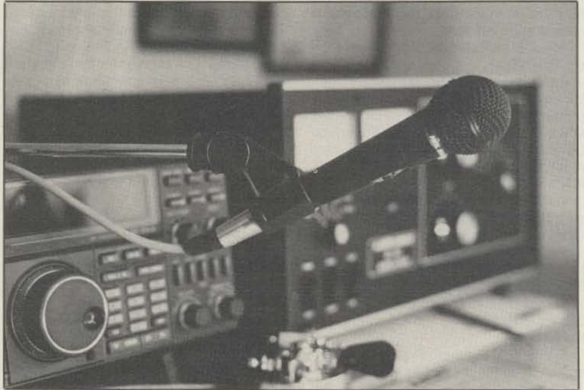
Fig. 1—The Heil HM-10 microphone is tops in audio quality. It is available with an HC-4 and/or HC-5 element as discussed in the text, or you can substitute an older HC-3 element for either element. Mic shown with optional AB-1 boom at K4TWJ.
