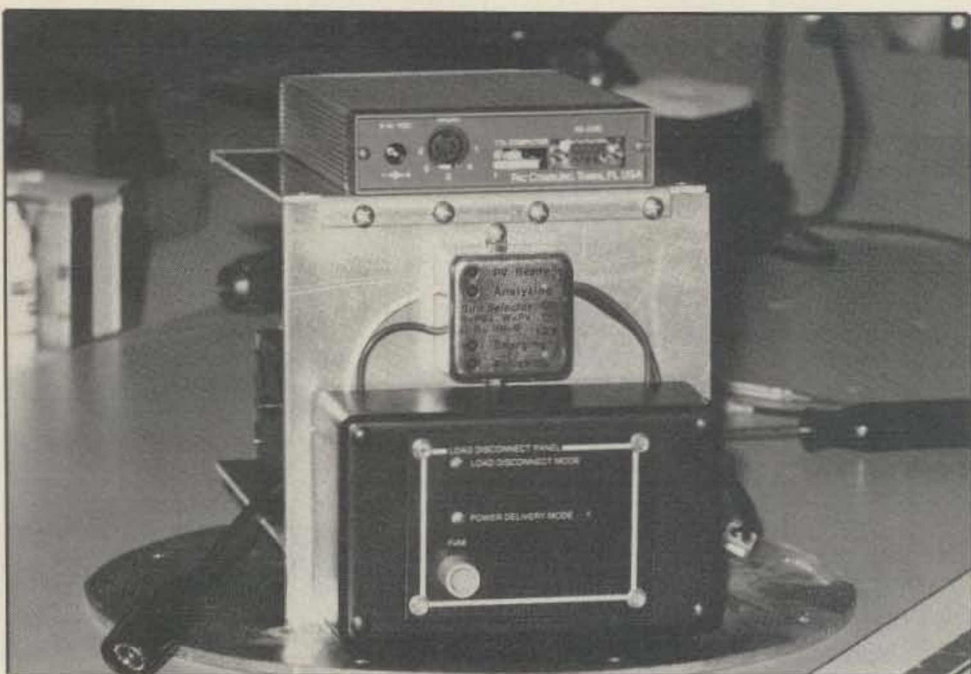
Photo B- The LD-15 Load Disconnect, shown at the bottom of the photo, is used to ensure that the transceiver and TNC (load) do not discharge the batteries below the preset level of 11.5 volts, or approximately 25% of the battery capacity.
