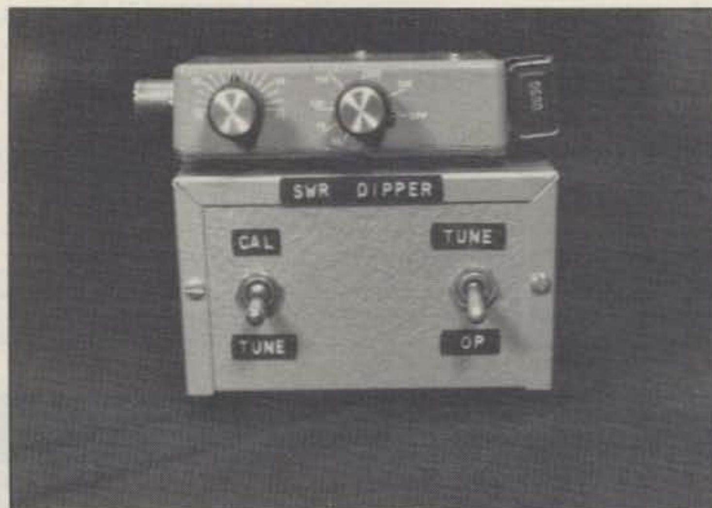
My Palomar RX Noise Bridge is held to the control box with a strip of Velcro®
