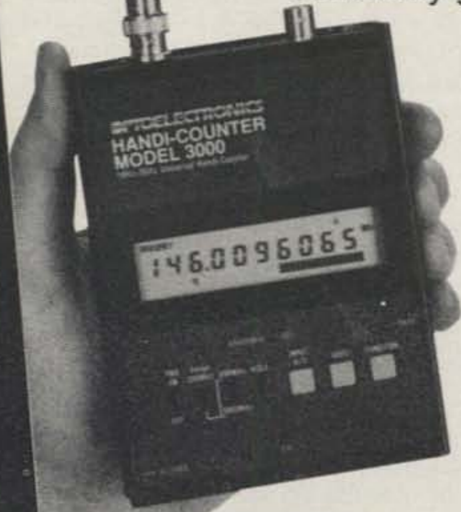
MODEL 3000 Multi-function Counter 10Hz-3GHz, 10 Digit LCD with frequency, period, ratio, interval & signal level bargraph....$375.
