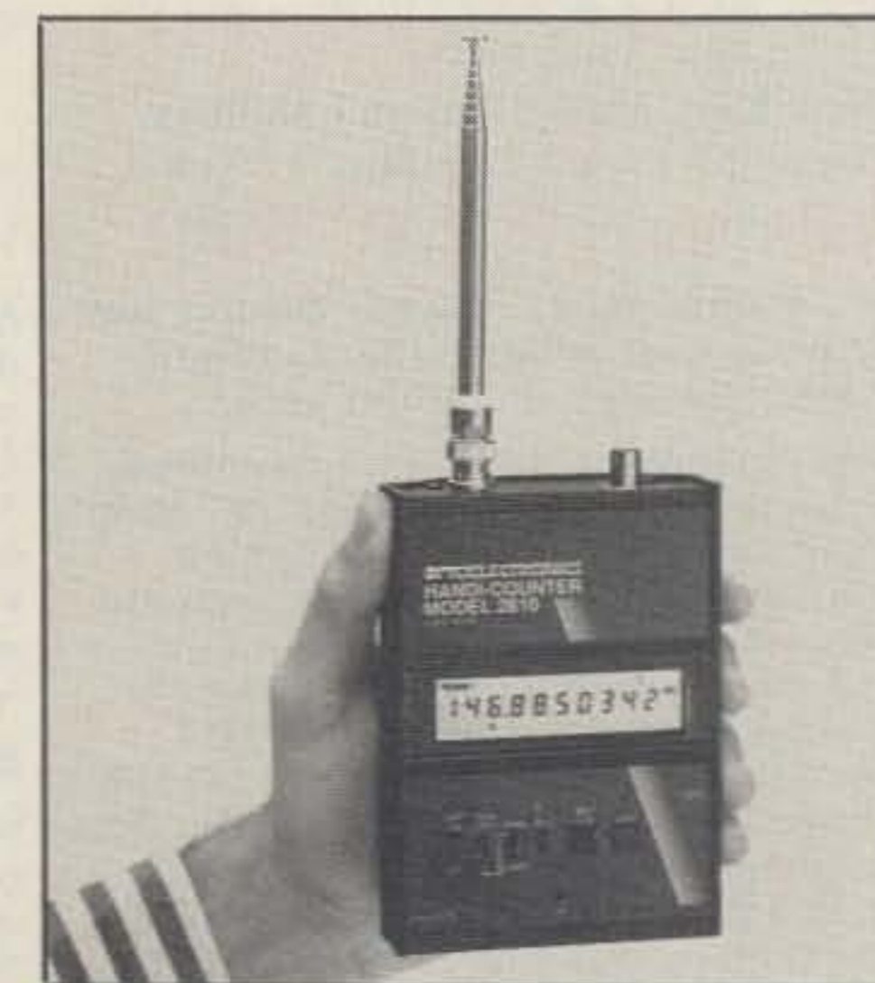
Photo 8—Whether tuning antennas, setting crystal-controlled VHF rigs on frequency, or working with class rigs, a digital frequency counter is super handy. Optoelectronics' Model 2810 shown here is exceptionally accurate and on sale this holiday season. Go for it!
