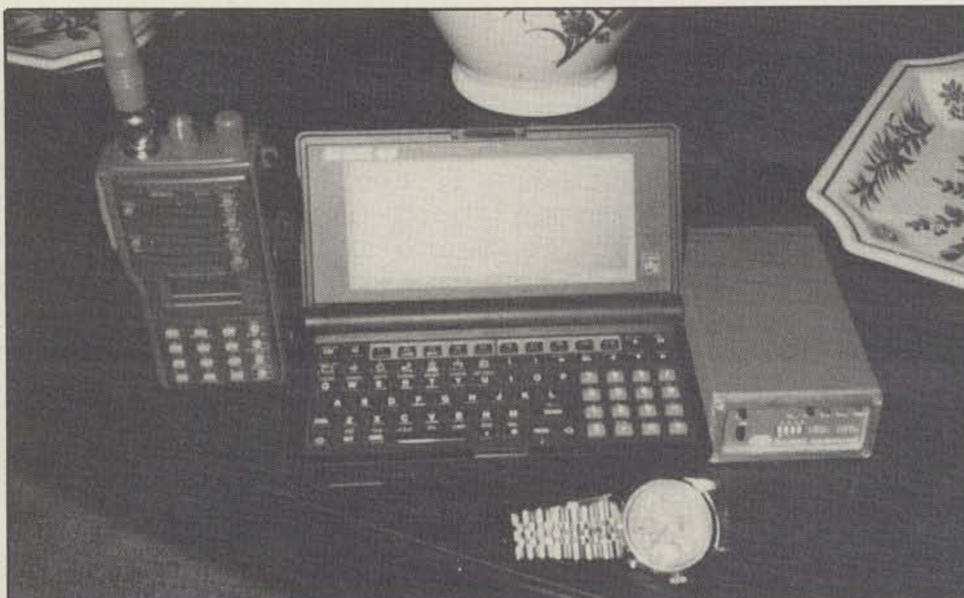
What do you get when you combine an Alinco F1 with a HandiPacket and the Hewlett-Packard 95LX? Another HP ("Hip Pocket") packet station! The Rolex is optional.
