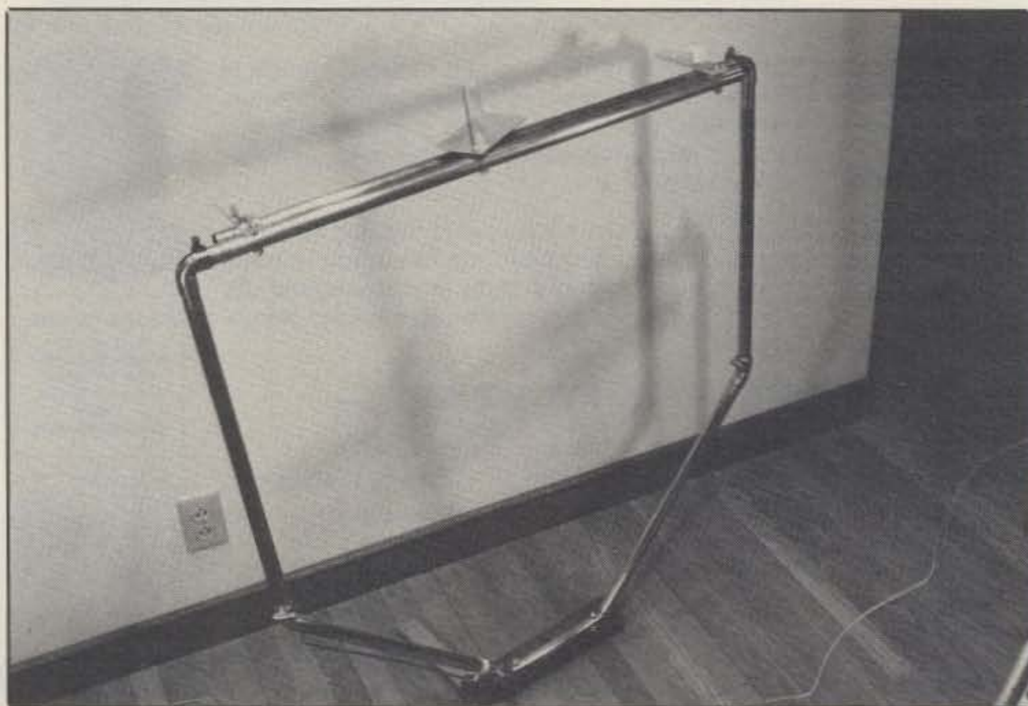
Fig. 1—The 20–10 meter transmitting/receiving loop antenna. The tuning capacitor is the top of the loop, between the two parallel lengths of copper pipe.
