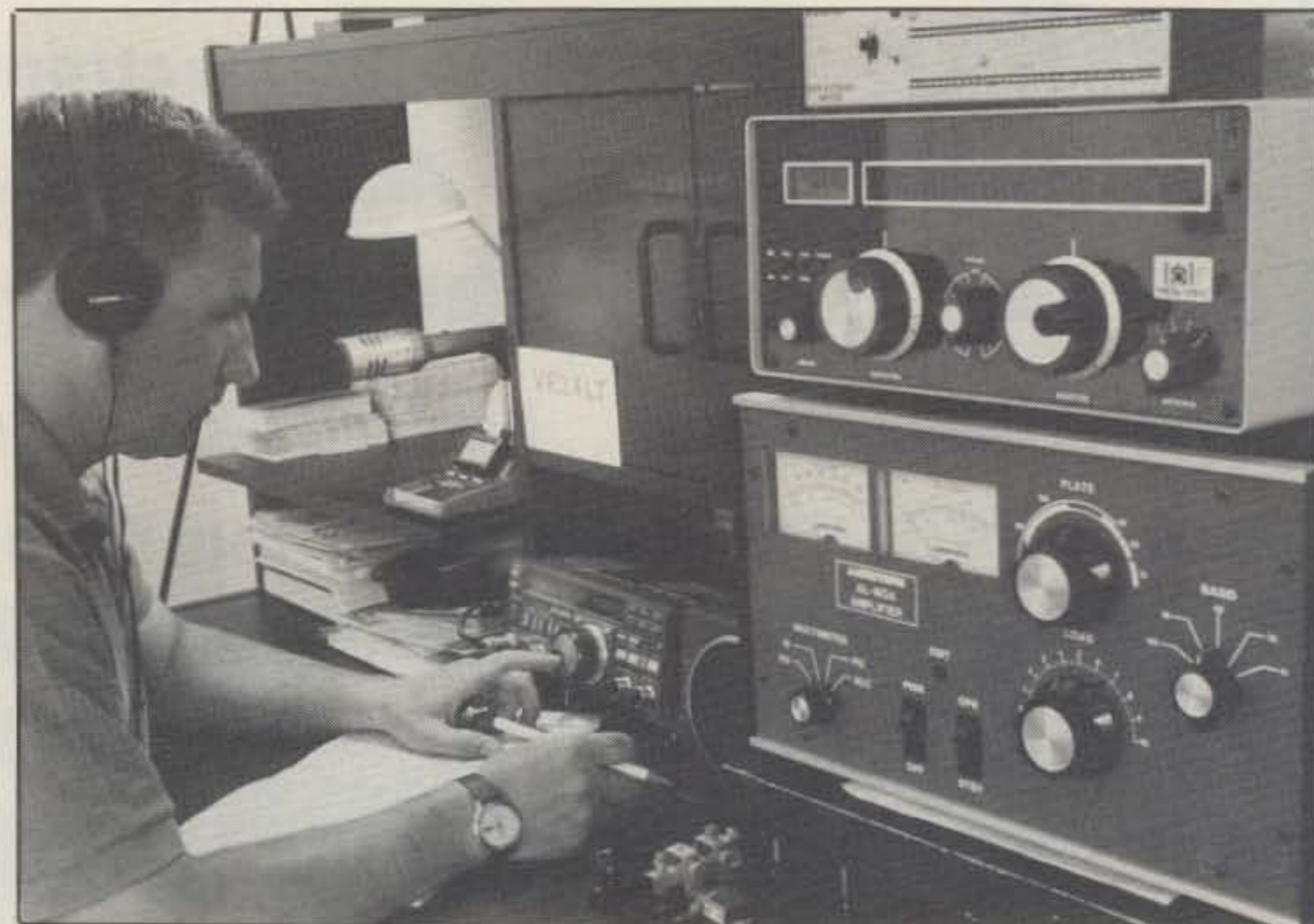
Yuri Dzyuba, VE2XLT, of Montreal, Canada, held UB5LT in the Ukraine during 1966 to 1970. He immigrated to Canada in 1989, sponsored by VE2SEI. His station includes Yaesu FT-757GX transceiver, Cushcraft R-5 vertical, and a Canadian Windom. Despite the Ameritron AL-80A linear amplifier included in this picture, Yuri makes many 3 watt (QRP) trans-Atlantic contacts.
