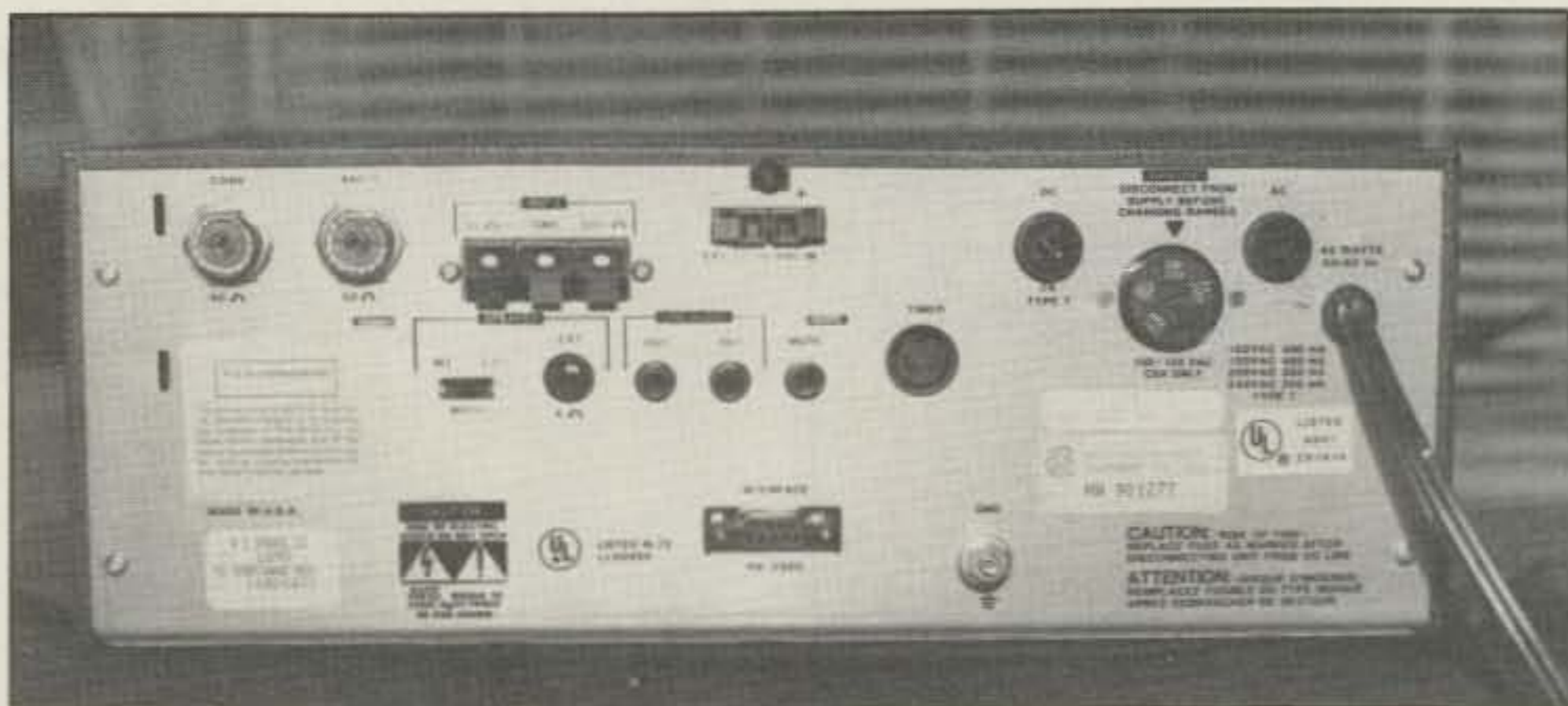
The rear panel contains a variety of connectors for external interfaces, including computer control, but it is generously dimensioned.
