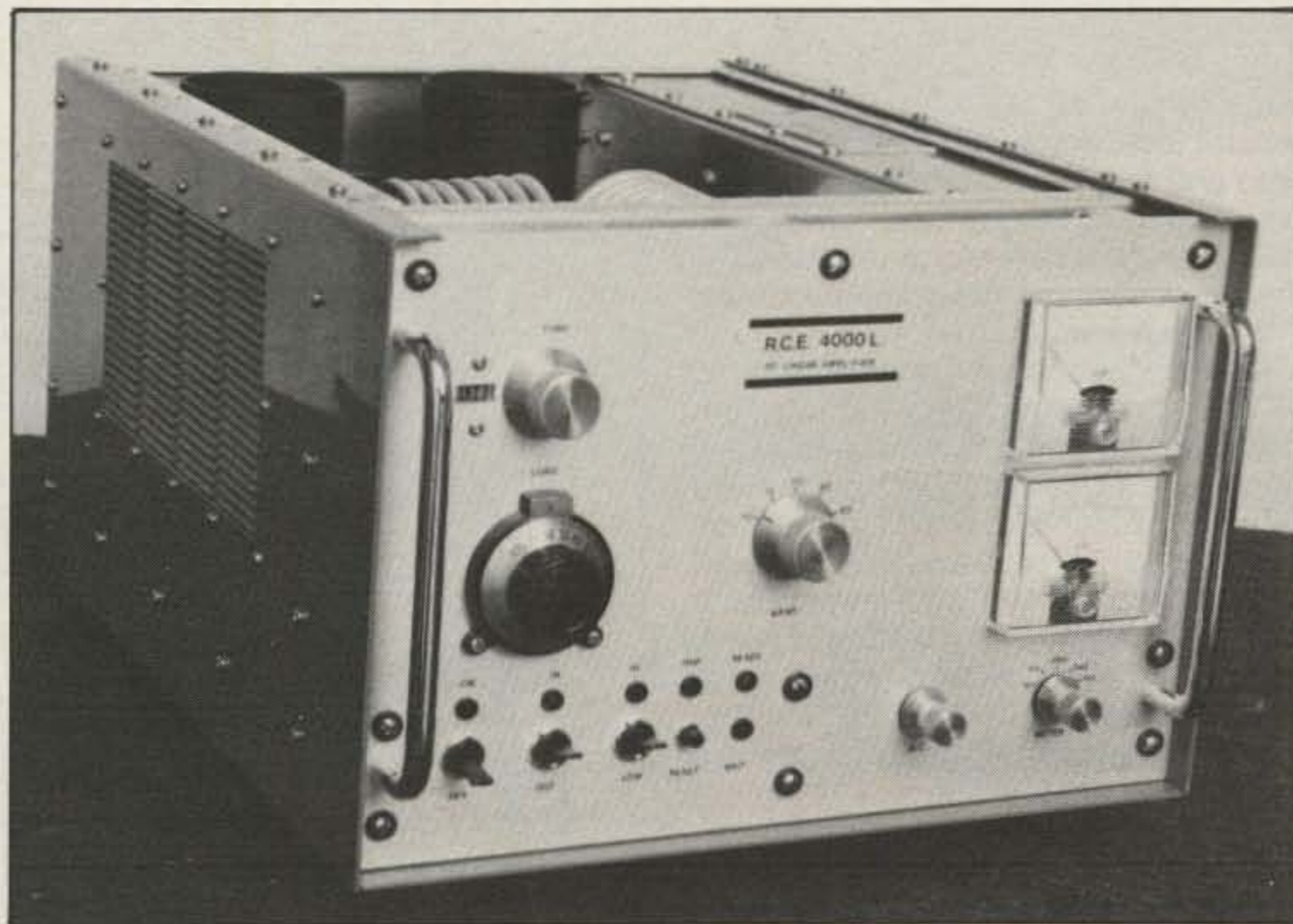
Fig. 6—Front view of the completed amplifier. The top left control is the turns-counter dial for the Tune capacitor. Below that is the vernier drive associated with the Loading capacitor. The handles are surplus from another project. Operational controls and indicating lights are grouped at the lower left. The two small controls at the lower right are ALC Adjust and the multimeter switch. The bandswitch is in the center of the panel. The top meter measures plate current and the lower one is the multimeter. The front panel was completely wire-brushed prior to lettering. This view also shows clearly the details of the RF switch (center).
