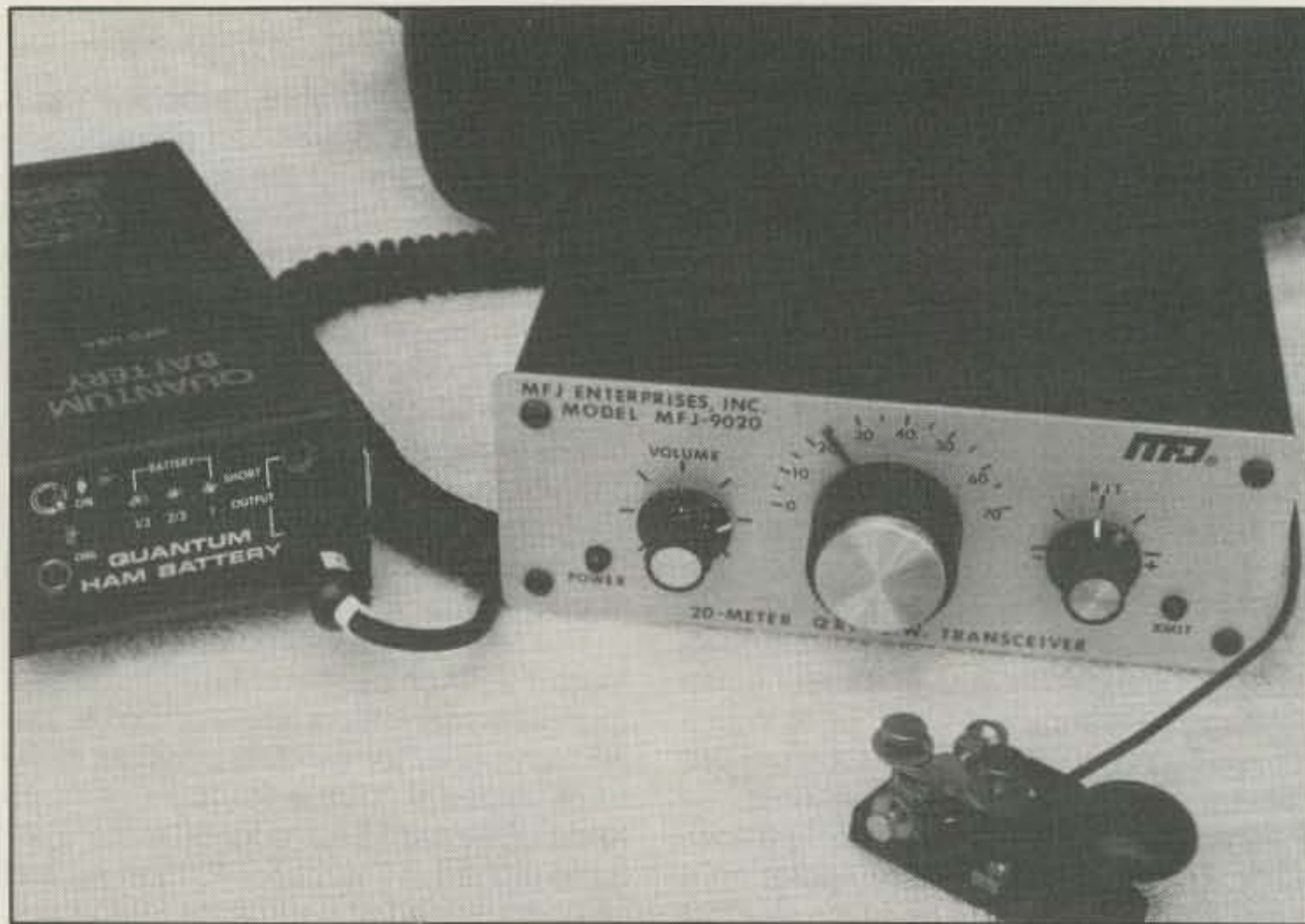
Fig. 5- A totally portable and high-performance QRP station. MFJ 20 meter transceiver is flanked by Quantum Ham Battery. Shoulder bag behind it carries both units plus miniature spy key (from K4TWJ collection).
