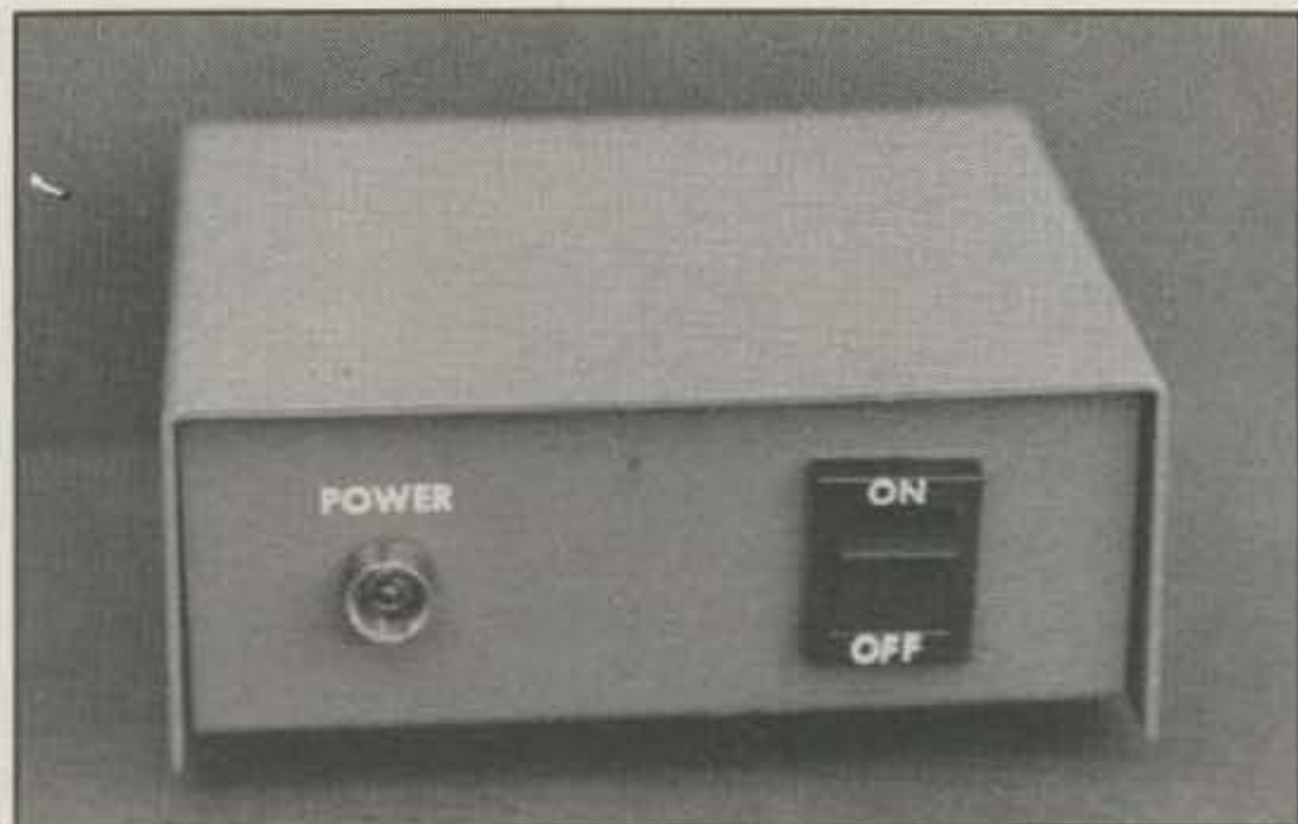
Front view of the interface. The LED indicator is on the left, and the power switch on the right. (Photos by Peg, KE2NP)
