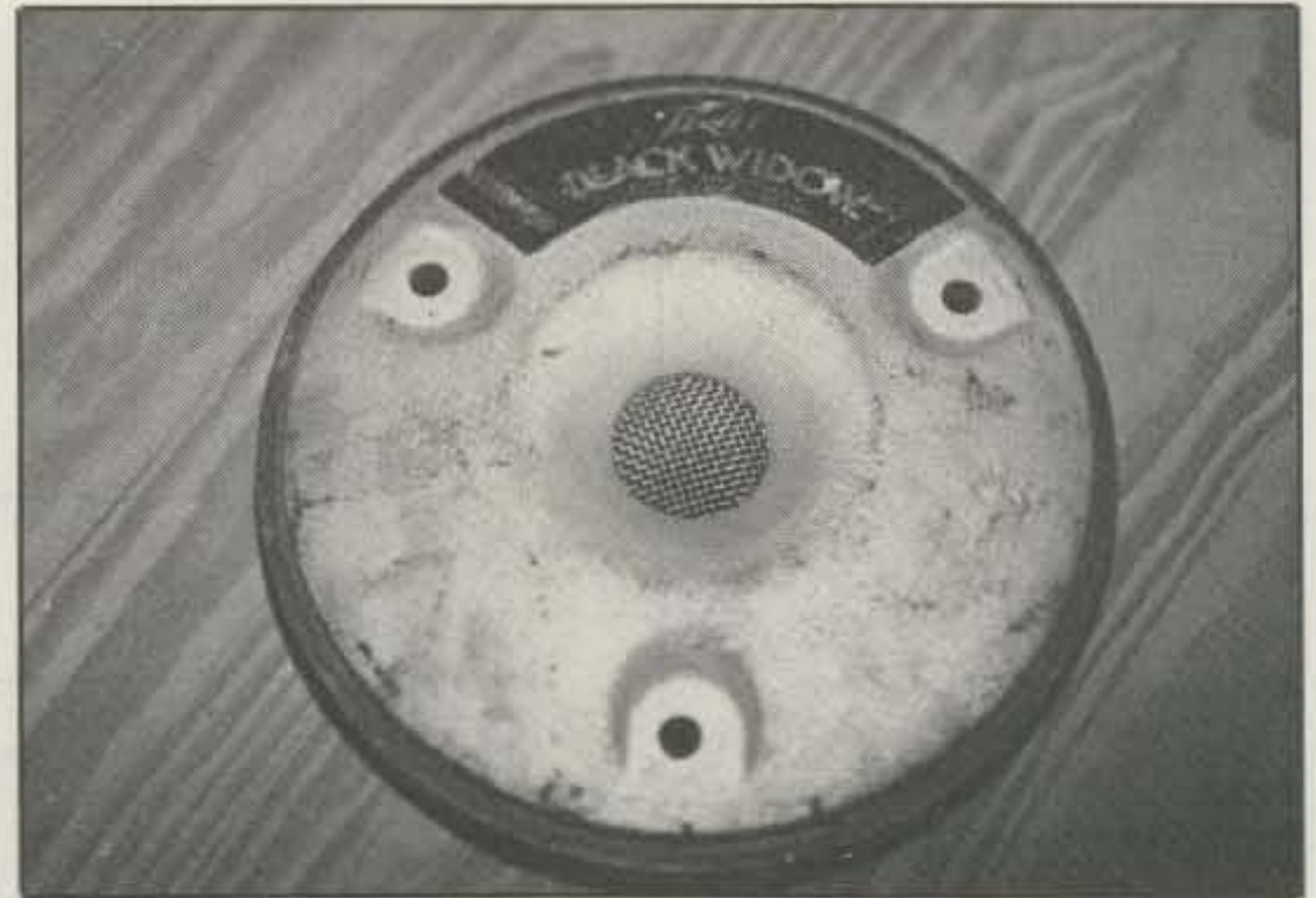
The Black Widow speaker magnet shown after removing the extra hardware and cone.
