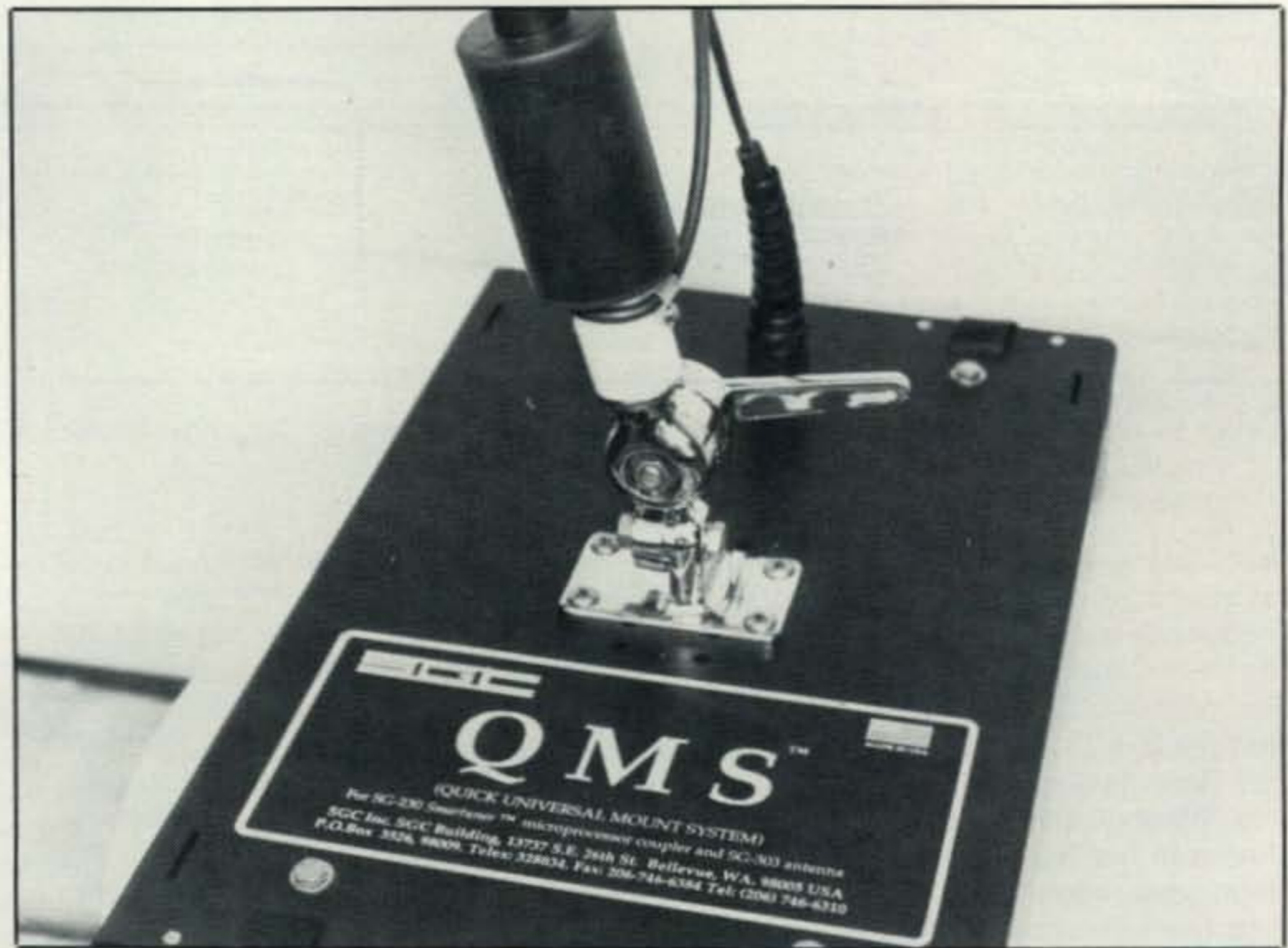
The ratchet-mount base for the SG-303 is massive. A hand grip allows for quick lowering of the antenna.
