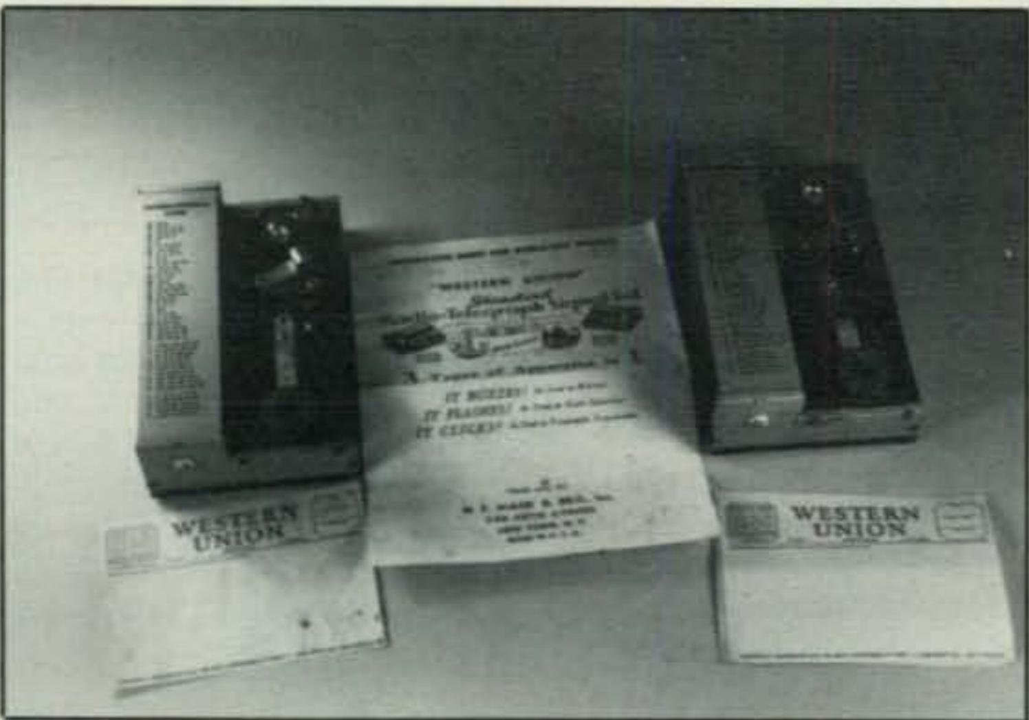
Photo 8— Items inside the Western Union telegraph set include two keys with buzzers and flashers plus neat instructions. (Photo via K1BH)
