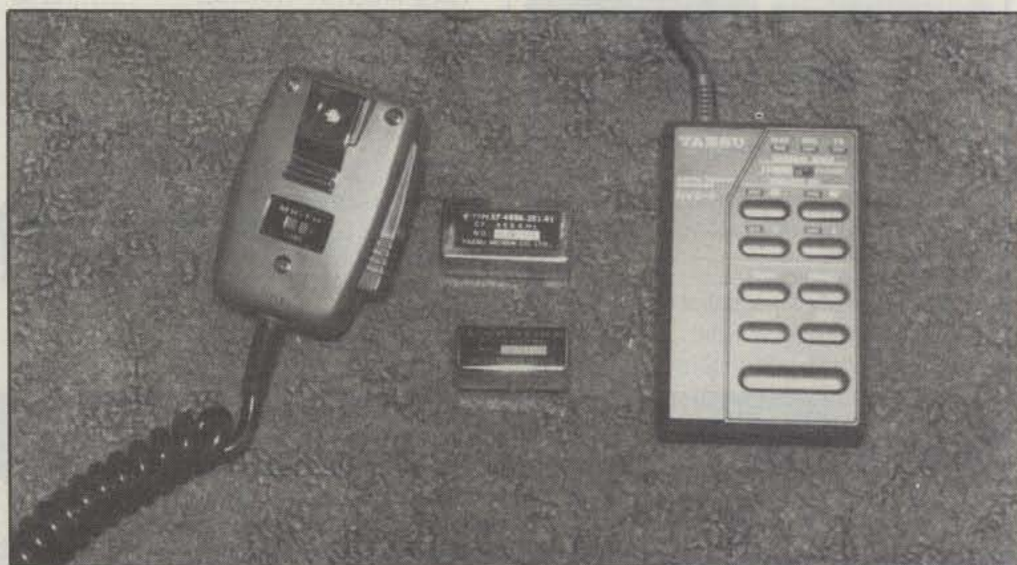
The MH-1 hand microphone supplied with the FT-990, the two optional IF filters, and the optional DVS-2 digital recorder. The back of the microphone is shown to illustrate a small switch, below the clip, which controls an RC time constant which slightly tailors the frequency response of the microphone. There are so many frequency response tailoring possibilities on both the transmit and receive sides in the FT-990 system that it's hard to believe that any operator can't be satisfied.
