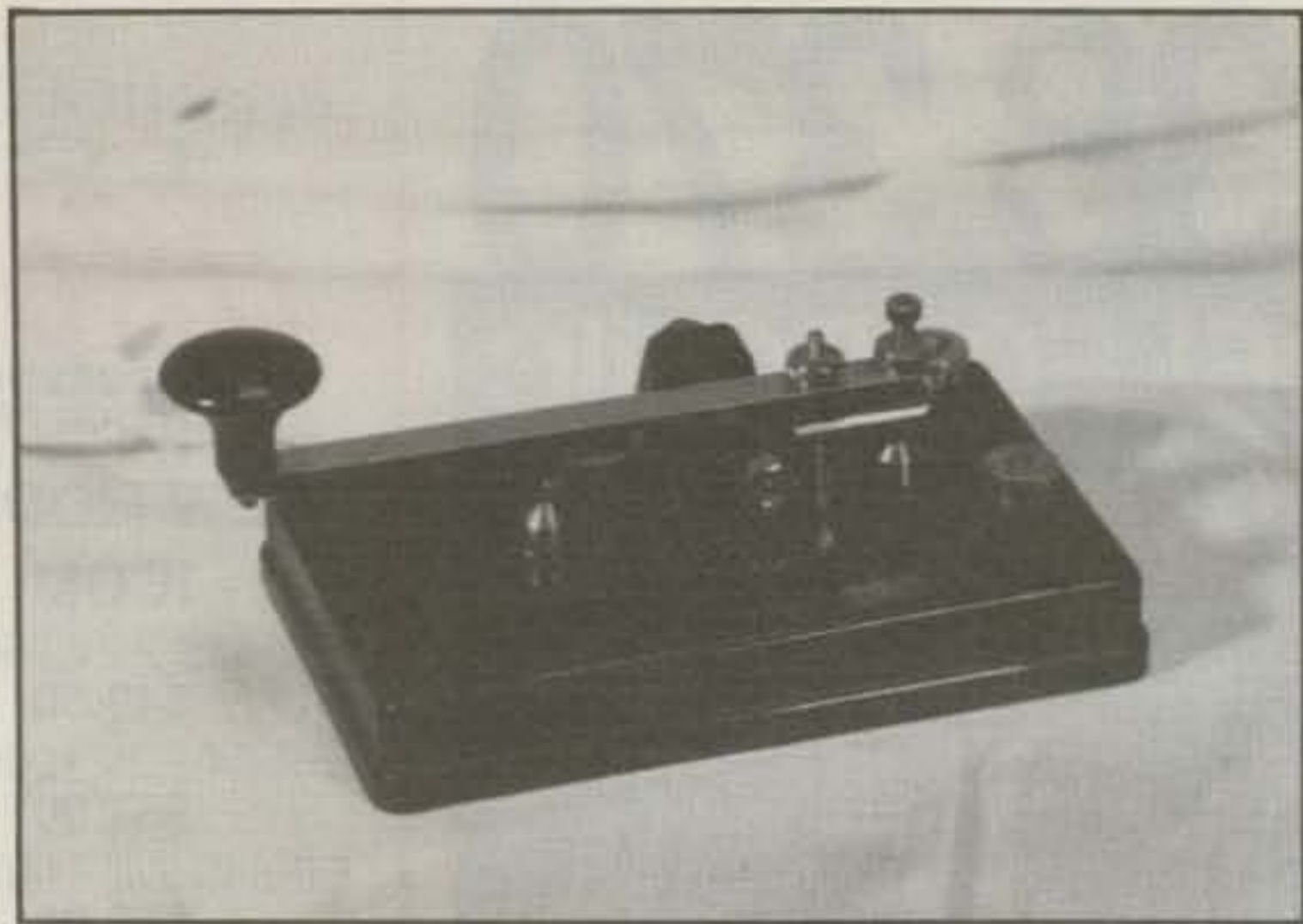
Photo 12- An interesting combination of elegance and simplicity is apparent in this neat Japanese hand key made by Sato Company. Its small adjustment screws have very fine threads, and pivot adjusting screws are set into locknuts at the fulcrum. Owner WB0AUQ did not tell us how the key feels during use, but judging by its workmanship, I would say it's a gem.
