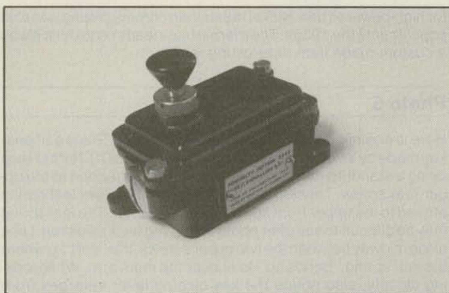
Photo 8- Sparton of Canada Ltd. made this waterproof key during 1943, and it is a delightful little gem. All adjustments are internal; thus it should be ideal for portable operating at the beach or maritime mobiling. Miniature keys such as this are a real treat to use on the air today, but finding them continues to be a real challenge. (Key owned and photographed by VE7FOU)
