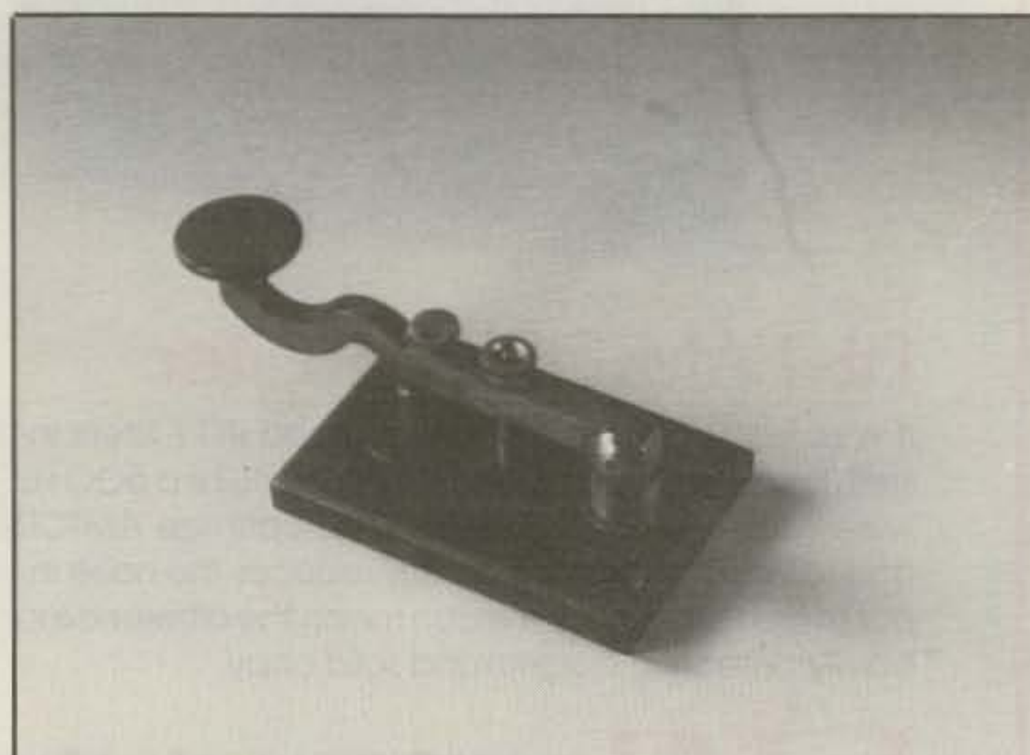
Photo 3— German-made Zimmerman Leipzig camelback made during the late 1800s. Notice rear support and simple, yet effective design. Cone-shaped adjustment nut often carries over to modern designs in German keys. (Photo courtesy K1BH)
