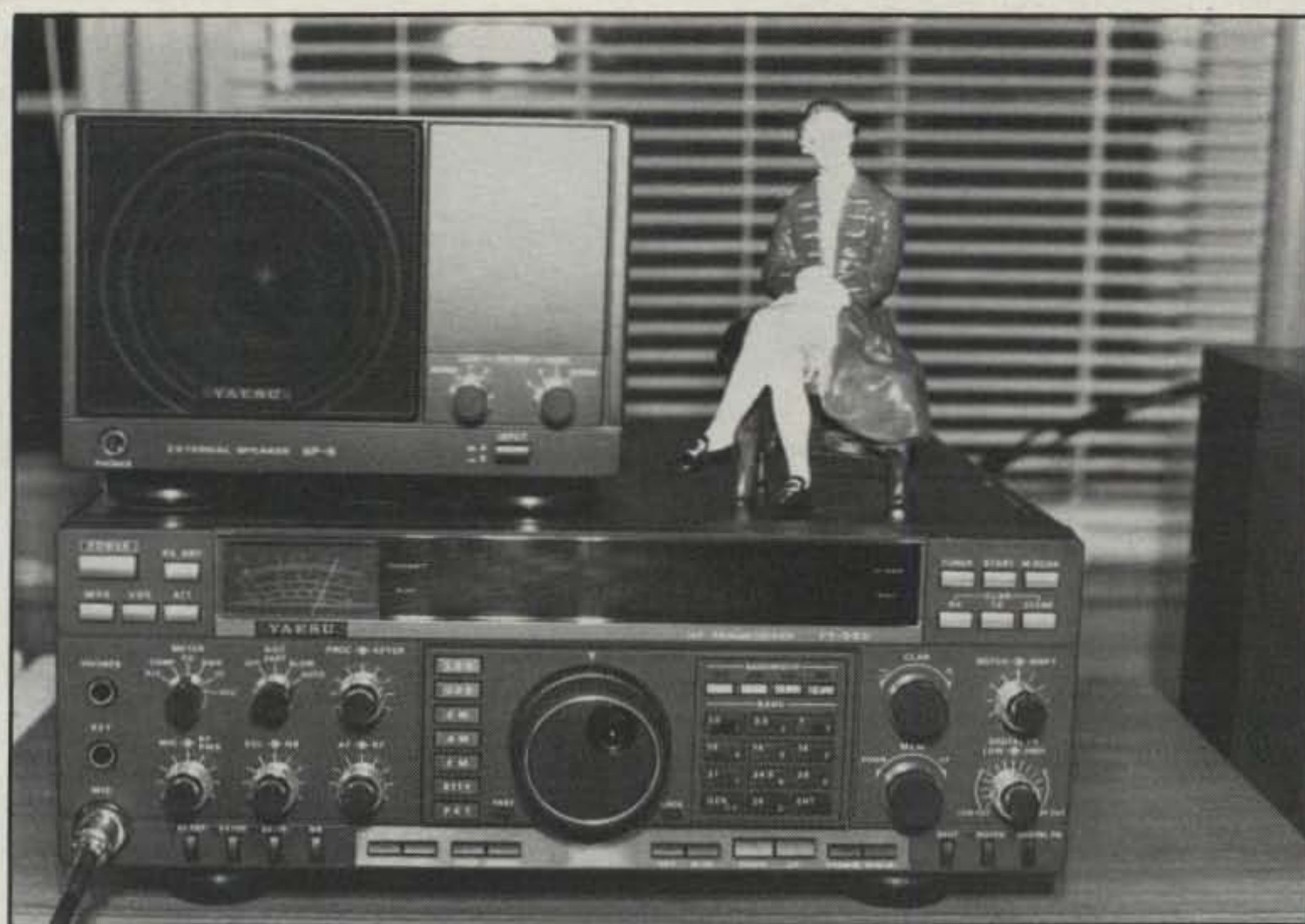
The FT-990 with the SP-6 optional speaker unit. The "Gentleman from Williamsburg" on the right is exactly 6 inches high, for size comparison.
