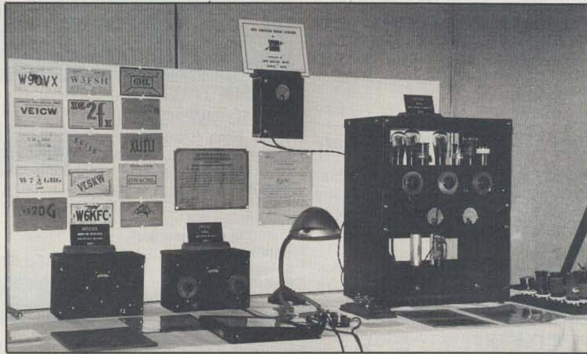
Complete "Gross" station reconstructed by John Rollins, W1YG. Jerry Gross, W2AAE, had a big amateur radio store on "Radio Row" in New York City. Station monitor at left, shortwave receiver center, and CW version of the "46 job" at right. Antenna tuner is mounted on wall.
