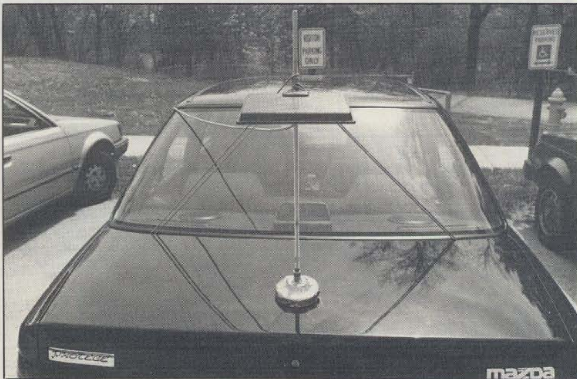
I used my SQLOOP antenna at the Dayton Hamvention by mounting it on the back of my rental car. This is a fun antenna! (See the text for more information on the SQLOOP antenna.)
