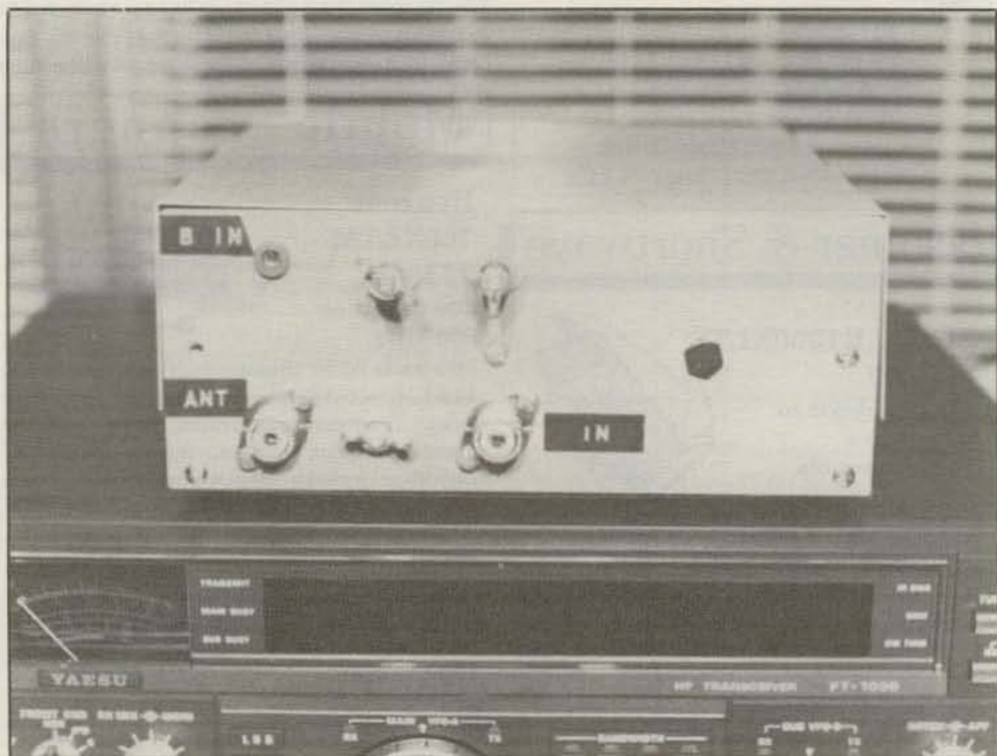
The rear panel of tuner #2. A plug-in jumper is used between "ANT" and "B IN" when the balanced line output is used.
