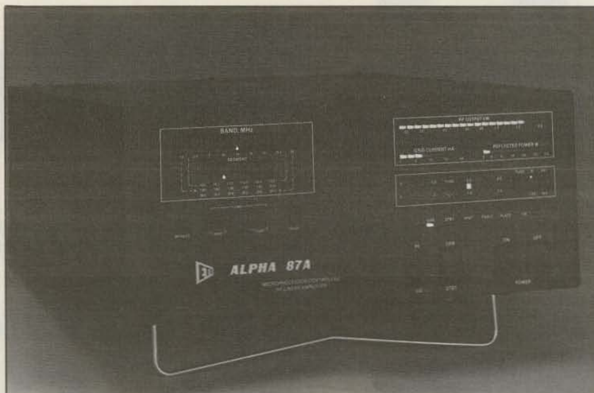
The front-panel view of the Alpha 87A. At the upper right are the bargraph displays. Frequency and band entries are at the upper left.
