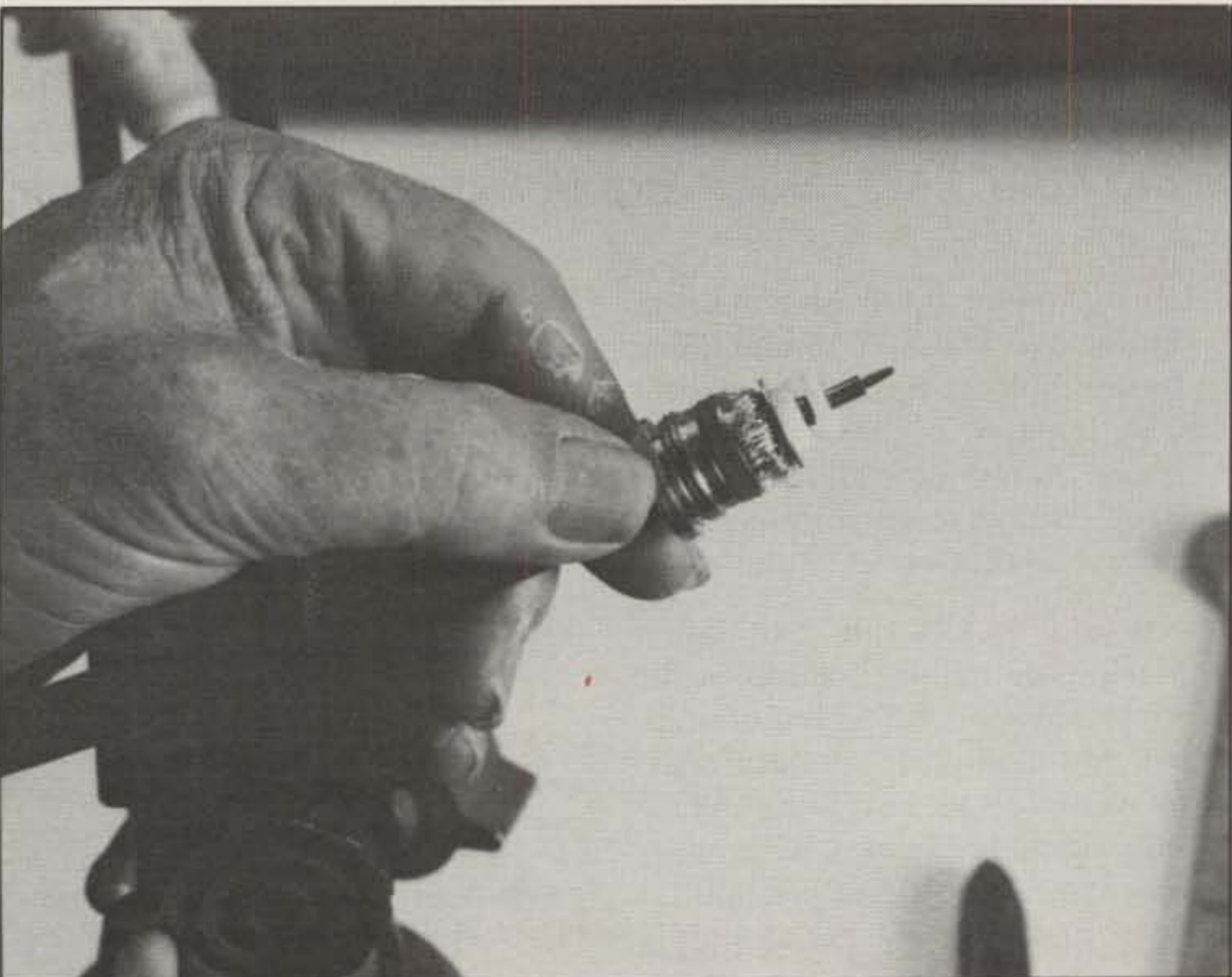
Photo 7—Finished prep ready for outer shell. You need to be able to see the metal shoulder of the center pin between the two Teflon™ washers.
