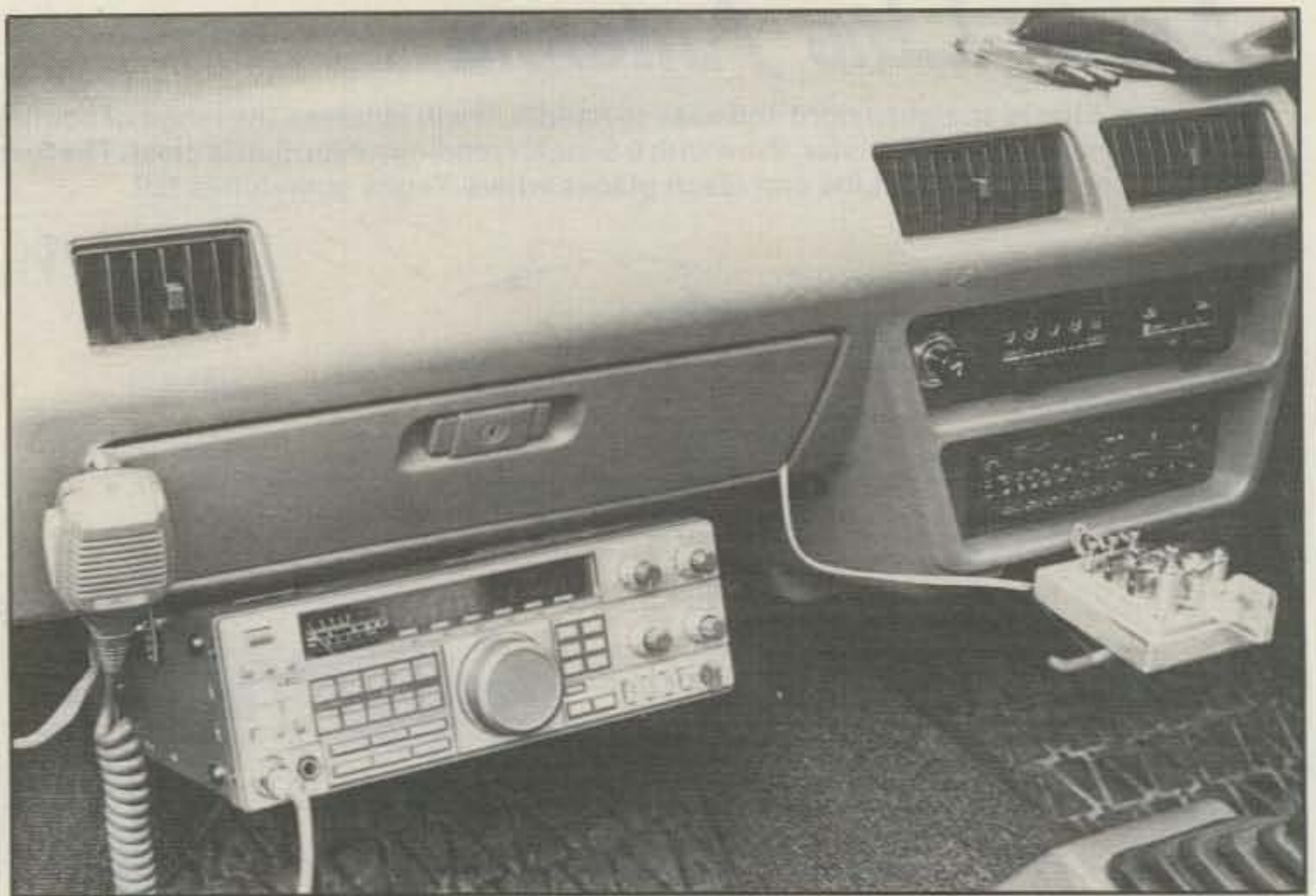
Photo 2- Mobile installation of G4ZAU in his Nissan Micra. When studying this neat installation, remember the steering column is on the right-hand side so Dudley must key with his left hand while also shifting gears.
