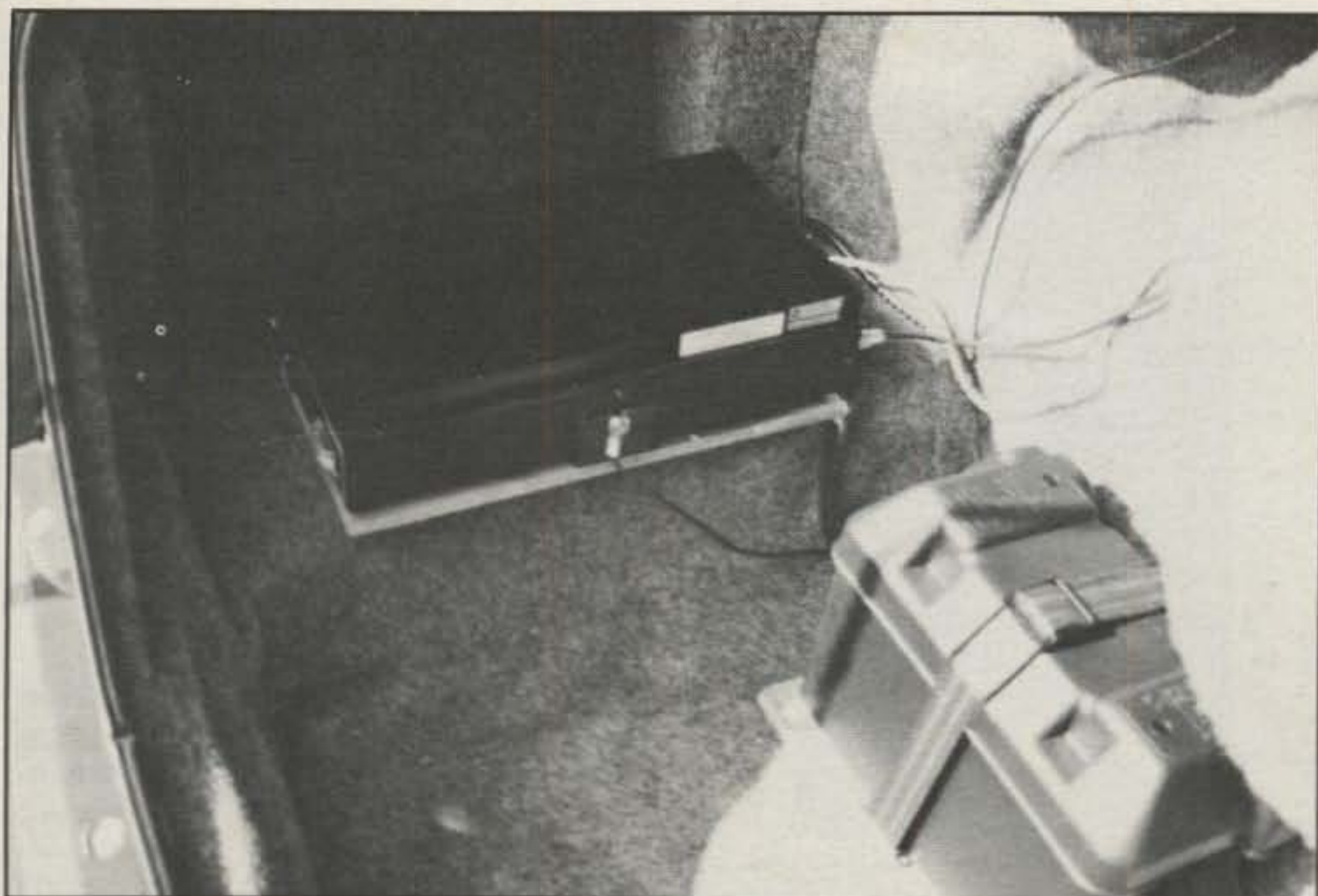
Photo 4- In-trunk view of N4XLL's kilowatt mobile amplifier and high-current marine battery. Large-diameter cables connect these items to front engine compartment. (Discussion in text.)
