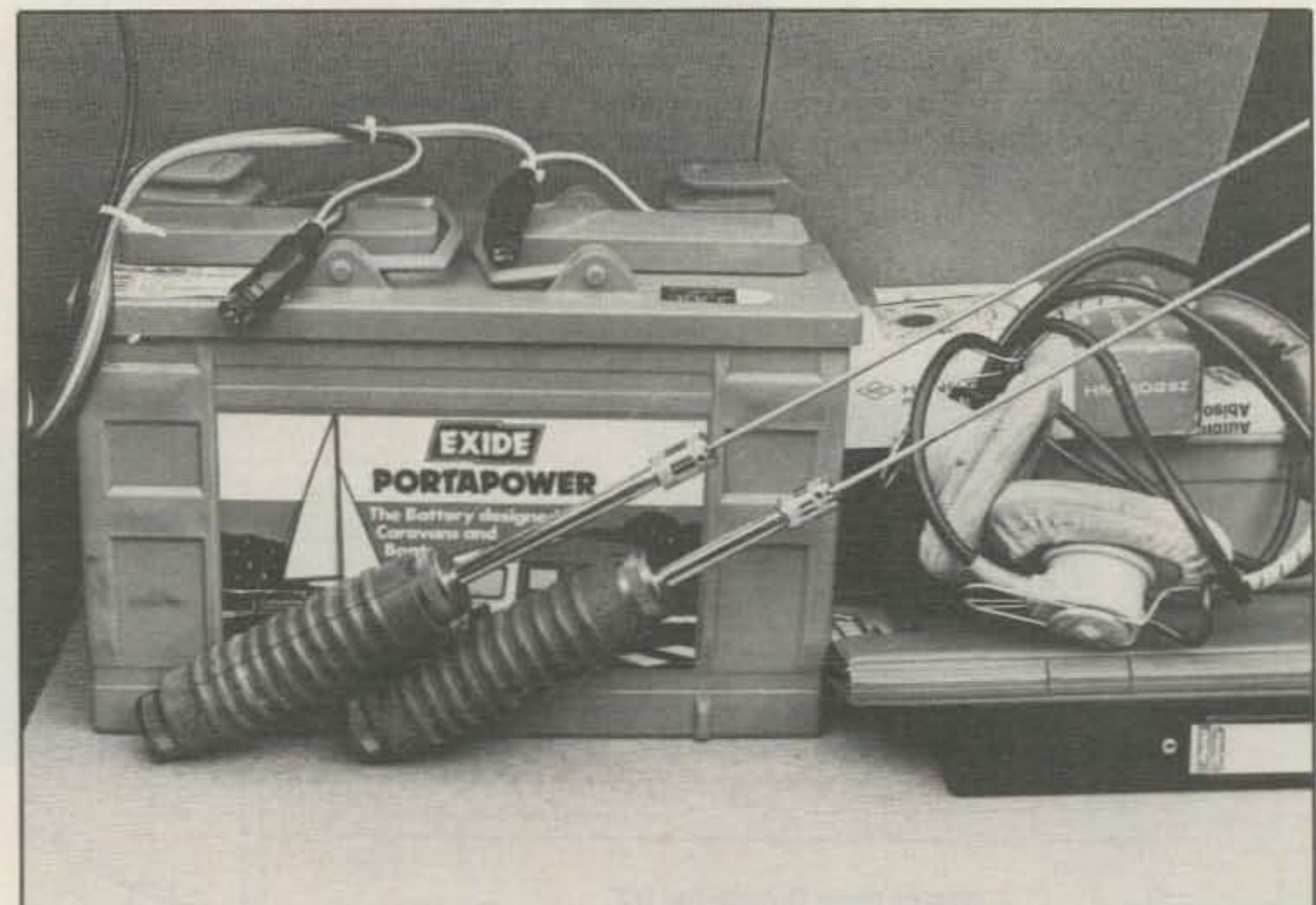
Photo 3- During inactive times G4ZAU stores his mobiling gear behind the car's rear seat. Shown here are his earphones, 90 amp battery, and 6-band NAVY antennas.
