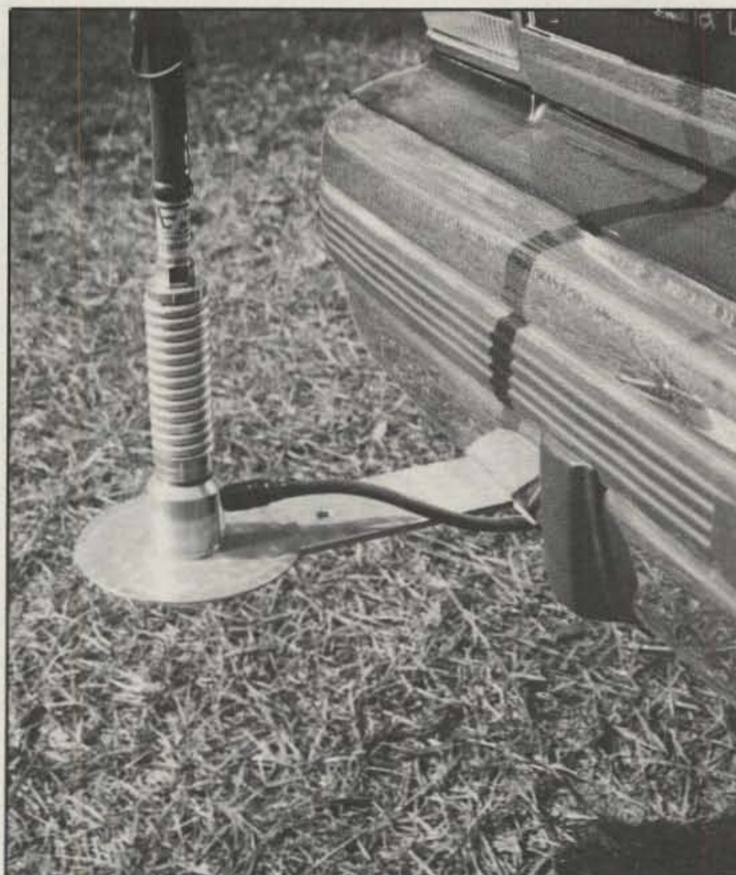
Photo 6- Close-up view of base mount for N4XLL's antenna. Large, circular disk helps impedance matching.
