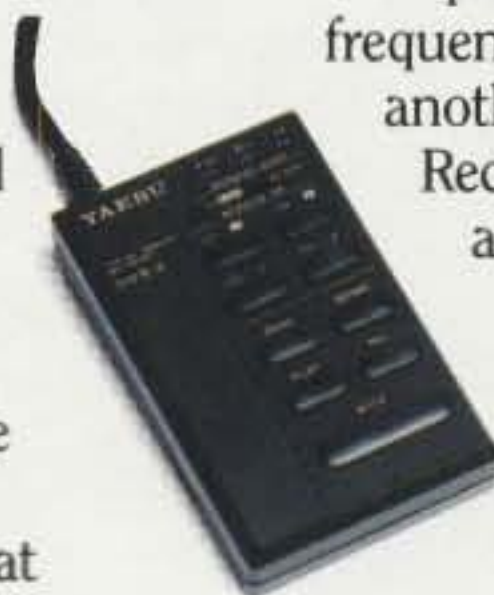
DVS-2 Optional Digital Voice System provides instant playback.
