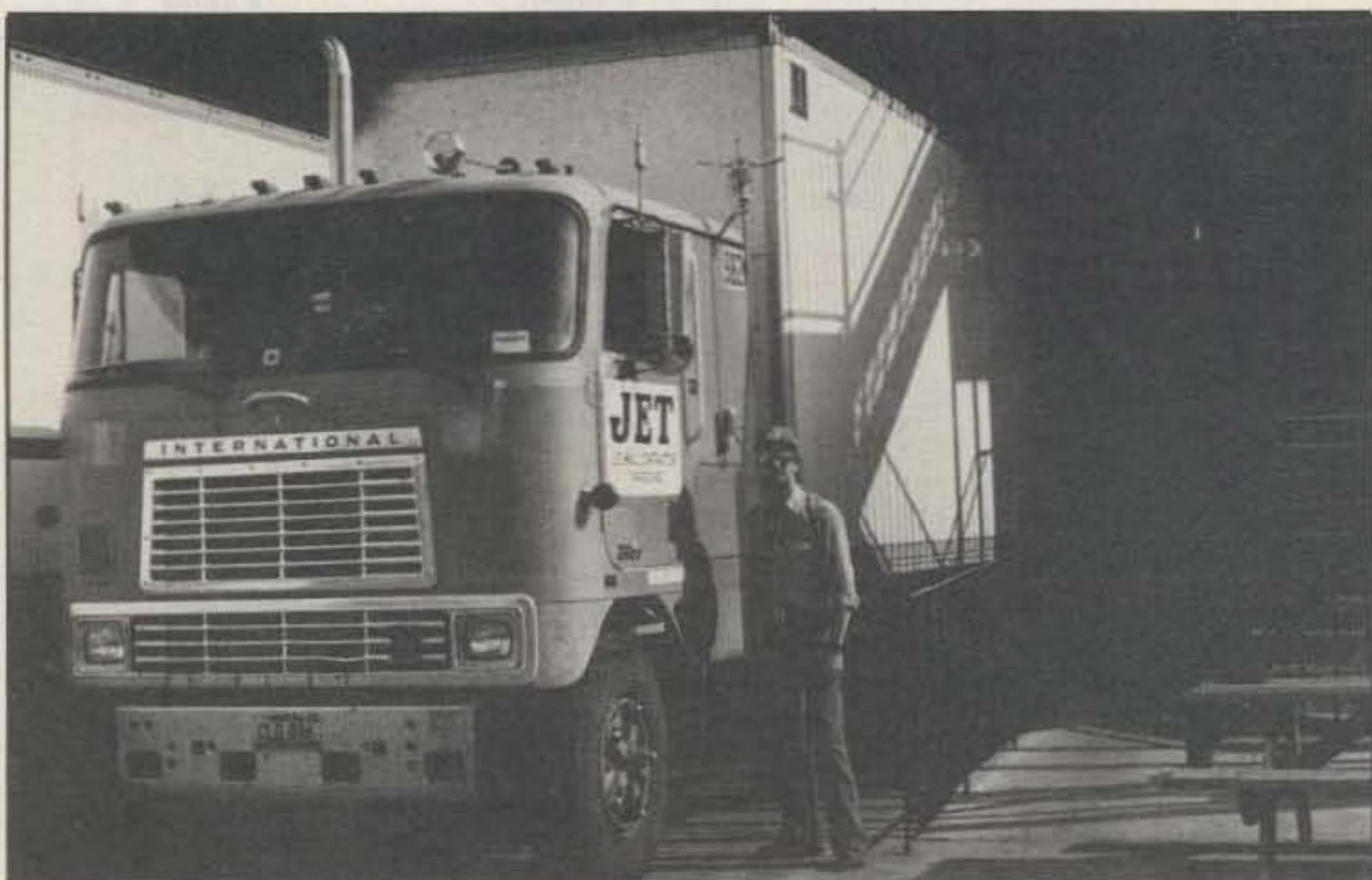
Photo 1—Jon, KA0ZFX, beside his super mobile. Bugcatcher antenna is mounted behind driver's door. Truck and trailer make a very effective ground system!
