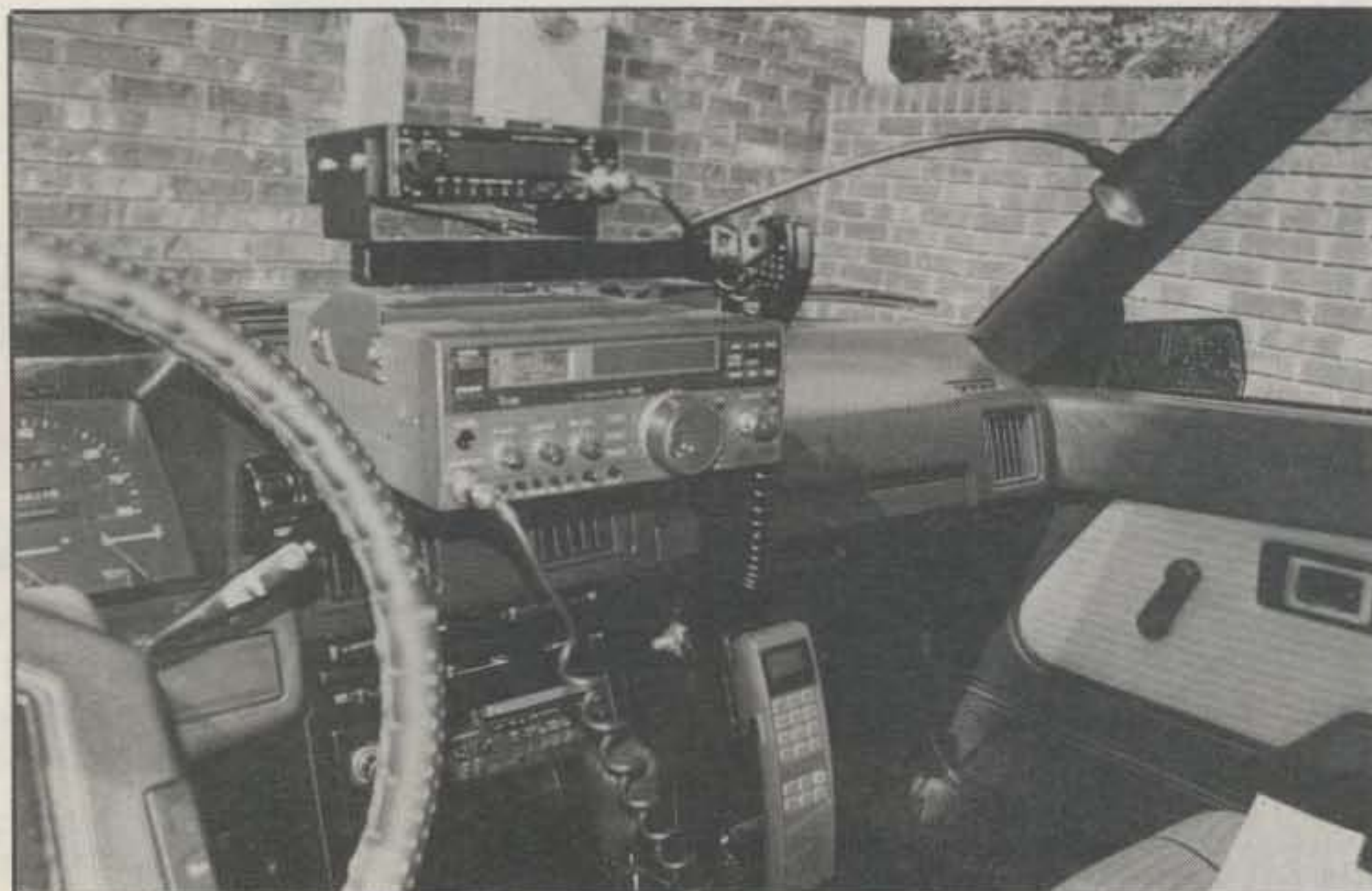
Photo 6- Cockpit view of Outbacker WD4FSY's setup. Rigs are held in position by custom IIX bracket, as discussed in text.
