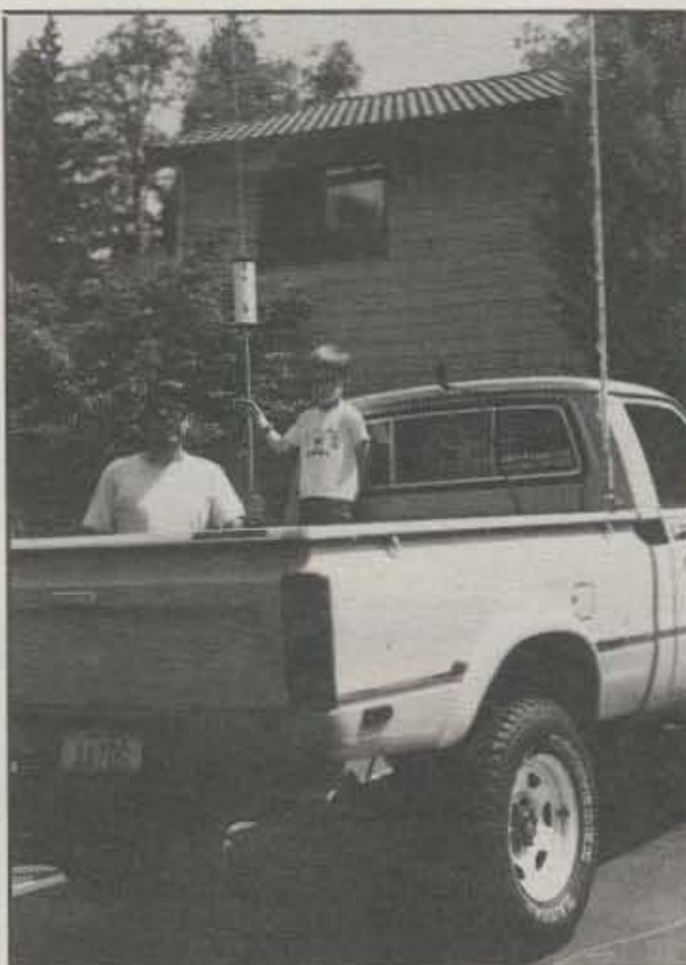
Photo 3- Lindell, AA7DG, and son Maxwell, with all-band mobile. Supertenna on left is flanked by Outbacker on right, 2m/70cm antenna on cab, and 1.2 GHz "spike" barely visible on cab's front.
