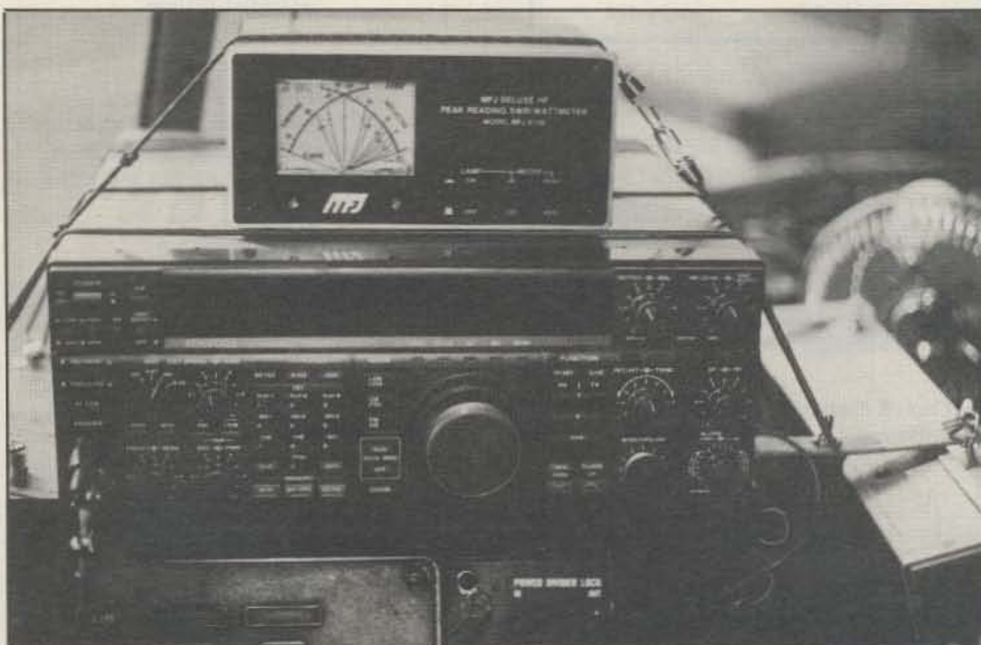
Photo 2—In-cab view of the 18-wheel KA0ZFX mobile setup. Kenwood 850 drives kilowatt amplifier barely visible on right. Note fan on dash for cooling.
