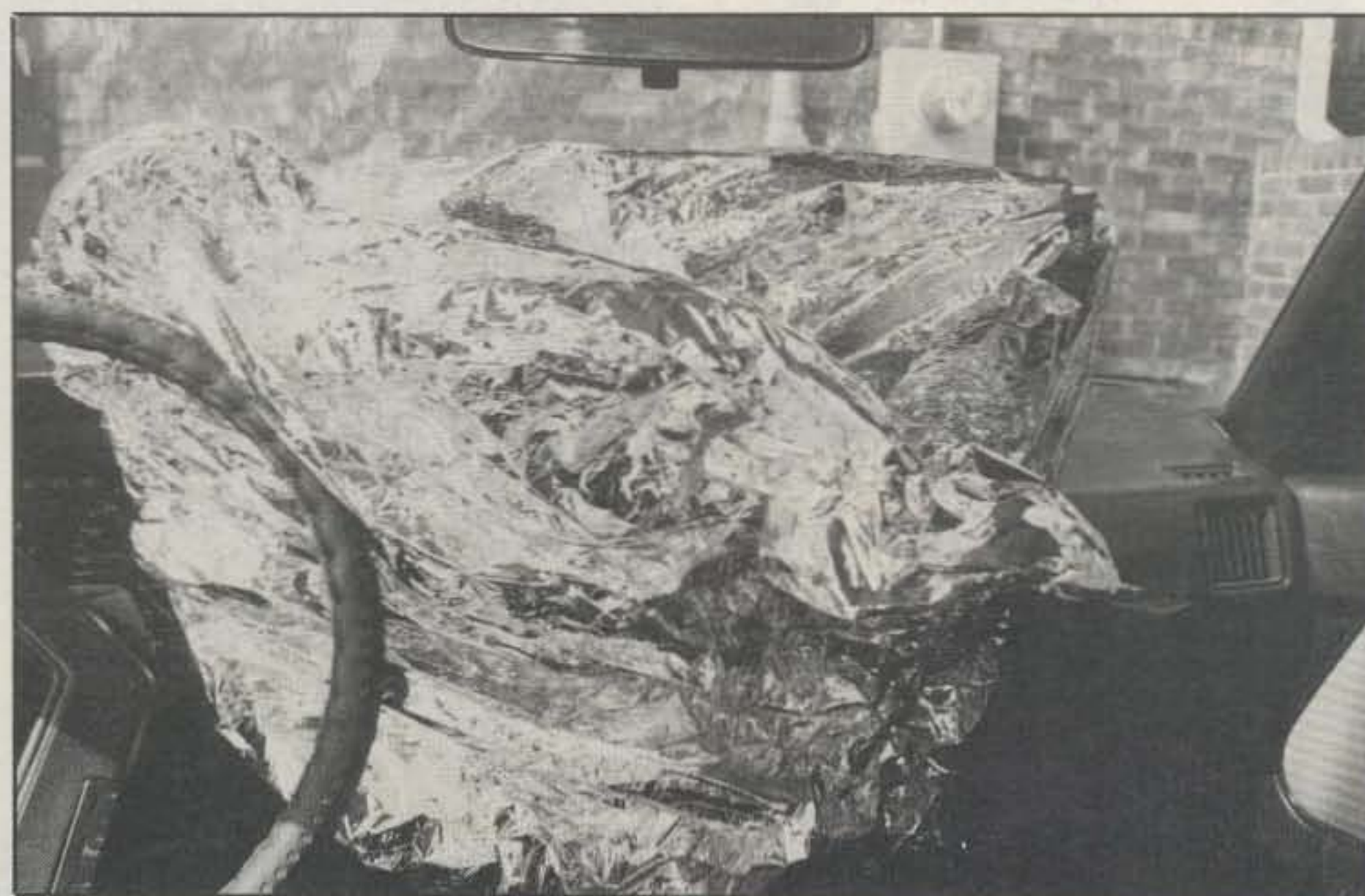
Photo 8- Ghostbusters mobile? No, it's an inexpensive emergency blanket used as a rig cover. (Details in text.)
