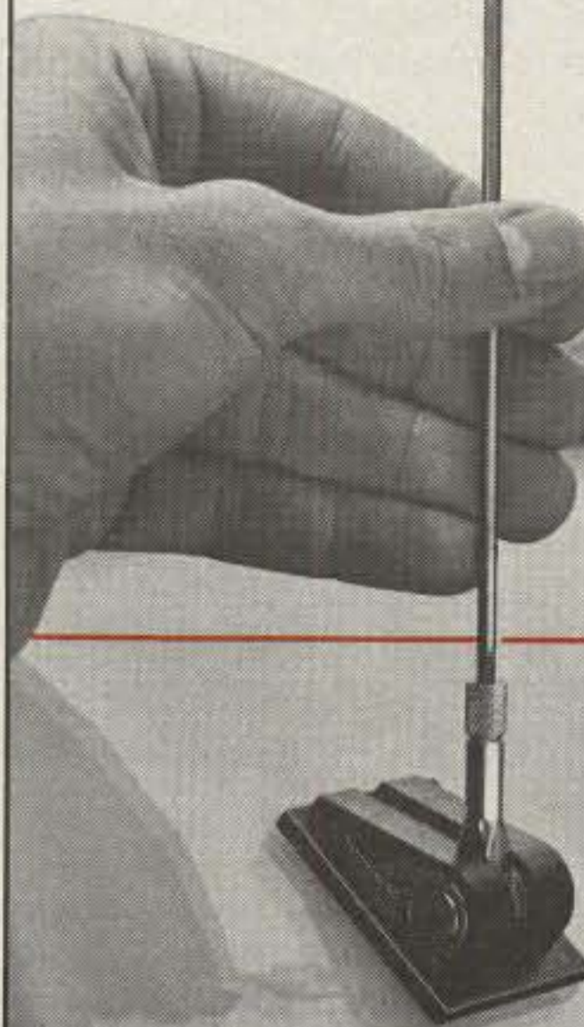
The Electron Processing MSW-1 Mobile Antenna Adapter is an amplifying receiving antenna coupler designed for mobile use. Its purpose is to allow the use of an existing car radio antenna with a separate shortwave or scanner receiver. The MSW-1 covers the range 0.5 to 1000 MHz and includes an internal 10 dB gain amplifier. (Photo courtesy Electron Processing, Inc.)
