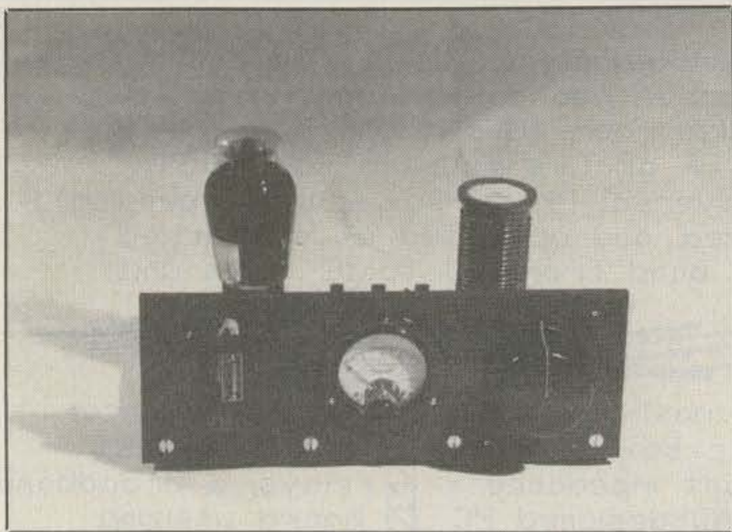
Fig. 4— Front view of KY8I's 1940s-style 6L6 transmitter. Visualize using this delight with a National SW-3 receiver today.
