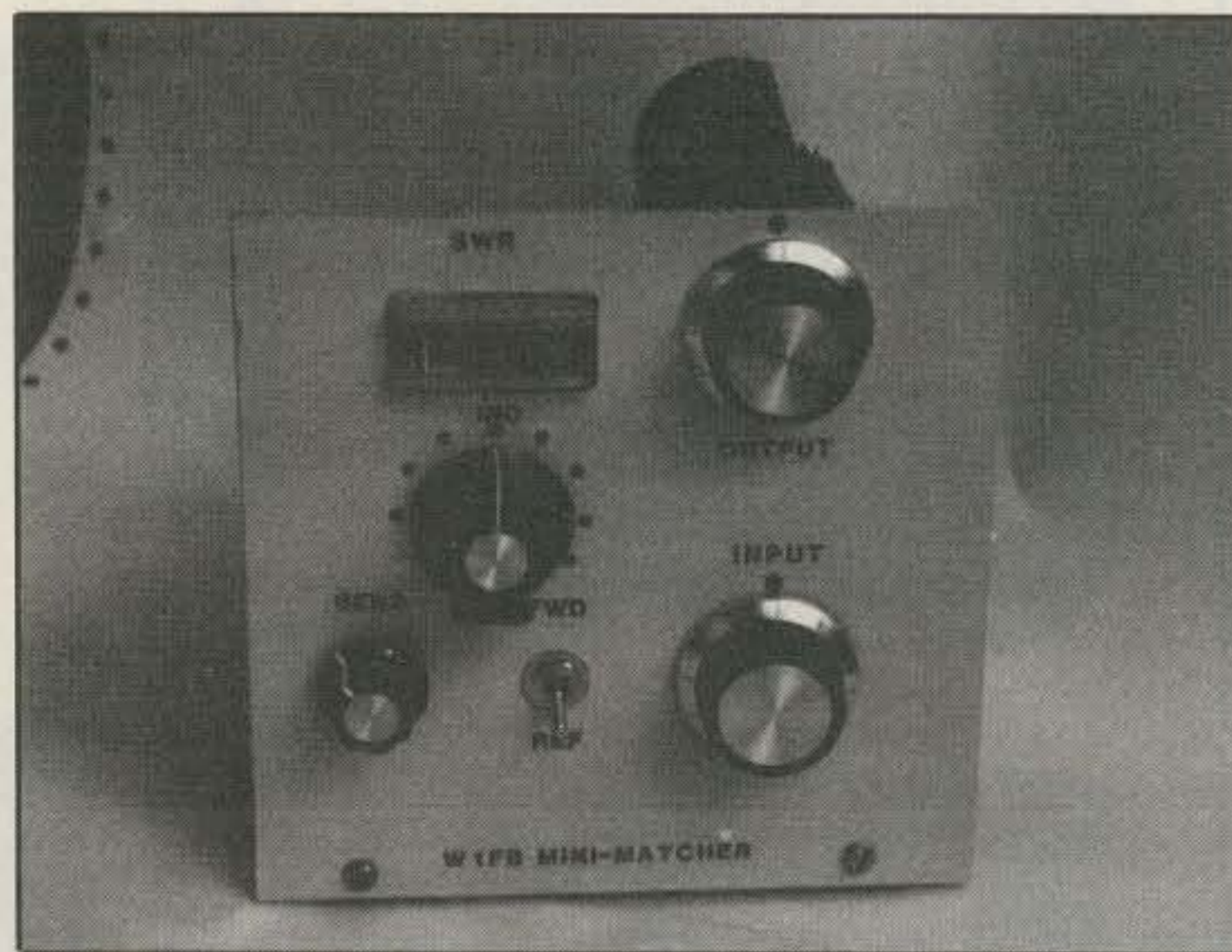
The front view shows a well-balanced layout of controls. The size (5 ¼" × 5" × 4 ¼") gives rise to its name of mini-matcher.
