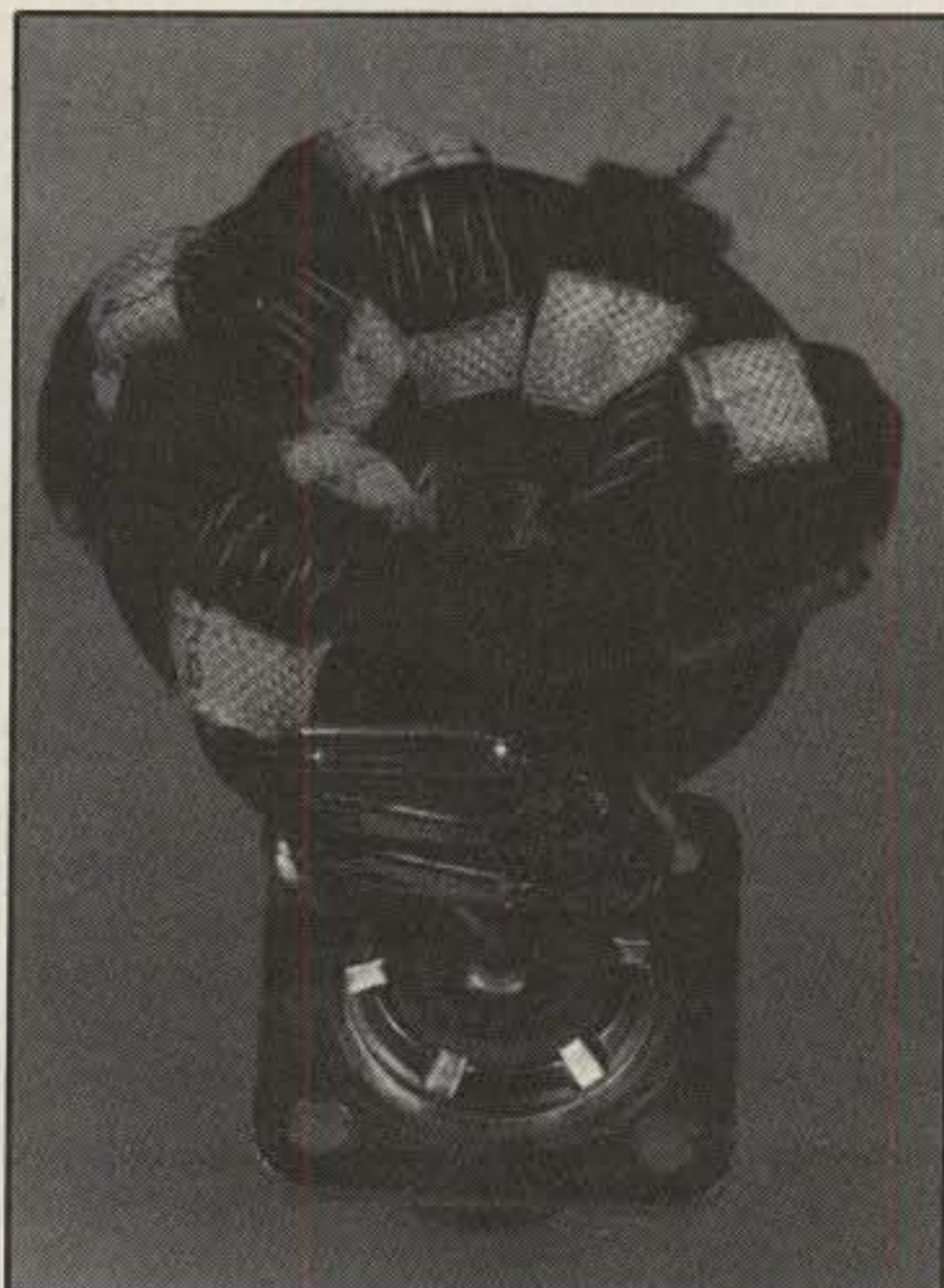
Fig. 4- Photograph of the 1.33:1 unun (66.7:50 ohms). This transformer also has a broadband 1.56:1 ratio (50:32 ohms).
