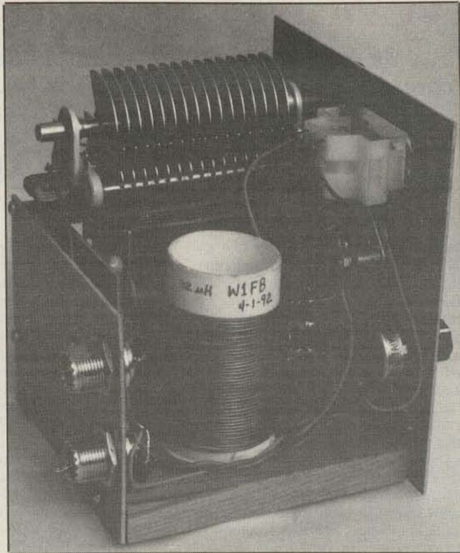
View of the left side of the tuner. L1 and its taps are visible in the foreground.
