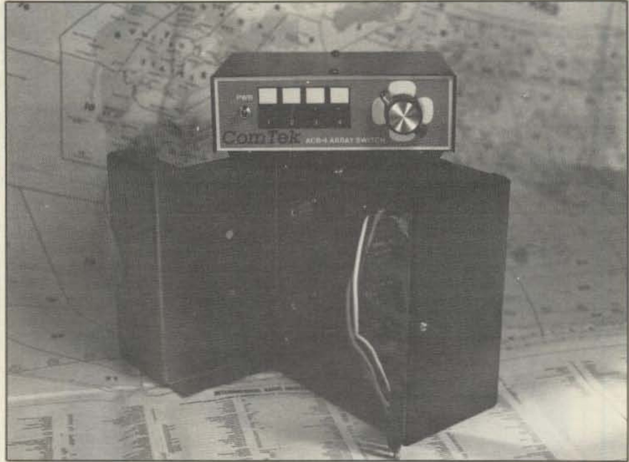
The heart of the ComTek phased array vertical systems is the outdoor switchbox and the in-shack selector/control box, shown in this photo. For more details, see the text of this month's column. (Photo courtesy ComTek)
