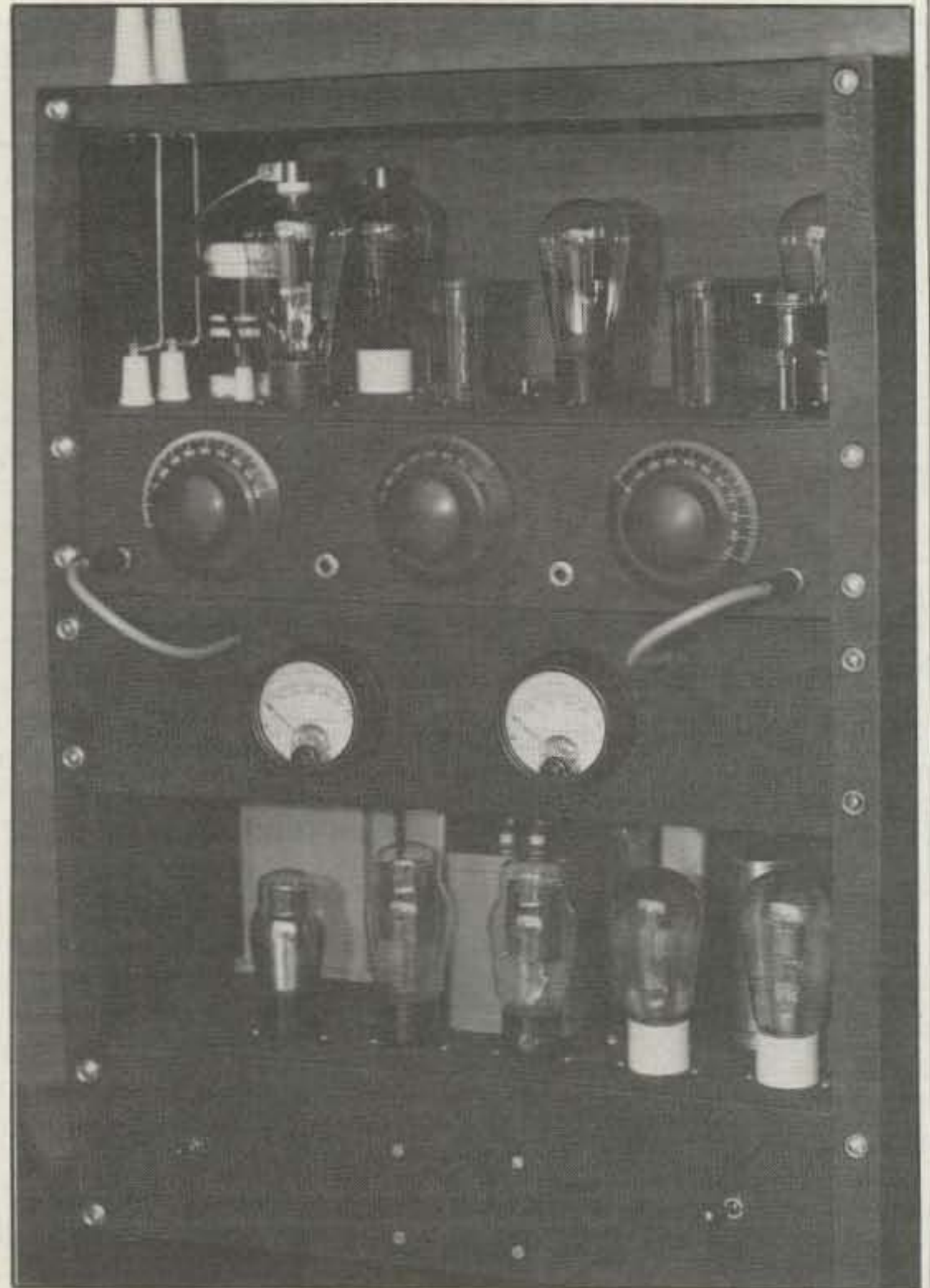
Fig. 8—Refurbished CB-25 transmitter of John Rollins, W1FPZ. The line-up is 47 crystal oscillator, 46 buffer, and two 46's in the final amplifier.
