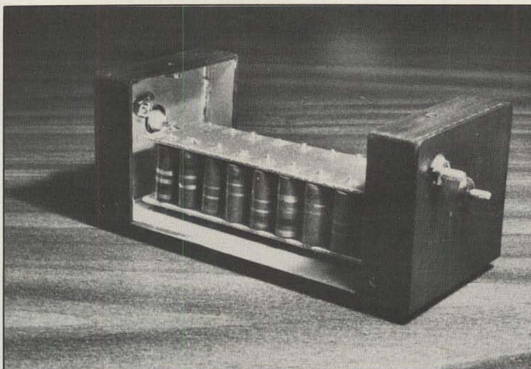
An inside view of the dummy load. Note the very short leads on the resistors and the BNC jack. Test points for attaching an oscilloscope probe are on the rear of the unit.
