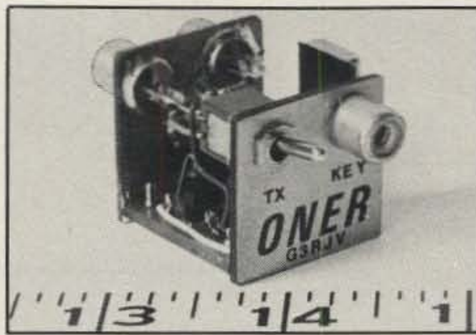
Fig. 4- The famous little "Oner" transmitter built by G3RJV. Complete rig is 1 inch square and produces 1 watt output.
