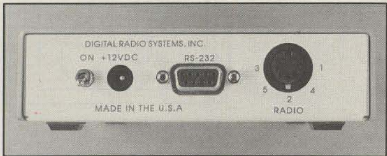
(Top) Front view of the DRSI DPK-2 TNC, which isn't a drain on the pocketbook or the power supply. (Bottom) Rear view of the DPK-2 showing the on/off switch and power supply, RS-232, and transceiver connections.
