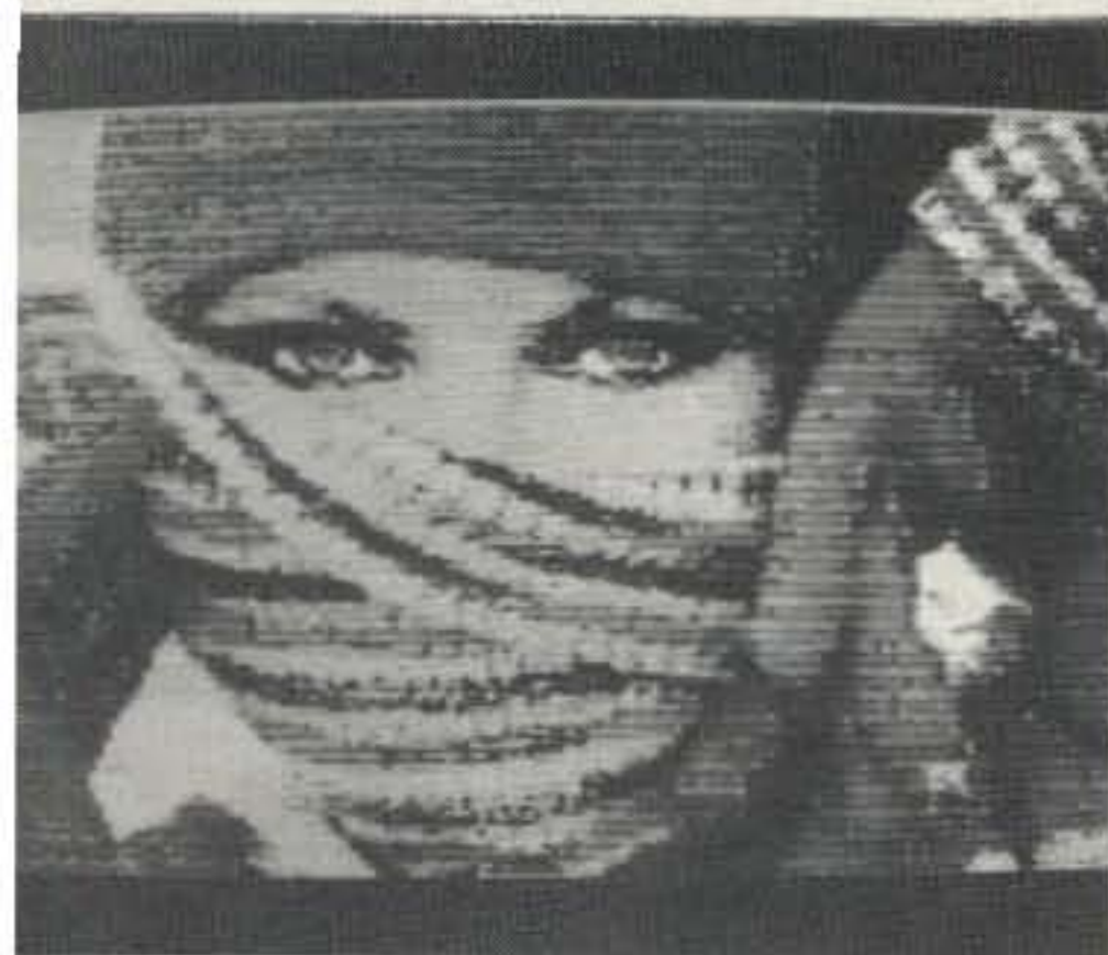
Full Color SSTV picture actually received on 4.230 MHz, using Robot 72 second format. Transmit and receive color and black and white SSTV pictures.
