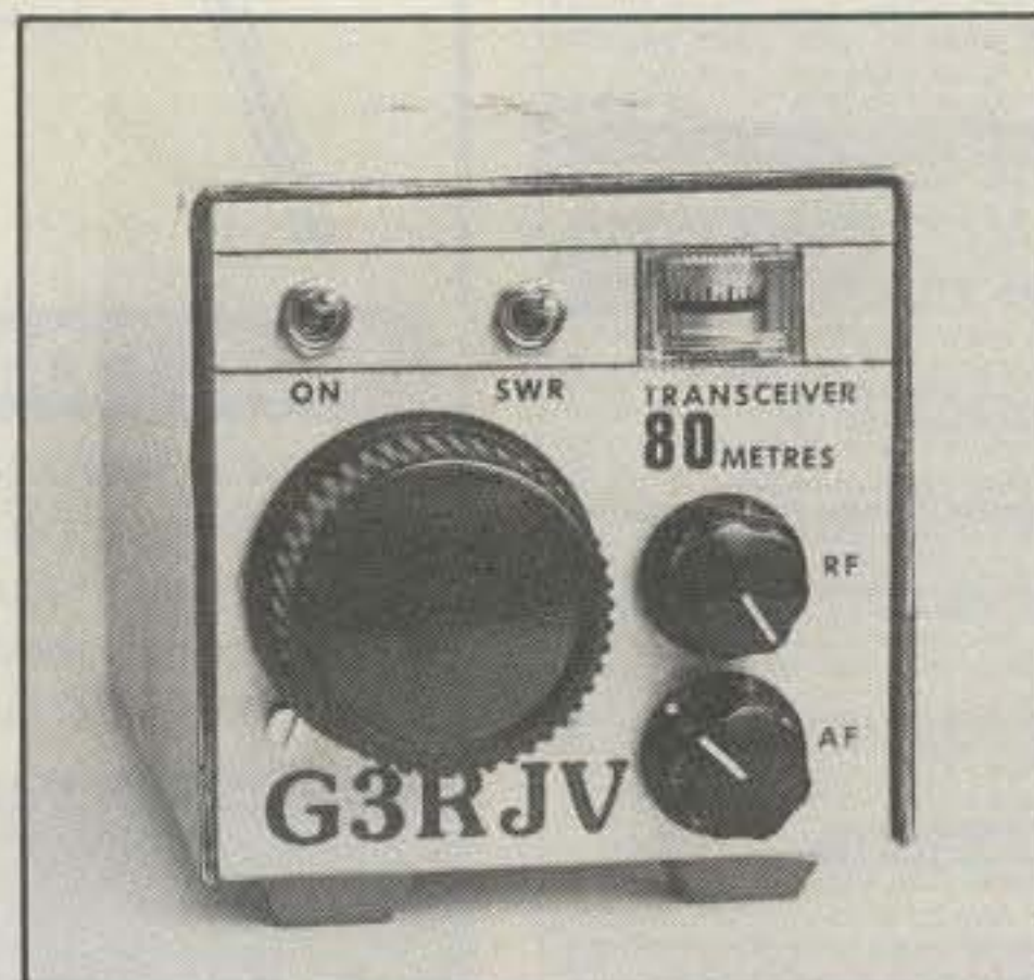
Fig. 9- A recent product of G3RJV's workshop: a compact 80 meter transceiver that works great.
