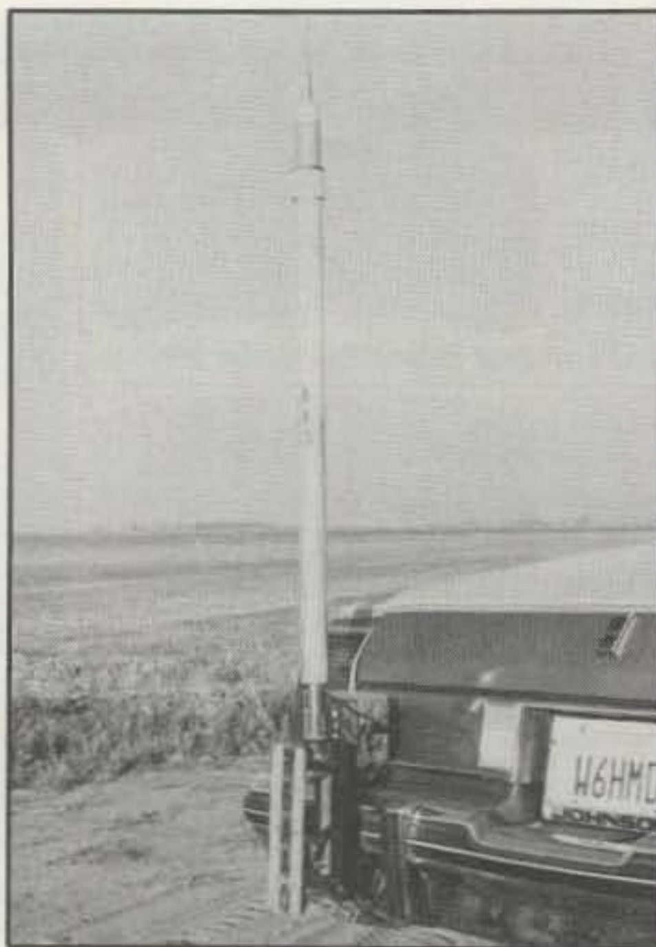
Photo 7— DK3 antenna mounted on rear of W6HMD (XYL of W6AAQ) car. Notice coil near photo top: It moves up and down in base unit to change bands automatically.
