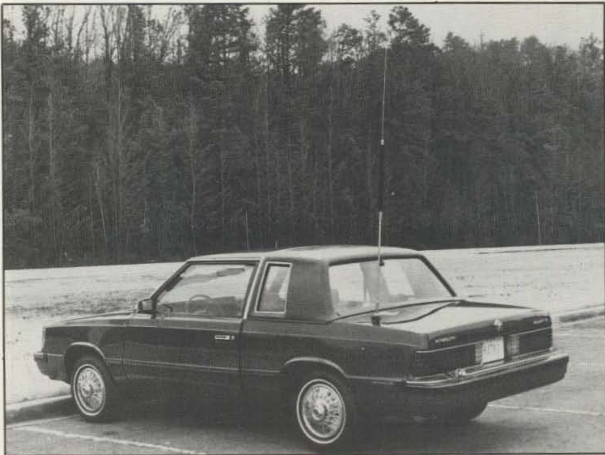
Photo 5- One-sixty meter mobile in style! Antenna is PRO•AM's PHF-160, and it works great. (Details in text.)
