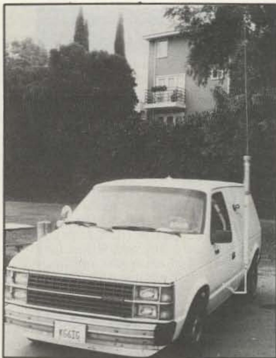
Photo 6— Now this is the way to go HF mobile! KG6IG's van is fitted with big W6AAQ DK3 all-band and fully automatic antenna system. Check out that heavy-duty mount! Top whip, incidentally, is almost full-size CB antenna!
