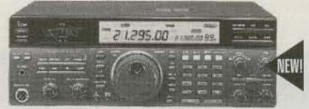
12V 100W w/auto Ant. Tuner Built-in Gen Cov. RX, 101 Mem. DDS, QSK, Passband tuning **Call For Special Price**
