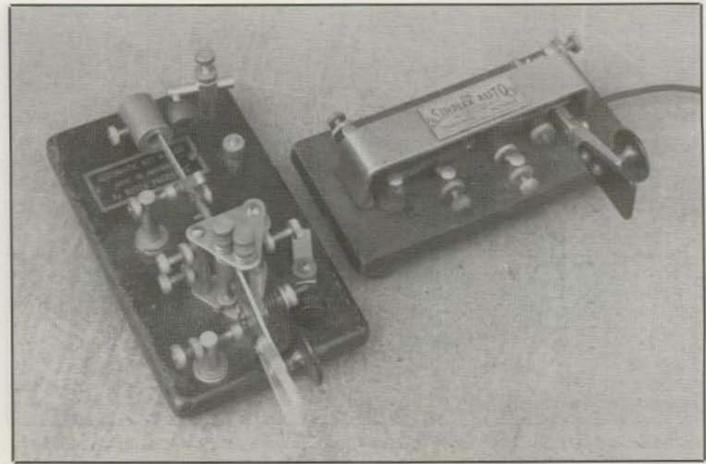
Photo 6- Australian-made Buzza and Simplex Auto bugs used daily by VK3XU. Right-angle bug is a real heart-throb. Drew works 30 meters, and his "CW fist" is outstanding.
