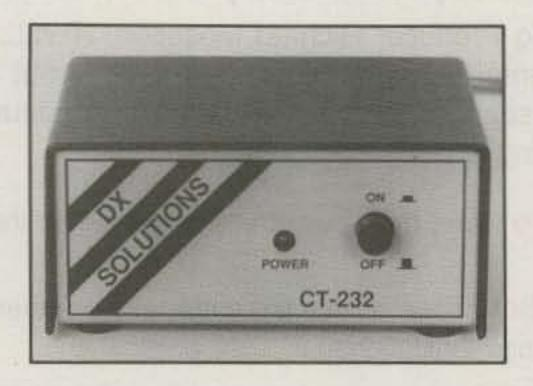
A companion to the SAS-6 is the CT-232 interface, a hardware interface to allow most transceivers to be computer controlled via a serial data link. It can be used together with most rig control software, in addition to the SAS-6 switch. The CT-232 interface is connected in series with the SAS-6; there's no need for an extra COM port on your PC. (Photo courtesy DX Solutions)
