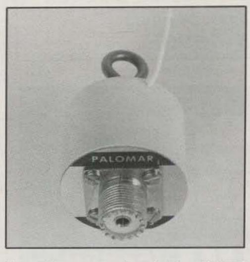
A special-purpose receive-only balun of interest to the SWL is the Palomar Engineers MLB-1 Magnetic Longwire Balun™, which connects at the end of a longwire antenna and allows coaxial cable to be used from this point to the radio. The MLB-1 has a SO-239 type connector to accept coax and a single-wire lead to connect to the antenna flattop. (Photo courtesy Palomar Engineers)
