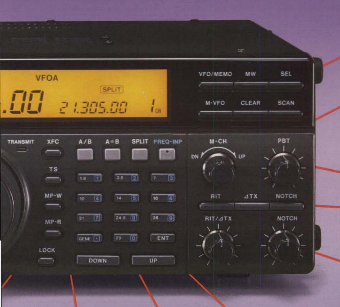
Hold SPLIT down for one second to start the split mode function and initiate QUICK SPLIT feature, equalizing both VFOs to the same frequency.
