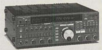
YAESU FT-736R • All-mode, 2M/430 multi-band VHF/UHF. Optional. modules for 50MHz, 220MHz, and 1.2GHz. 10W on 50MHz and 1.2GHz, 25W.on 2m and 440 MHz. Built-in AC ps, or 12V DC w/optional power cord. 5½"h x 14½"w x 11½"d, 19.8 lbs... LIST \$1999.00
