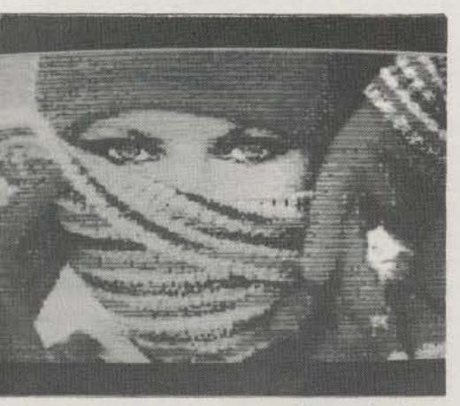
Full Color SSTV picture actually received on 14.230 MHz, using Robot 72 second format. Transmit and receive color and black and white SSTV pictures.
