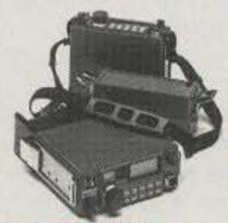
MK II's 2½w, FM, SSB/CW portable. Requires 12V DC @ 1.1A, or opt. battery case with 9 (C) cells or nicads. DTMF mic with up-down control, dual VFOs, 10 memories with scan. Offset tuning, LCD display. 2½"h 6½"w x 7½"d, 2.6 lbs.
