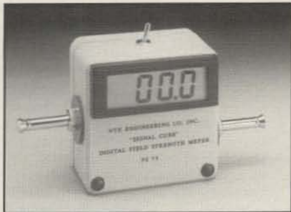
The Nye Engineering FS 73 Signal Cube is an untuned, broadband device that covers 0.1 to 450 MHz and can be used for absolute readings with its built-in dipole antenna. It's equipped with a 3.5 digit LCD display that indicates RF amplitude. (Photo courtesy Nye Engineering Co., Inc.)
