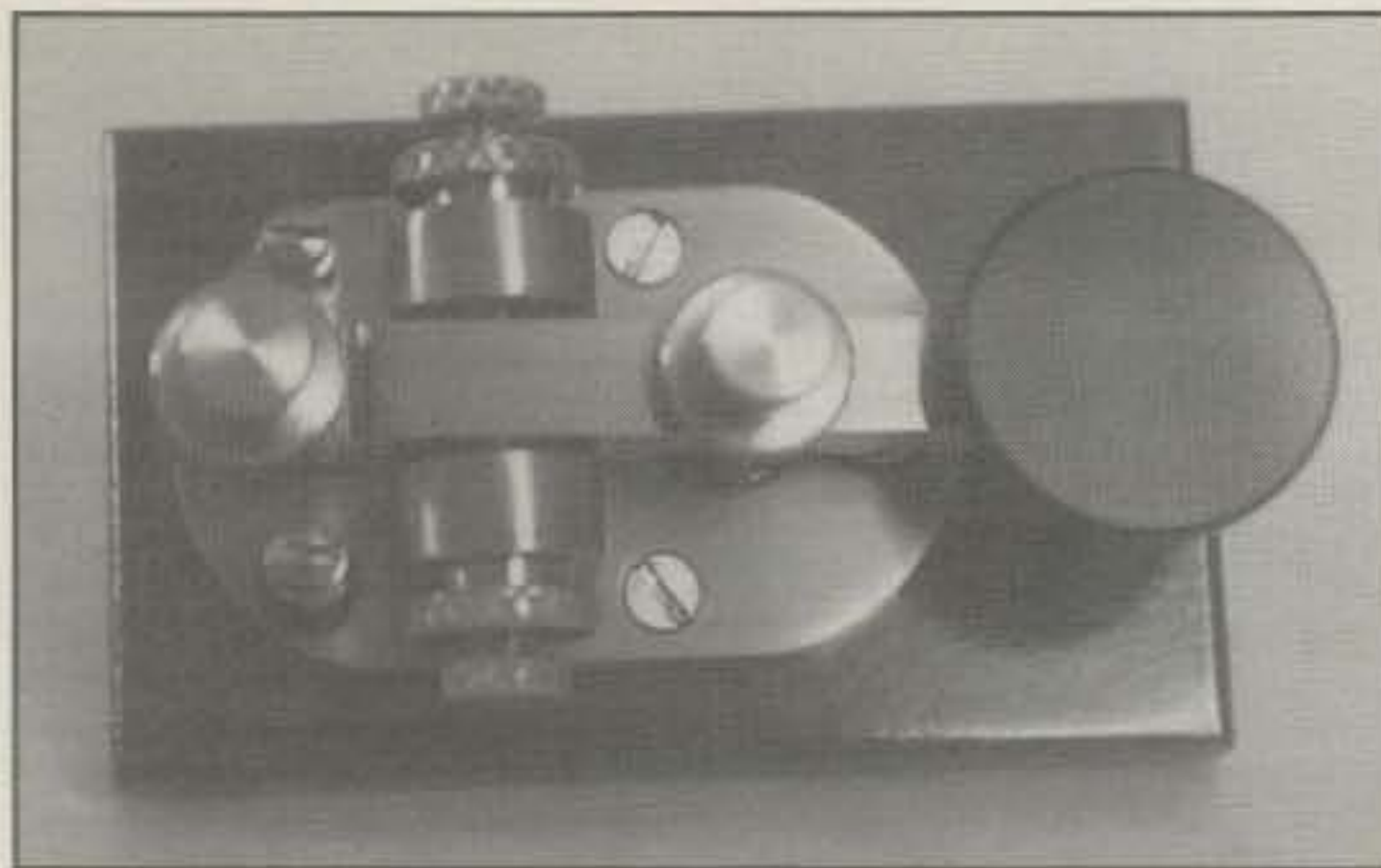
Photo 5— Top view of W8WVM's key shows narrow gap between arm and pivot points. Unique design reminds me of classic Chubbok key in its closely spaced fulcrum.
