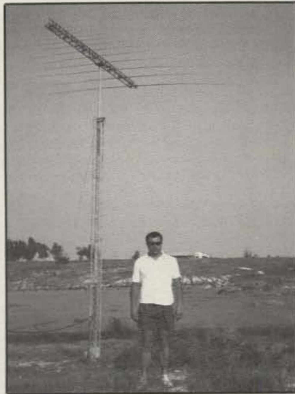
The voice of P31A, Ivo, 5B4ADA, stands in front of his 14-element log periodic.
