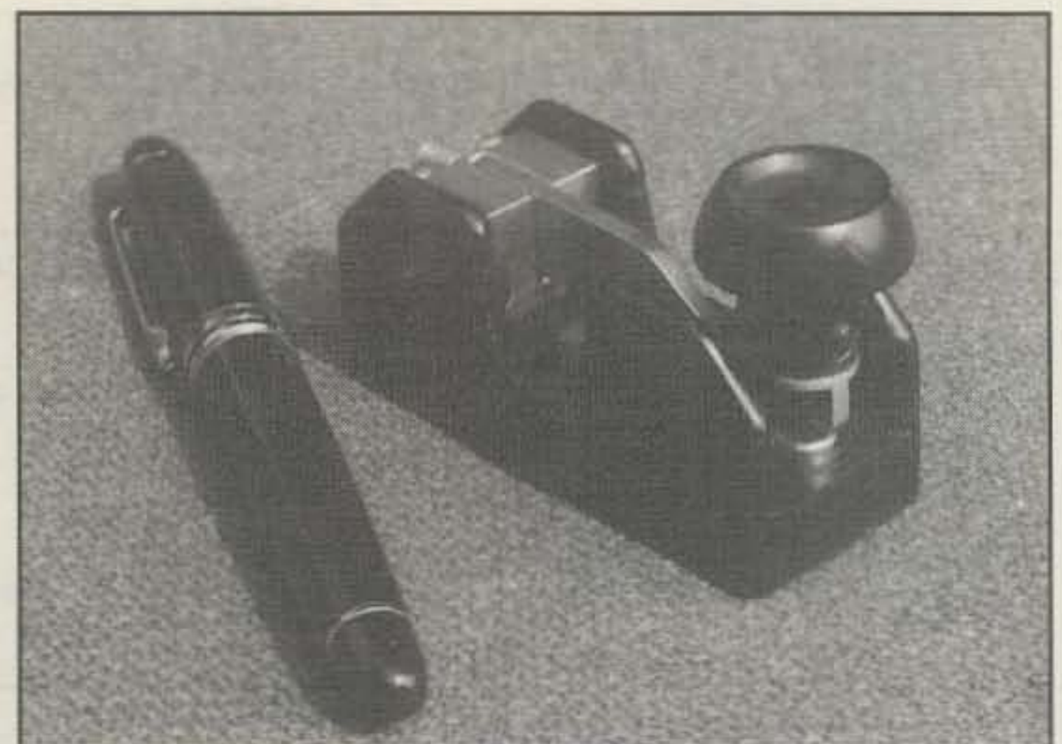
Photo 10— This N1KPR home-assembled key was made with parts of a fuse holder. Incredible what can be accomplished with a little imagination.
