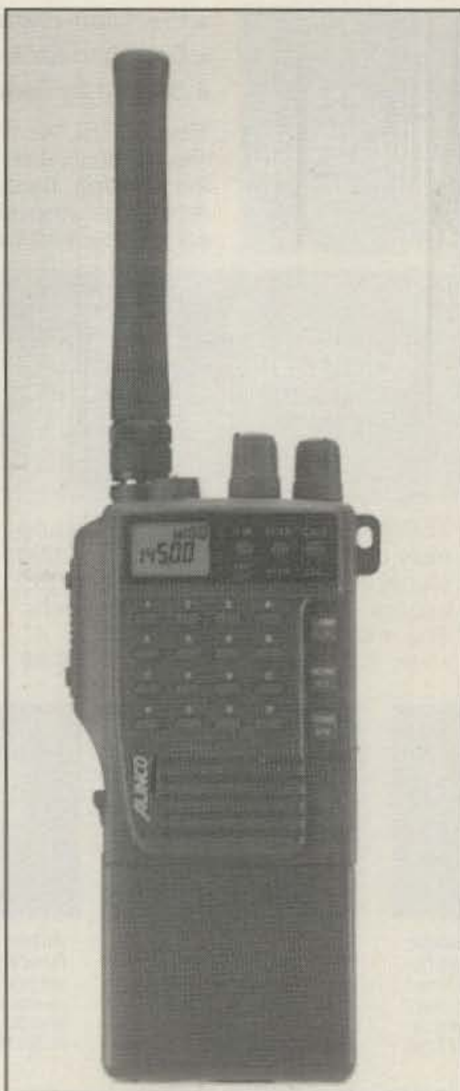
The Alinco DJ-180 is a 2 meter FM handheld that has all of today's most popular features.
