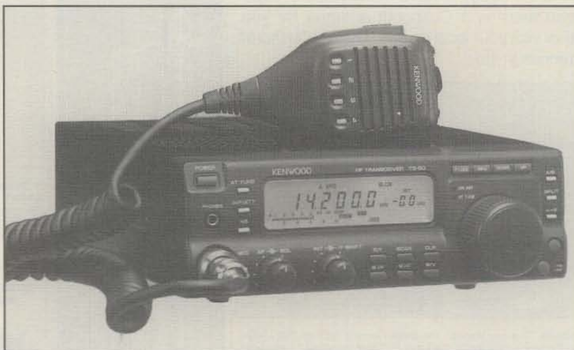
A view of the front of the Kenwood TS-50S. As explained in the text, the mic serves as a "tuning" control along with other front-panel control items.
