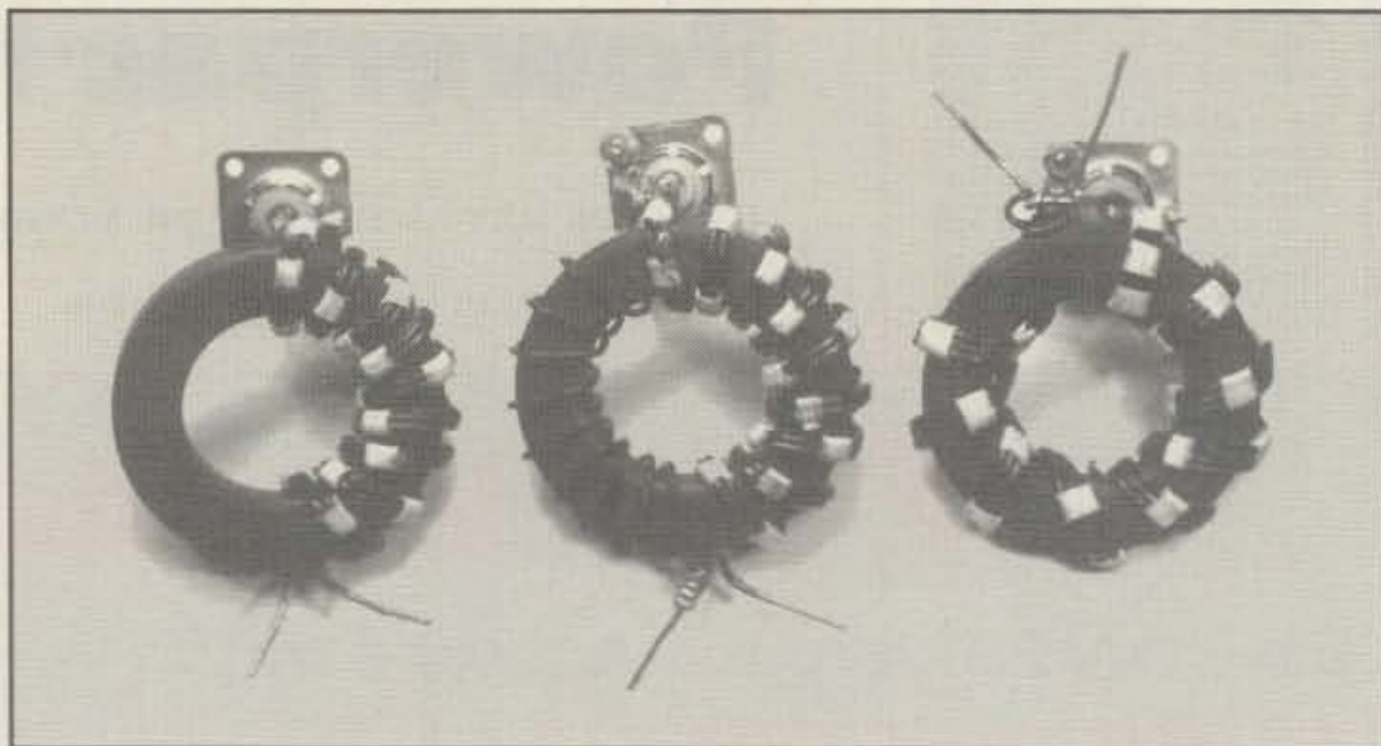
Photo A—The three basic forms of the 1:1 balun: left, the Guanella (current/choke) balun; center, the Ruthroff balun; and right, the trifilar (voltage) balun.
