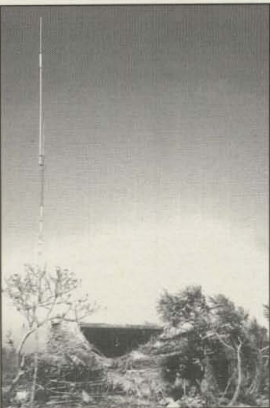
Most IOTA DXpeditions make do with the simplest equipment, such as this trap vertical antenna of I2YDX/DU6 pictured here on Caluya island (OC-125) in 1991. (VE3XN photo)
