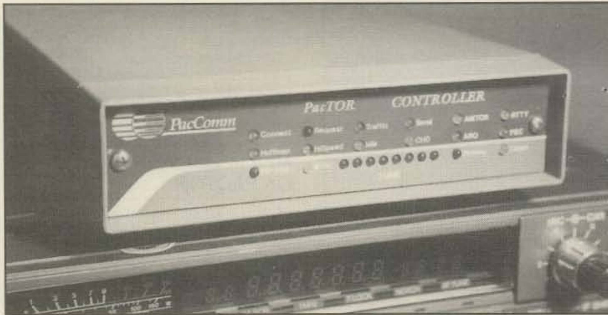
One of the first controllers to introduce PACTOR to the American amateur, the PACTOR Controller from PacComm also includes support for AMTOR and RTTY. (Photo courtesy PacComm Packet Radio Systems, Inc.)
