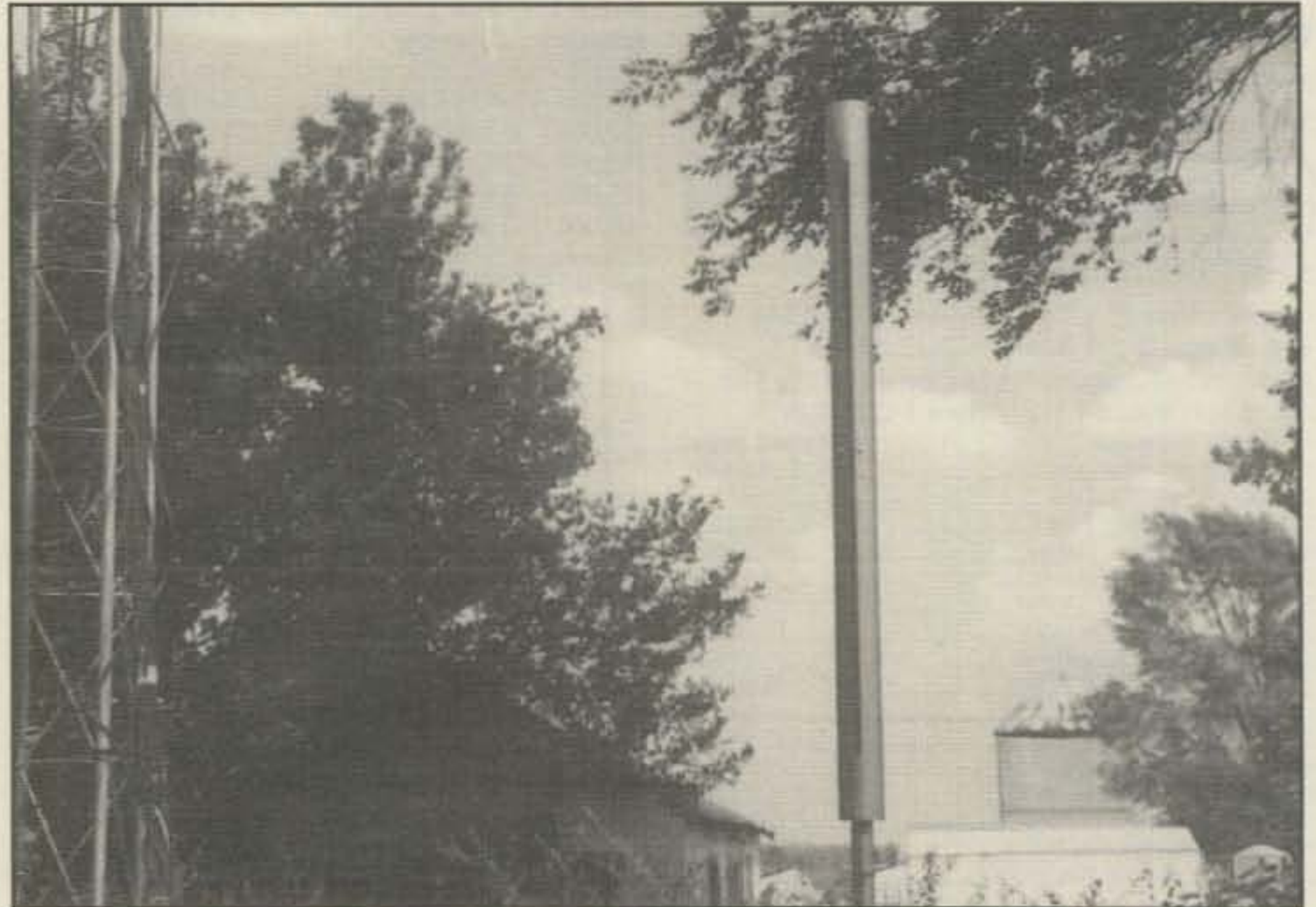
The Model AS70 modified Alford Slot ATV Repeater Antenna offered by WB0QCD is based on a 1939 Andrew Alford design and later work by Merle Reynolds in the 1980s. The slot design is well suited for use by low-power TV broadcast stations as well as ATV repeaters and remote transmitters, 70 cm packet radio links, and individual UHF stations. The basic antenna is a two-wavelength, 5.6 dBd gain horizontally polarized omnidirectional radiator. A dual-slot, 8.0 dBd gain array also is available. (WB0QCD photo)
