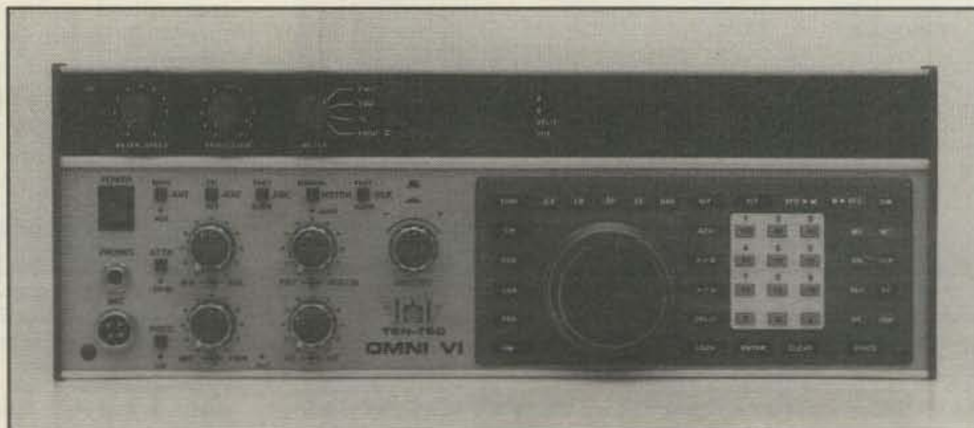
This is the front view of the Omni VI showing all the controls and layout. All switches and controls are very easy to handle. While not visible in this photo, the LED frequency readout consists of LEDs that are .56 inch high, a very large and easy-to-read display.
