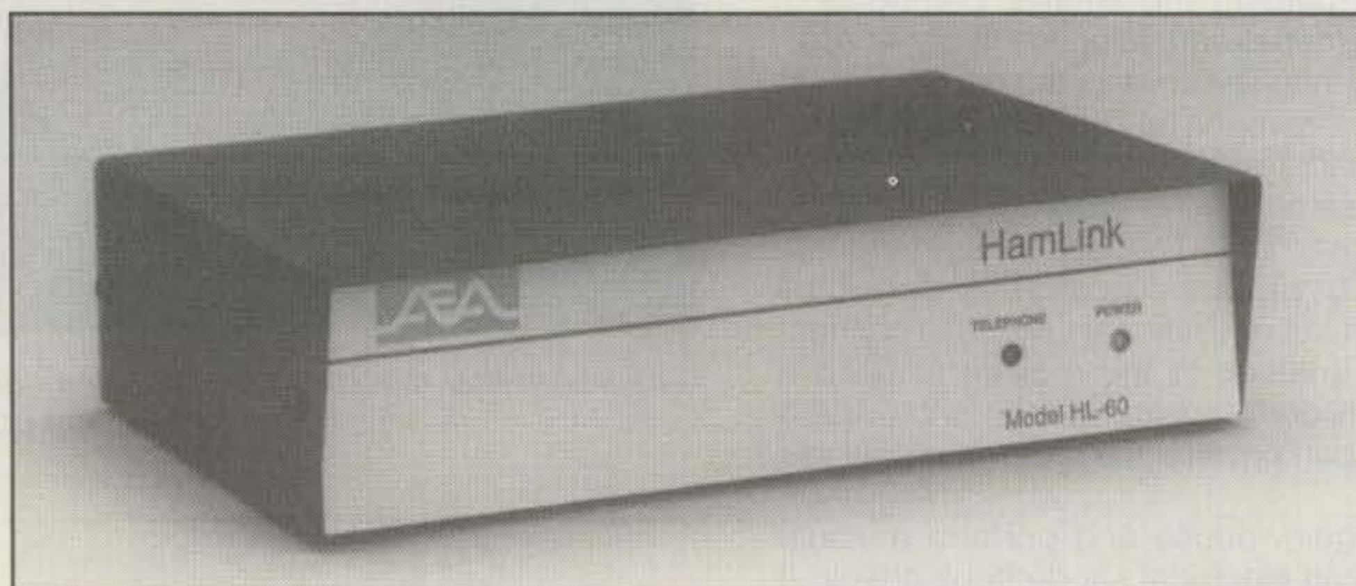
The HamLink, manufactured by AEA, allows you to control your radio from any DTMF-equipped phone, anywhere.
