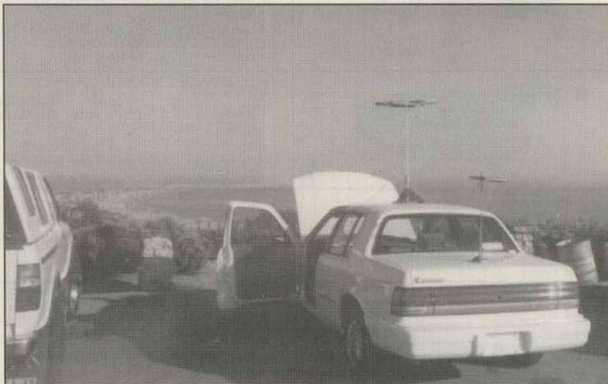
Once again I use my rental car for an antenna farm. The hood is raised so that I have access to the battery for power to the FT 650. On top of the car is the 6 meter SQLLOOP. On the trunk of the car is the 2 meter SQLLOOP. In the background is the southern California coastline.
