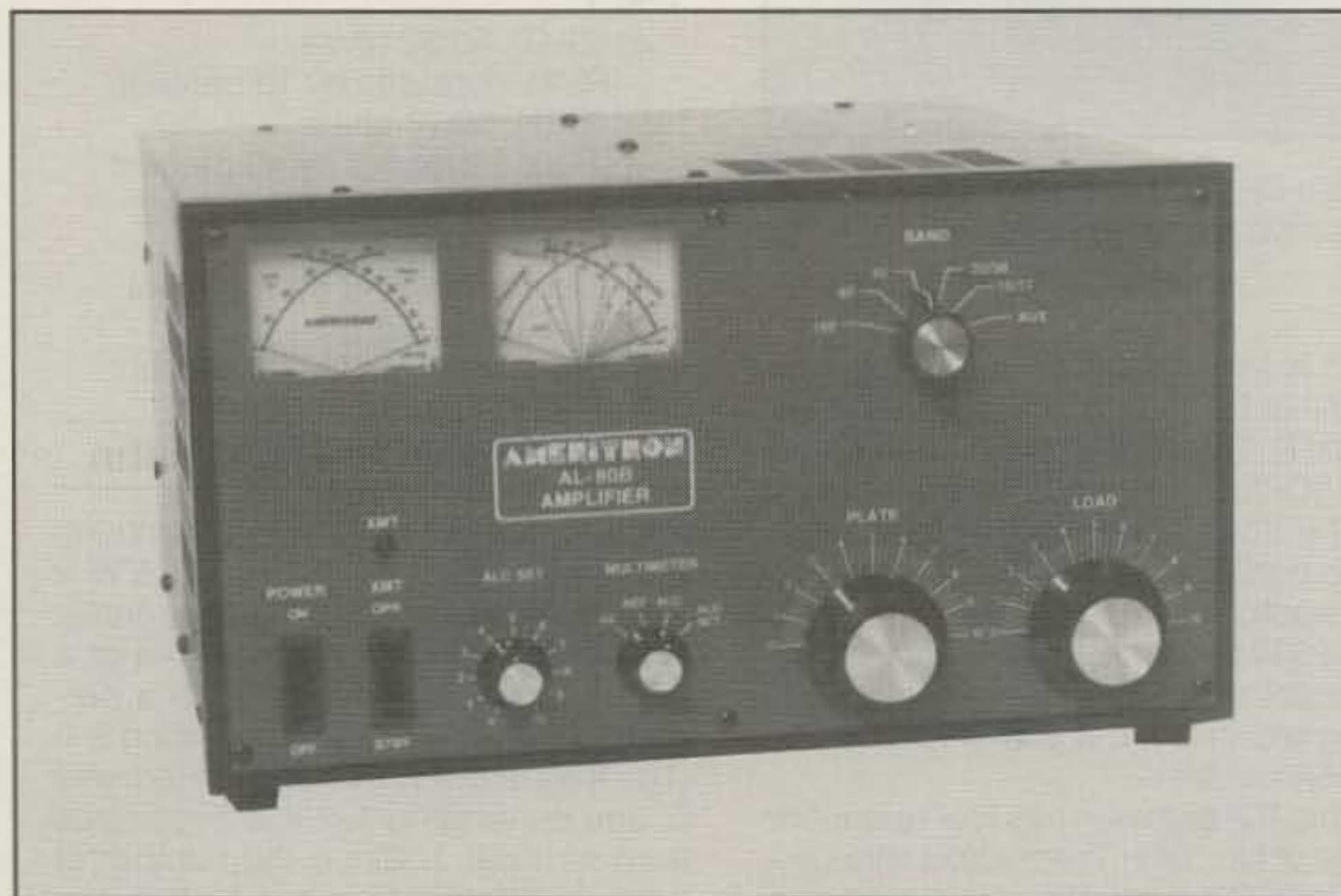
This is the AL-80B. Note the large meter at the upper left. The bandswitch is at the upper right, and the plate and loading controls are at the lower right.
