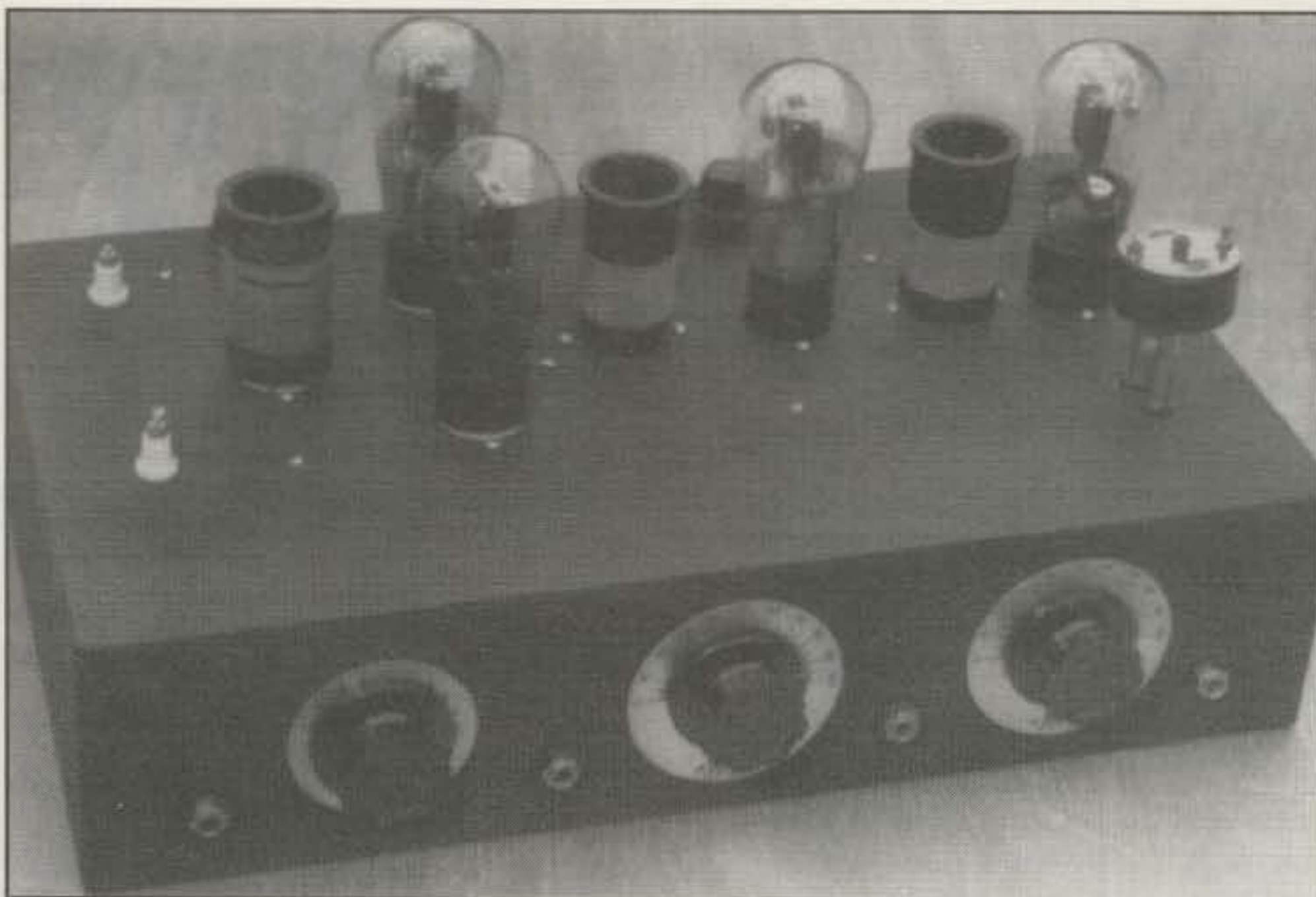
Photo C- Gross CB-25 RF deck. Operation is possible on 160, 80, 40, and 20 meter bands with 40 watts input. Jacks provide meter monitoring points.
