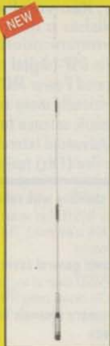
NEW SB-7/SB-7NMO Dual-Band 146/446MHz Gain & Wave: 146MHz 4.5dB 6/8 wave center load 446MHz 7.2dB 5/8 wave x 3 VSWR: 1.5:1 or less Max Power: 70W FM Length: 4' 7" Connector: PL-259 or NMO style
