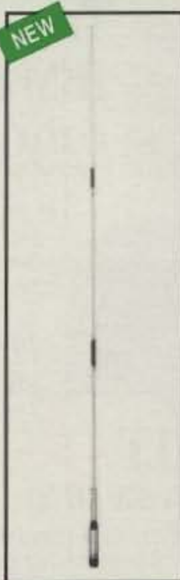
SB-7/SB-7NMO Dual-Band 146/446MHz Gain & Wave: 146MHz 4.5dBi 6/8 wave center load 446MHz 7.2dBi 5/8 wave x 3 VSWR: 1.5:1 or less Max Power: 70W FM Length: 47" Connector: PL-259 or NMO style
