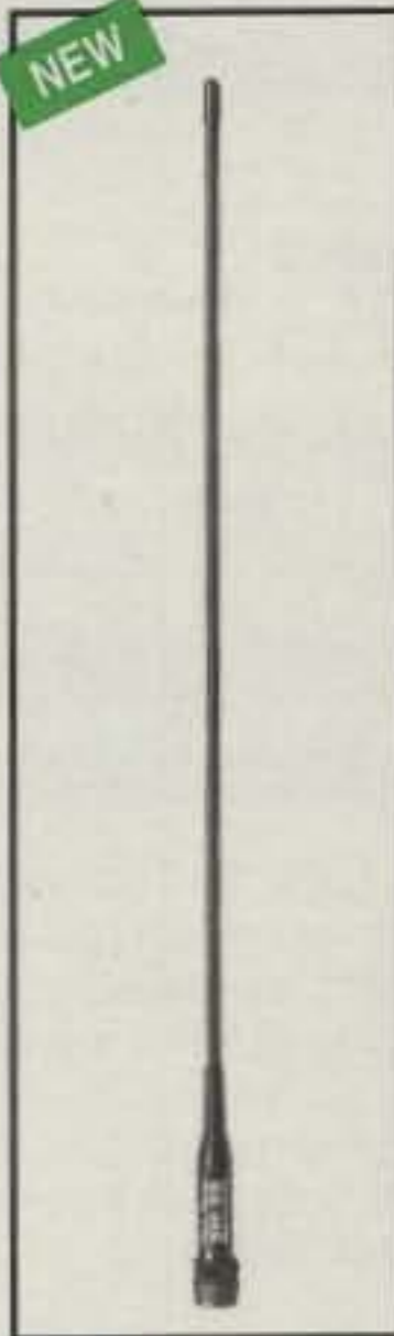
SH-55 146/446MHz HT Antenna Gain & Wave: 146MHz 1.5dBi 1/4 wave 446MHz 3.2dBi 5/8 wave Max Power: 10 watts Length: 15.5" Connector: BNC
