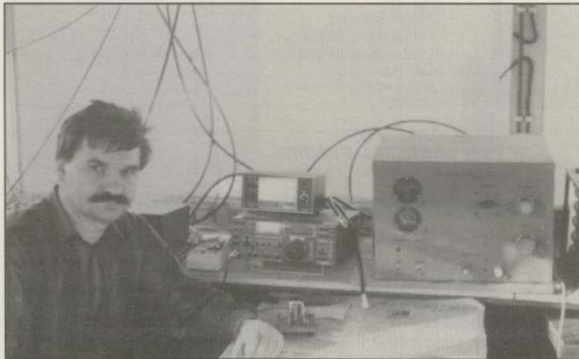
YU7AV sent along this photo of his station complete with homebrew 2000 watt PEP linear!
