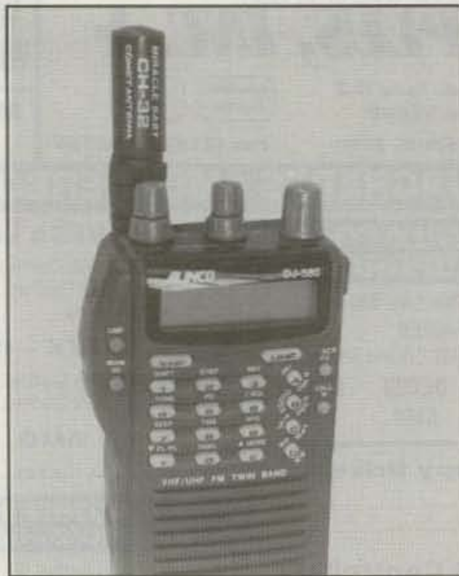
Photo 6- Comet's CH-32 "Miracle Baby" 2 meter/70 cm antenna really makes a handheld compact! This micro-duckie is only 1.3 inches tall and works well for close-range communications.
