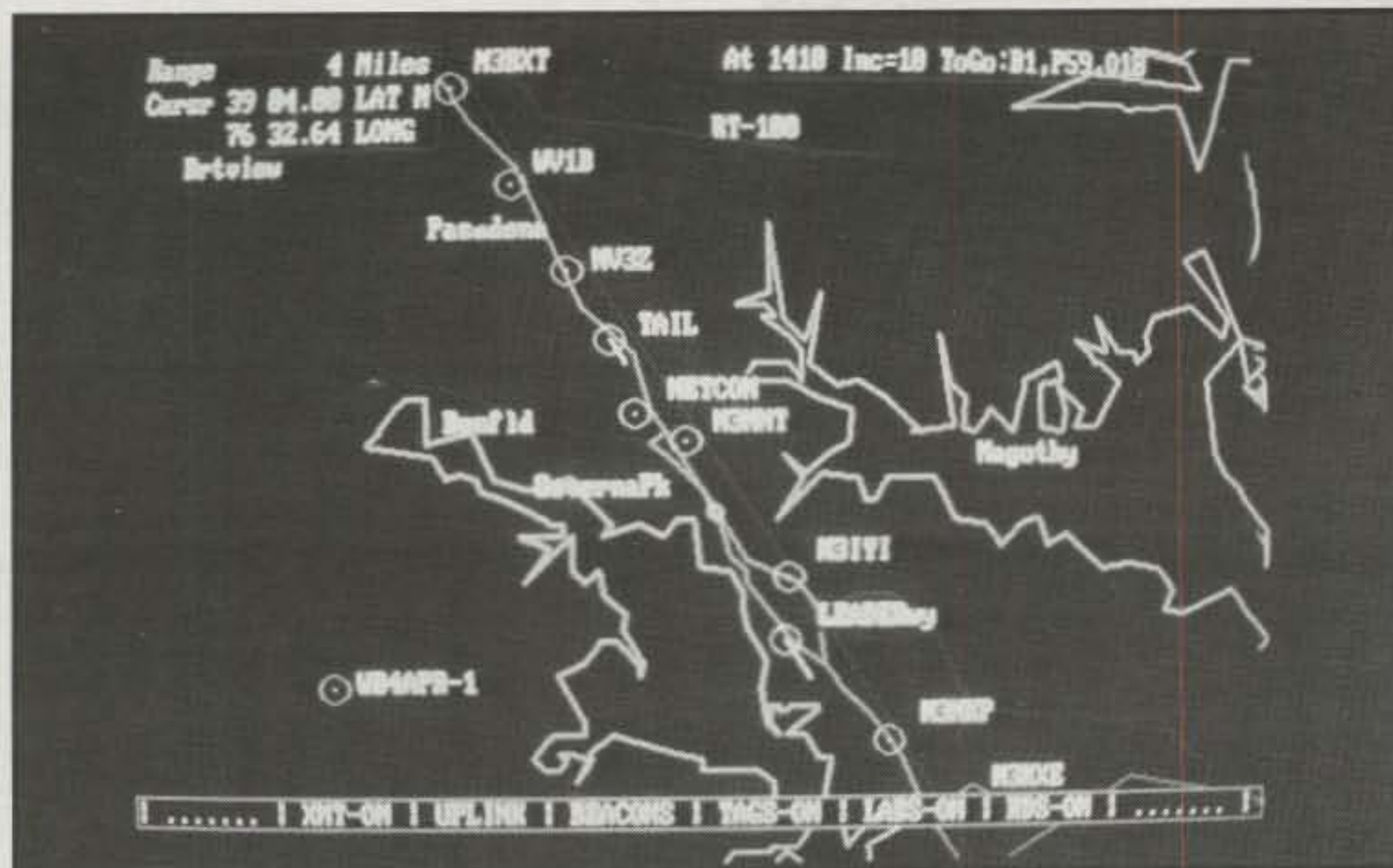
Fig. 3— Here the APRS is being used to track the running of a local marathon. Nine portable packet stations were used along the course for displaying the location of the LEAD, PACK, and TAIL bicycles. Although the bicycles were equipped with GPS interfaced to TNCs, a lot of the tracking was done by manually updating the position of objects along the course.
