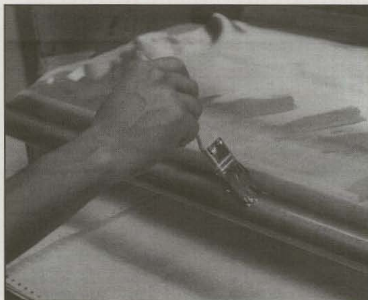
Wrapping the fiberglass cloth over the coil.
