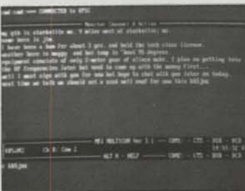
MultiCom™ lets you carry on two digital QSO's simultaneously using two multi-modes or TNC's and two comm ports.
