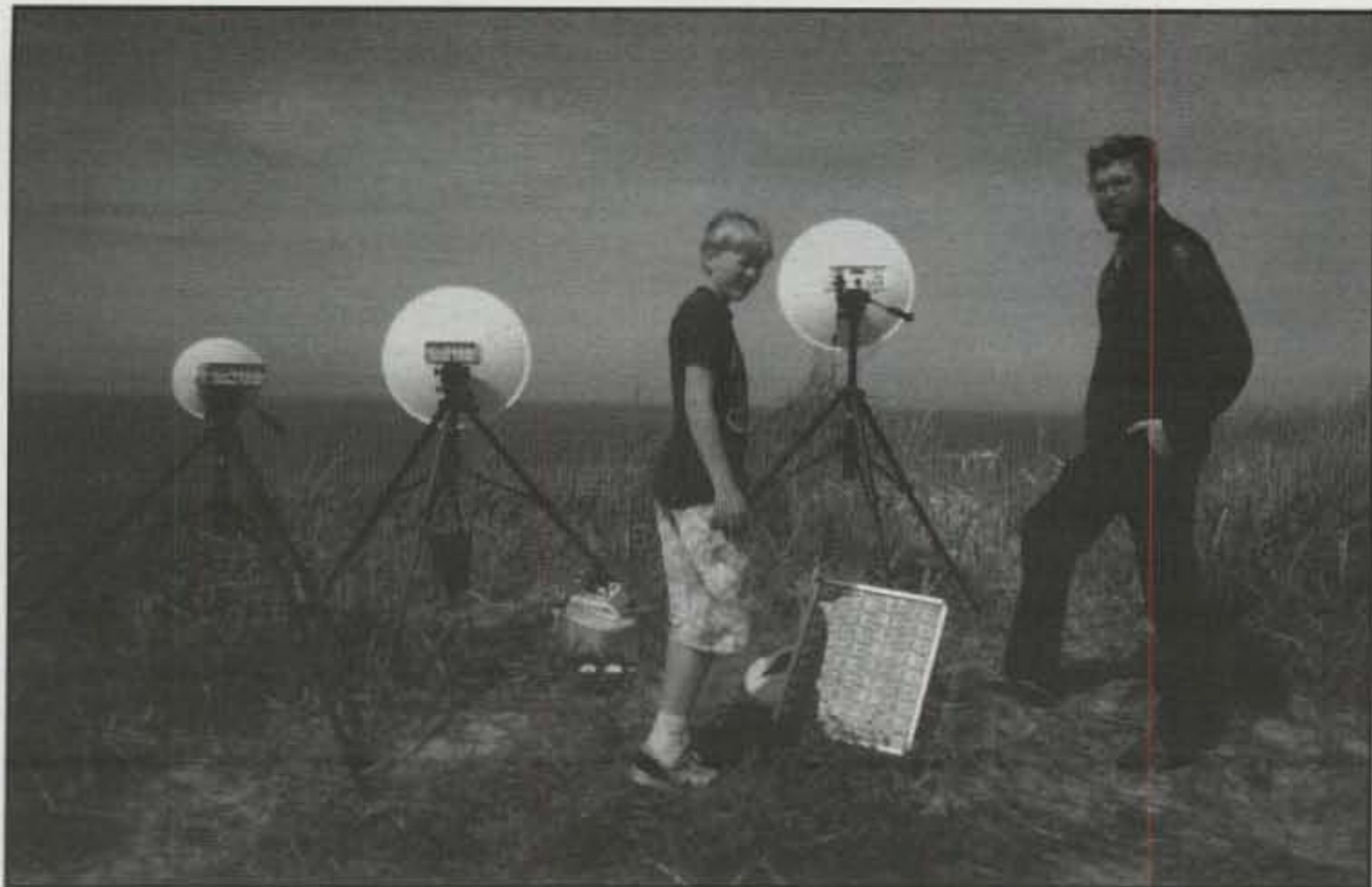
The son of OZ1UM (left) and CE5SPR (right) look over the OZ1UM 10, 24, and 47 GHz stations set up at Spodsbjerg (grid square JO55wx). Note the solar panel: all stations are fully powered by the sun. (Photo via OZ9ZI)
