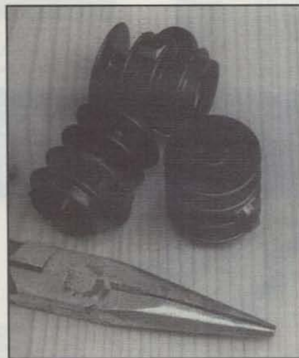
Electric fence insulators are an inexpensive and easy tool for managing balanced feeders. Runs of 450 ohm "windowed" ladder line fit over the top. Three-hundred ohm "windowed" line can be held by the hooks on the side, and a pair of these at the required spacing will keep open-wire line in place. (Photos in this article by Don Randall, WB5ROU)
