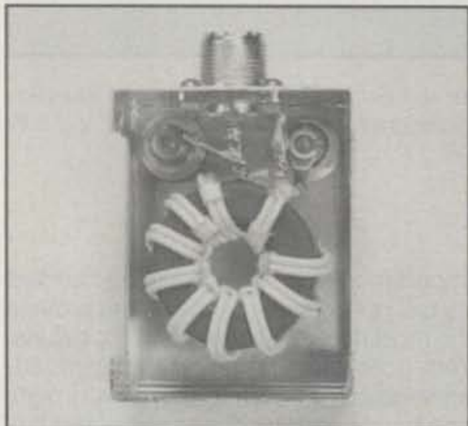
Photo E— Three different views of the low power 4:1 Ruthroff balun designed to handle the output of any HF transceiver. The enclosure is a 2.75"L x 2.125"W x 1.625"H CU-3000-A minibox.
