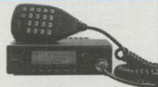
FT-2200 2 Meter Mobile With 50 Watts Output
