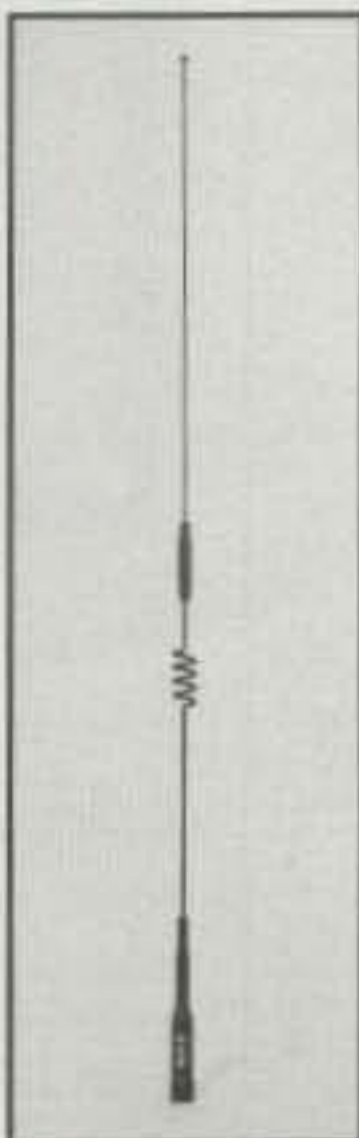
B-20/B-20NMO Dual-Band 146/446 MHz Gain & Wave: 146MHz 2.15dB 1/2 wave 446MHz 5.0dB 5/8 wave x 2 VSWR: Less than 1.5:1 144-148MHz, 440-450MHz Max Power: 50 watts Length: 30" Connector: PL-259 or NMO style Construction: Black, w/fold-over w/fold-Over
