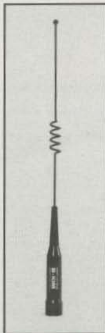
B-10/B-10NMO Dual-Band 146/446 MHz Gain & Wave: 146MHz -dB 1/4 wave 446MHz 2.15dB 1/2 wave VSWR: Less than 1.5:1 144-148MHz, 440-450MHz Max Power: 50 watts Length: 12" Connector: PL-259 or NMO style Construction: Black, cellular look-a-like w/fold-Over
