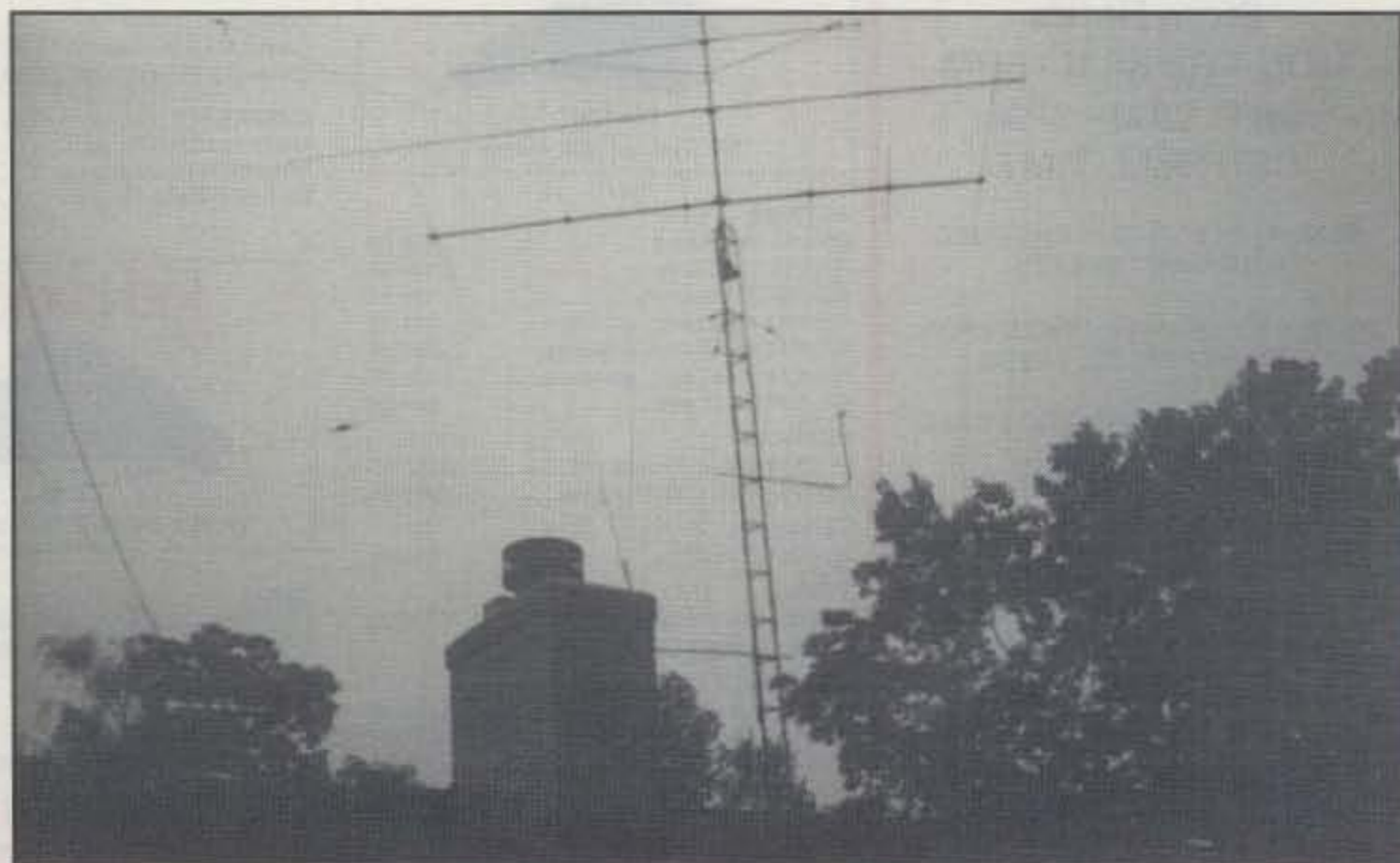
Those big signals you hear on the bands from Rex, WB8TDG, emanate from all those antennas. From top to bottom: 70 cm, 135 cm, 2 meters, and 6 meters. (Photo via WB8TDG)
