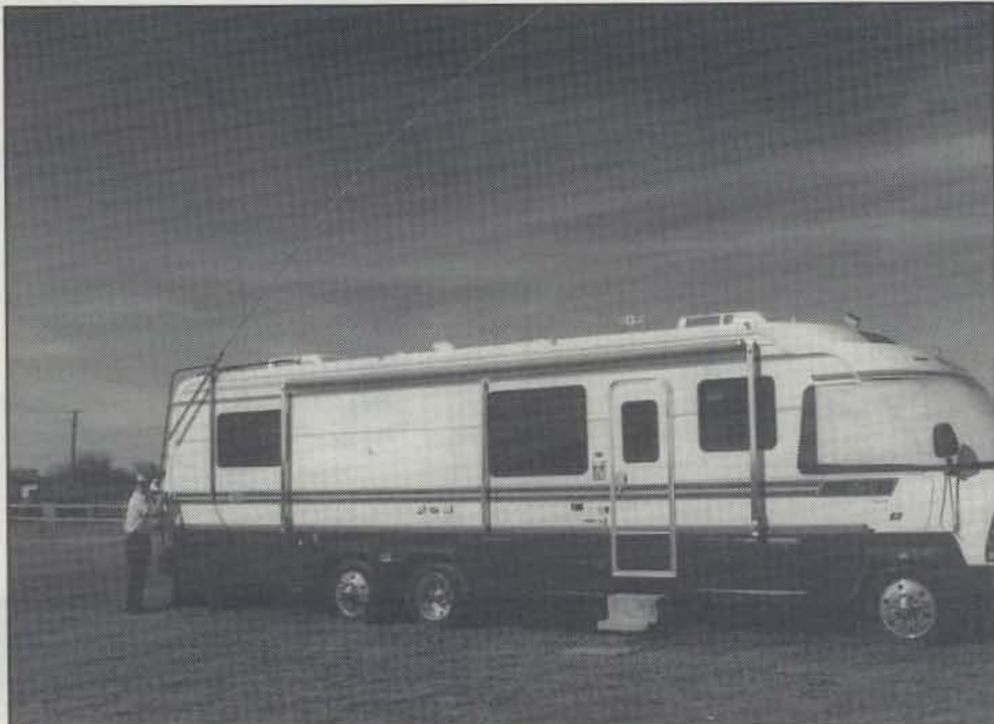
Photo 2—WDØP raising the folded monopole RV antenna from the horizontal traveling position to the vertical operating position.
