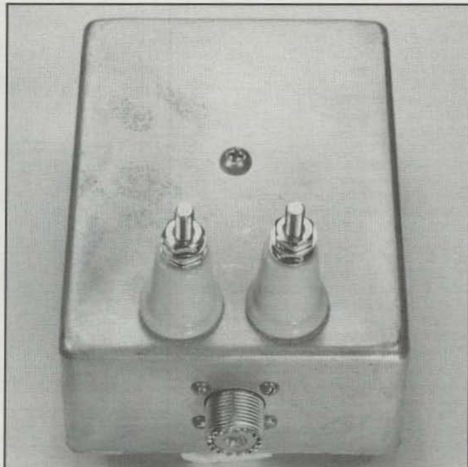
Photo B— Two different views of the optimized version of the 4:1 Ruthroff balun mounted in a 4"L x 3"W x 2.25"H Bud CU 234 aluminum enclosure.
