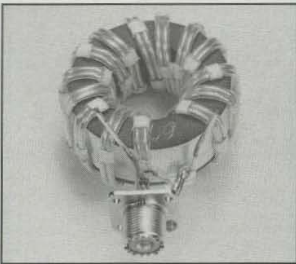
Photo D- Three views of the very high power 4:1 Ruthroff balun using two low permeability (40) ferrite cores. The aluminum enclosure has the dimensions 5"L x 3.5"W x 2.25"H.
