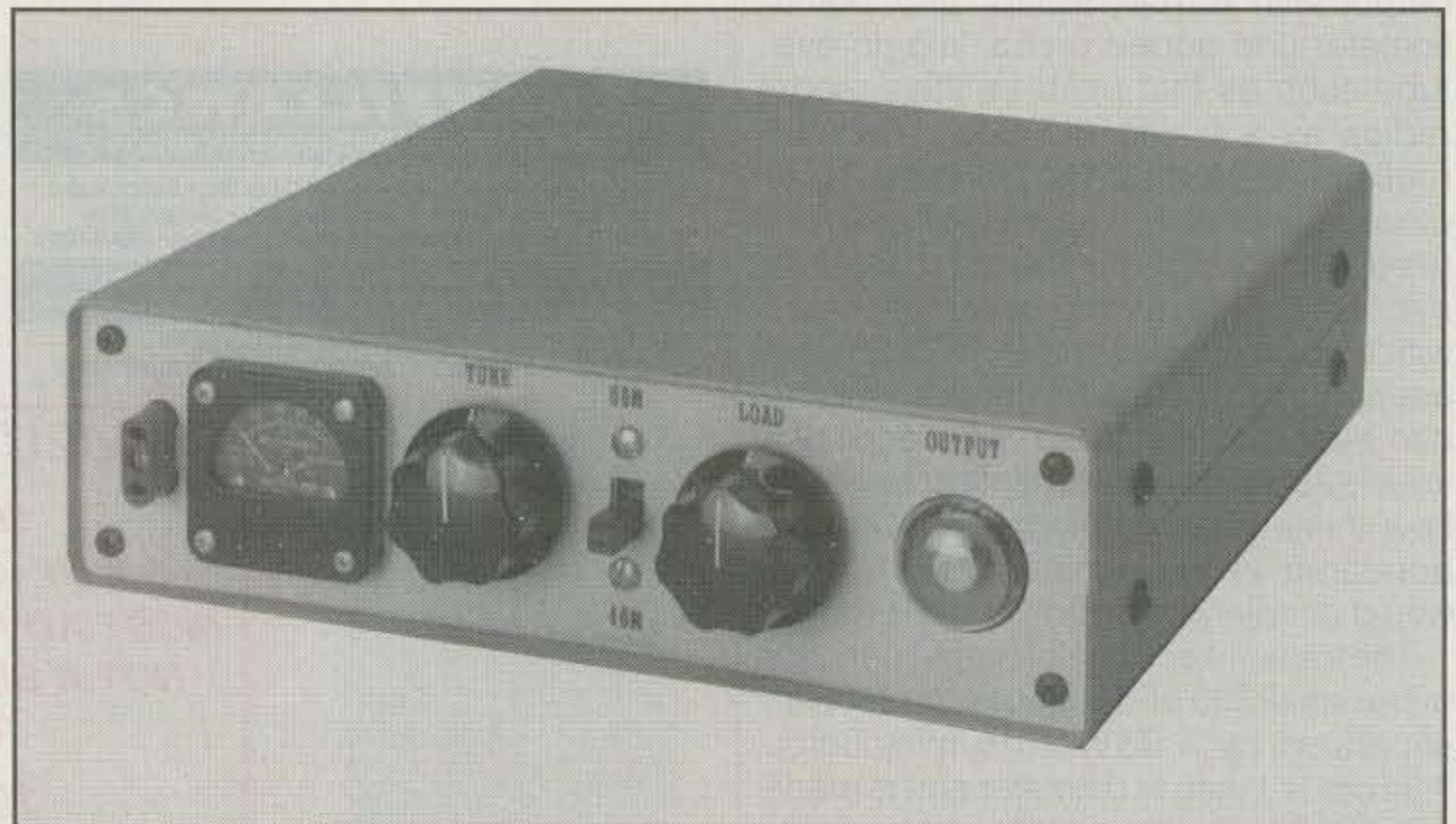
Fig. 5— Impressive homebrew 6AG7 transmitter built recently by Dave Ishmael, WA6VVL. Cabinet measures 2.5"H x 9"W x 9"D and has front "magic eye" tube for monitoring output. The on/off switch is mounted on the rear panel. (Photo courtesy Joe Veras, N4QB)
