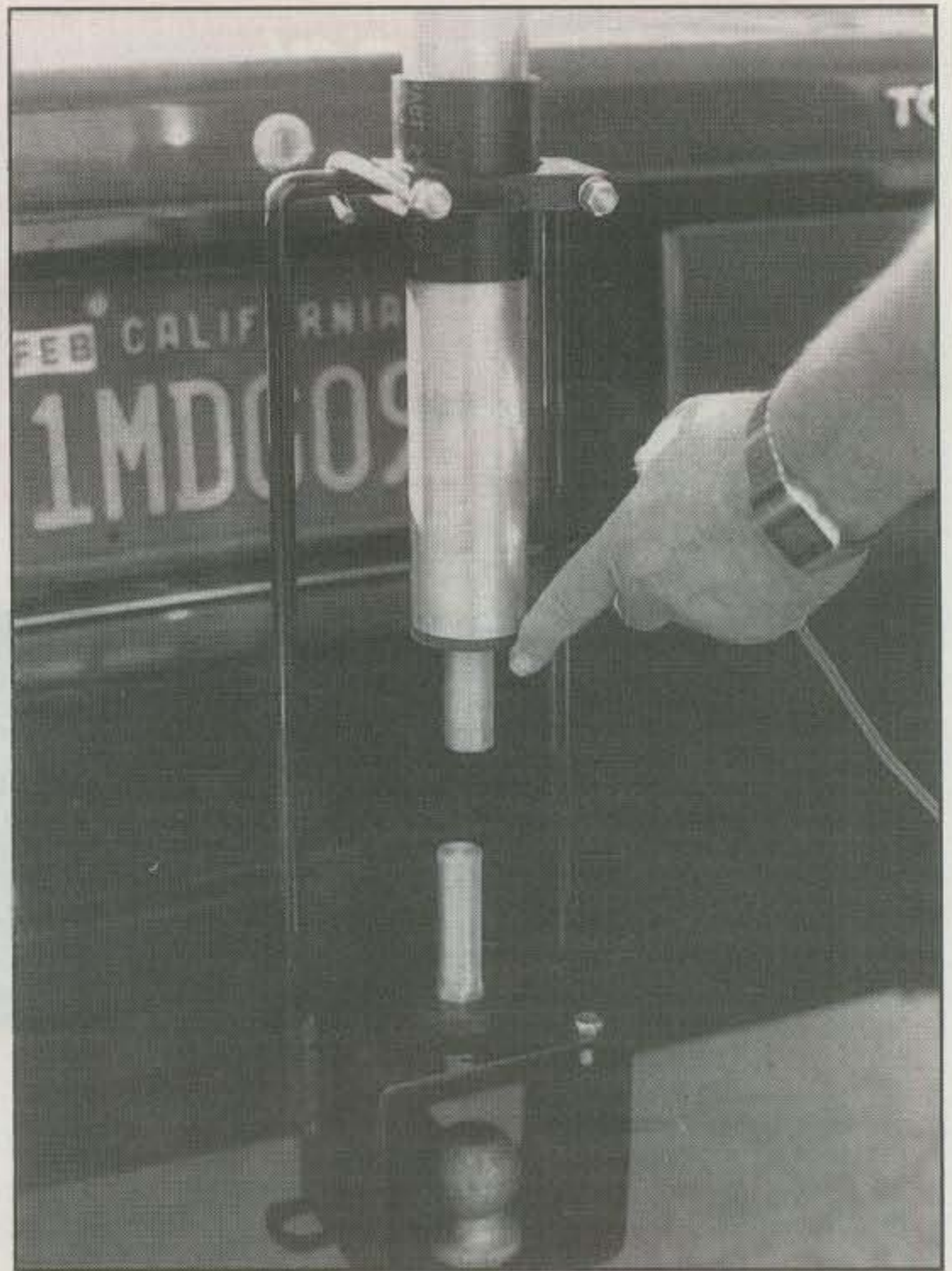
The base of the antenna has a tapered hole which fits down over the tapered solid bar mounted on the hitch fitting. The bottom of the solid bar has an insulated washer and is secured via a large nut (also the coax feed point). This makes an extremely efficient mount.
