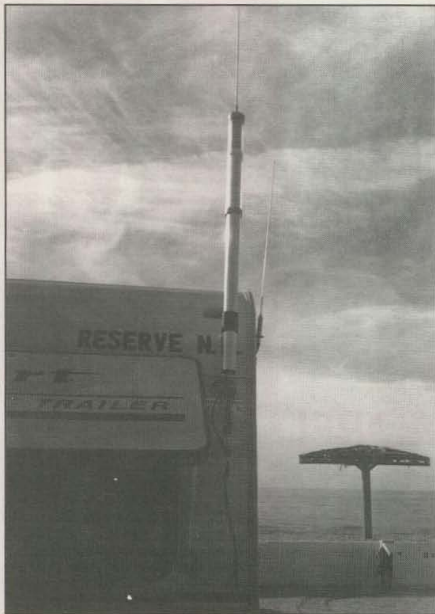
The High Sierra antenna mounted on my trailer. Note the convenience of the gate hinge for support. Of course, I do not use this when I'm moving, because the antenna is mounted high.
