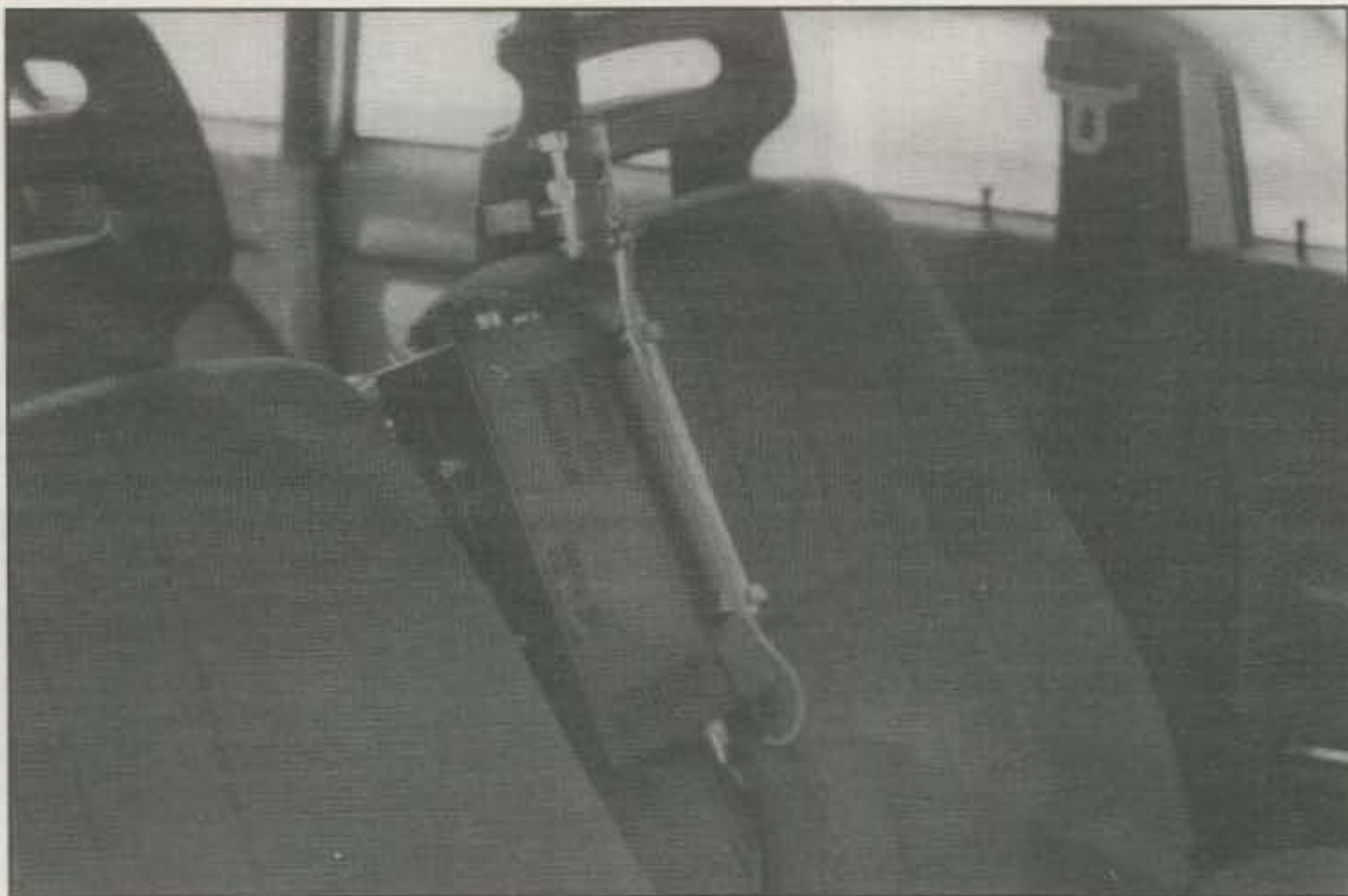
W9WBL's rig and paddle in "stowed" position, achieved simply by raising front armrest in car.
