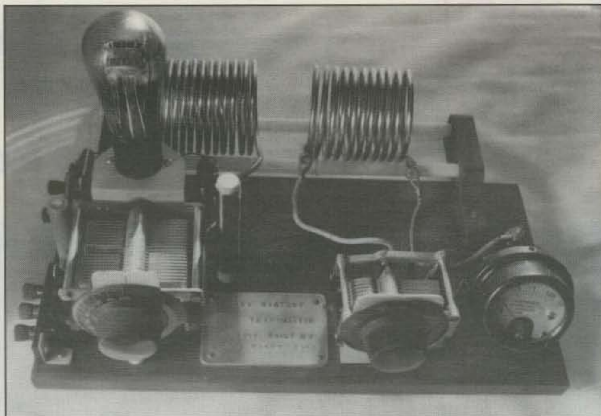
Replica of a "1929 Hartley" transmitter, built with several original parts, including the General Radio hot-wire ammeter for antenna current. The meter cost $2.50 on sale. Tube is a 7 1/2 watt 210. (Photo by Lewis Coe)
