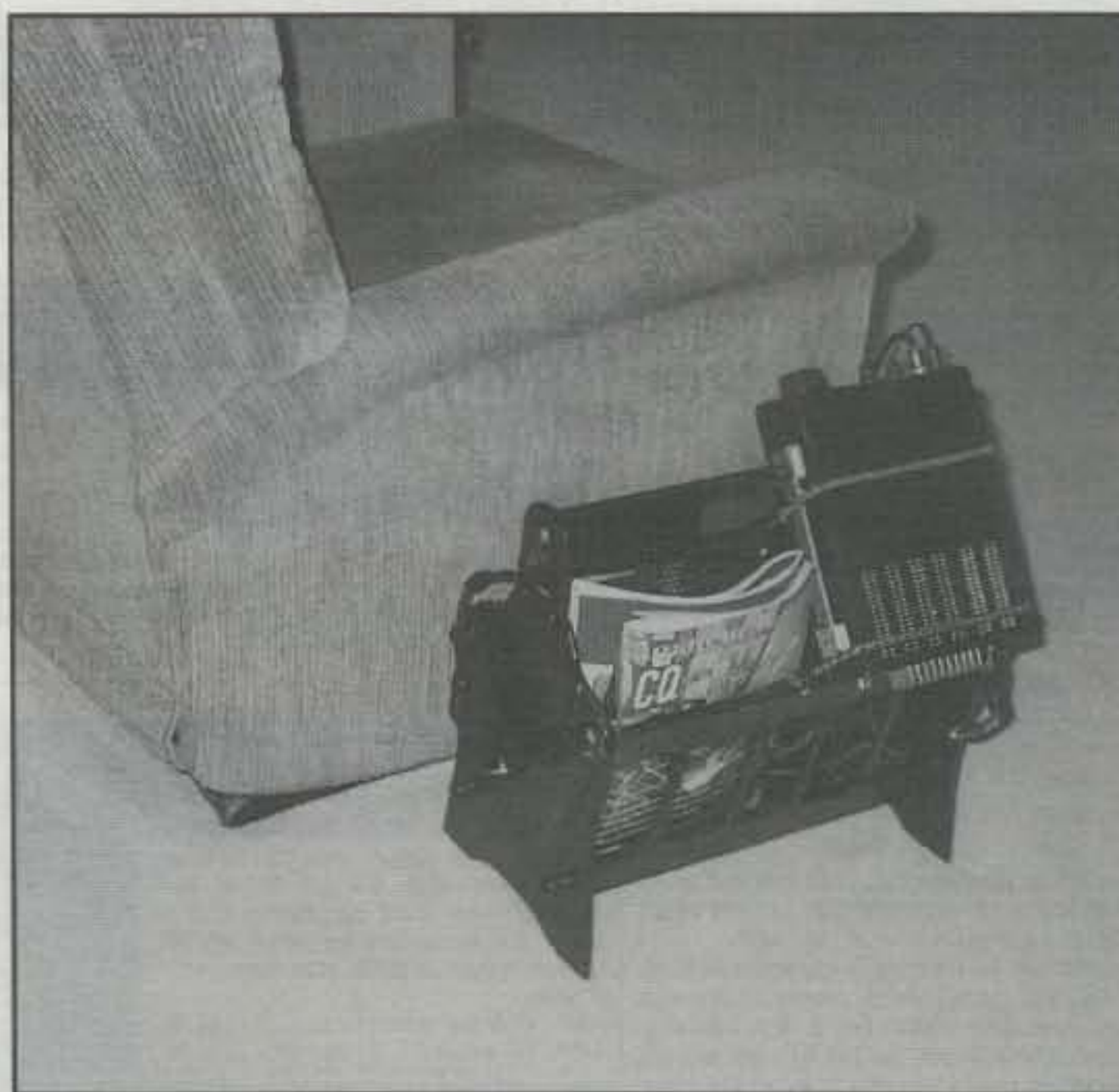
Photo 4— Opposite side view of W4CEC's "lift and go" magazine-rack shack. Power supply to transceiver cable is inside the rack. Earphones and mic hook on the side. Bungee cords hold the gear securely.
