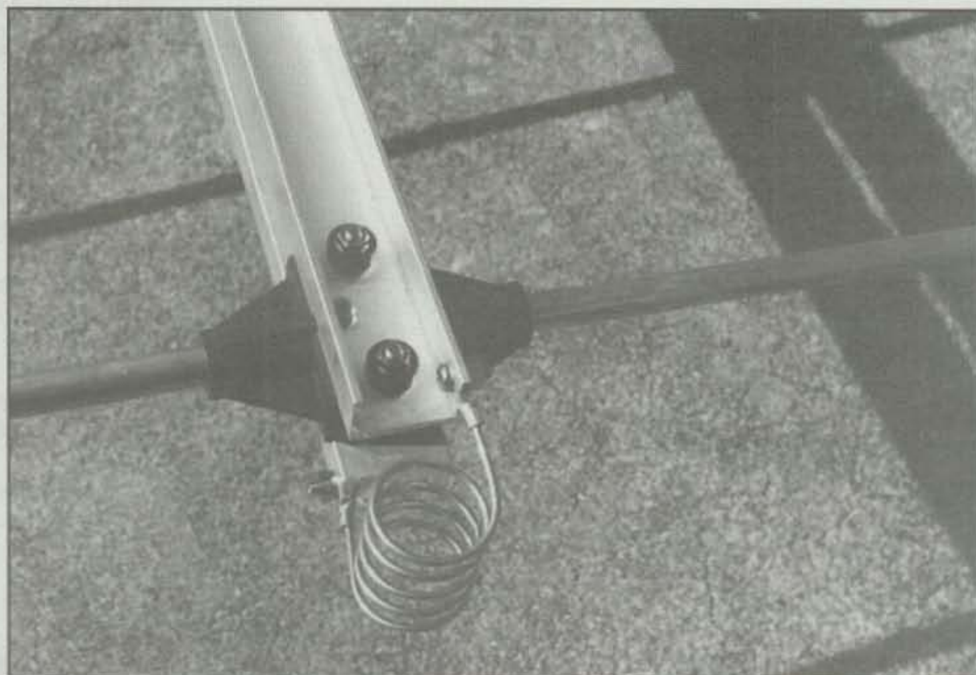
The Arrestor coil is the last item to be installed. You might want to wait to install it just prior to installing the antenna in order to keep from accidentally crushing it.
