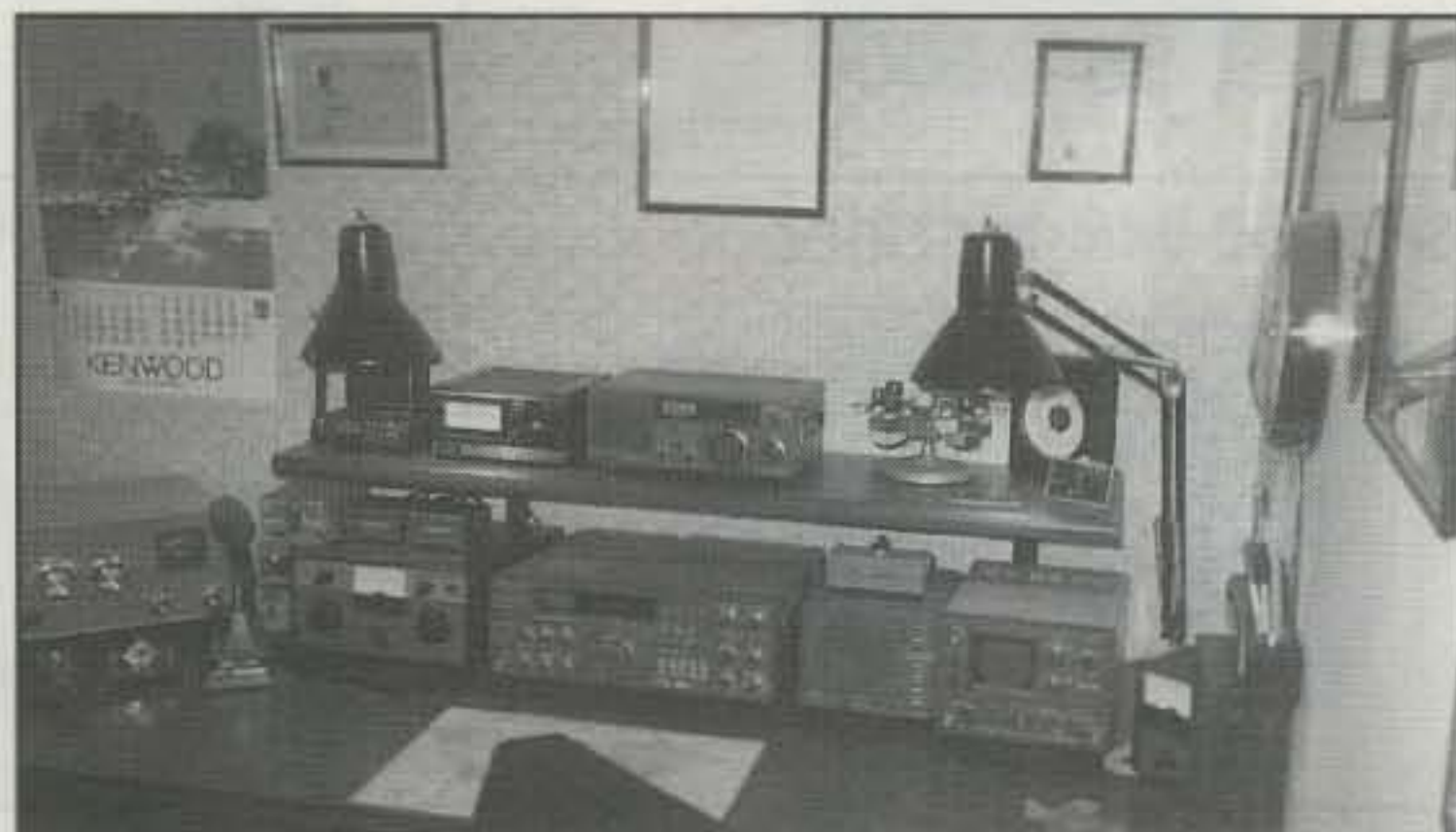
The main requirement for most satellites is for multimode 145 MHz and 435 MHz transceivers and a suitable RF power amplifier. These photos show a typical satellite-capable hamshack, this one belonging to Keith Baker, KB1SF. Primary equipment for satellite communications are Kenwood TS-711A (145 MHz) and TS-811A (450 MHz) transceivers, plus an RF Concepts RF power amp. The portable hamshack gear consists of a Ten-Tec "Mode B" (435 MHz uplink/145 MHz downlink) converter to a Kenwood TS-50S. (KB1SF photos)
