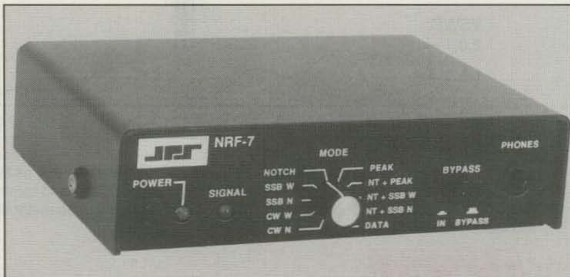
The JPS NRF-7 general-purpose audio processing unit.
