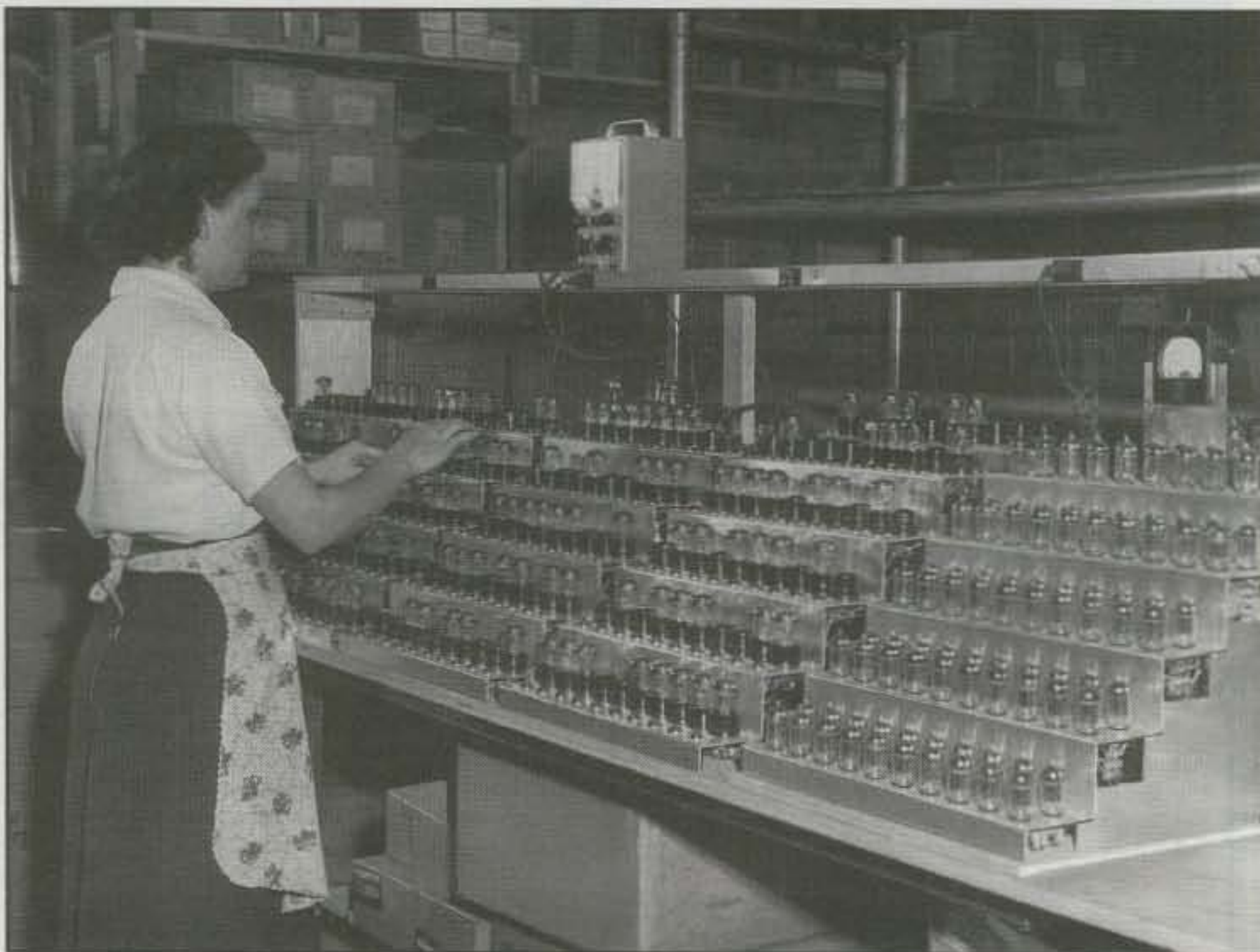
Heathkits ranged from the 1947 oscilloscope and vacuum tube voltmeter (VTVM) to the last Heath amateur radio product, the 1991 intelligent antenna rotator. Shown in this classic photo are some of the war surplus 6H6 vacuum tubes (used in thousands of VTVM kits) being aged in racks to assure stable performance in the completed kits. (Photo courtesy Terry Perdue, K8TP)
