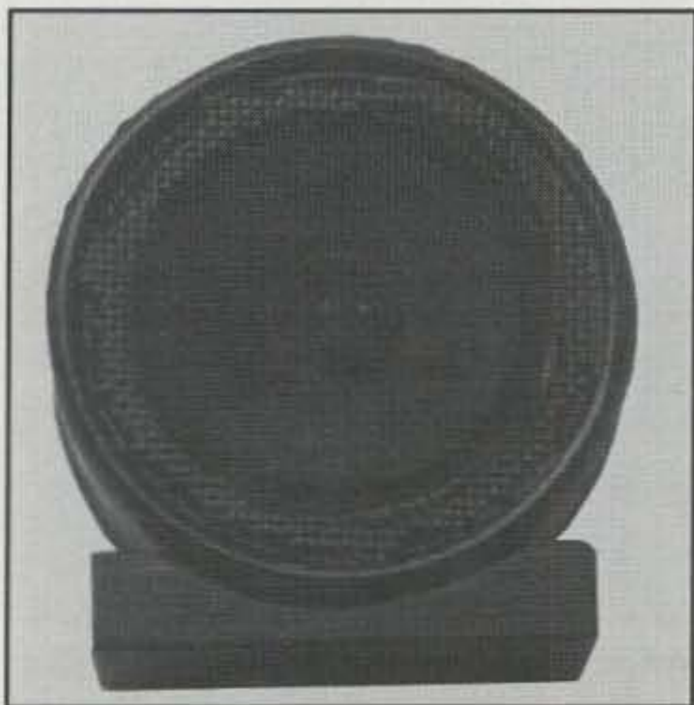
Photo 4- A speaker can be enclosed in a food container at low cost. This photograph shows W1FB's portable speaker housed in a tuna fish can. The grill is a piece of metal window screen.
