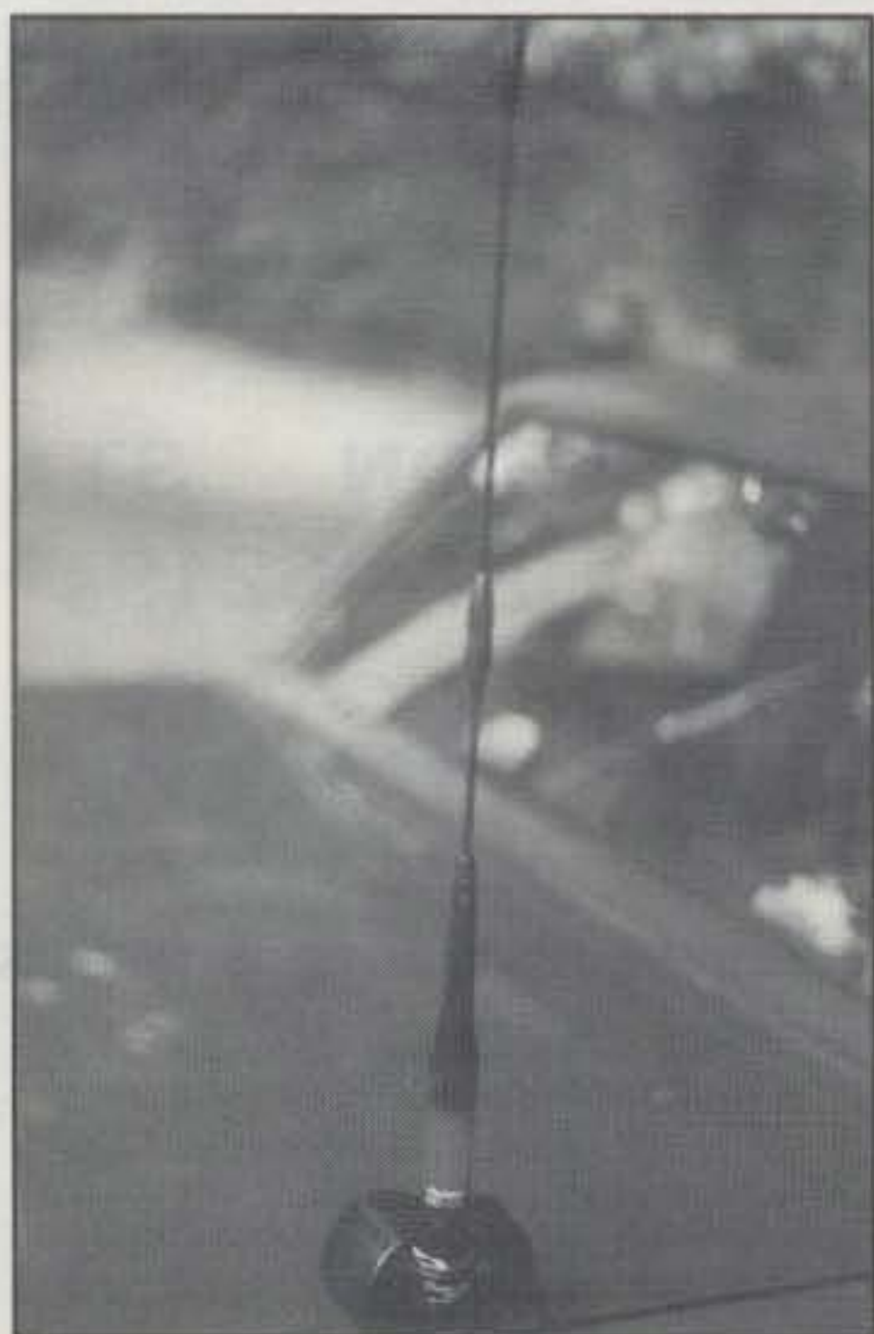
Photo 2—Maldol's MK-30 motorized tilt-over trunk-lid mount with ARD-12B gain antenna for 2 meters and 70 cm installed. Unit is remote-controlled from car's dash and works great!
