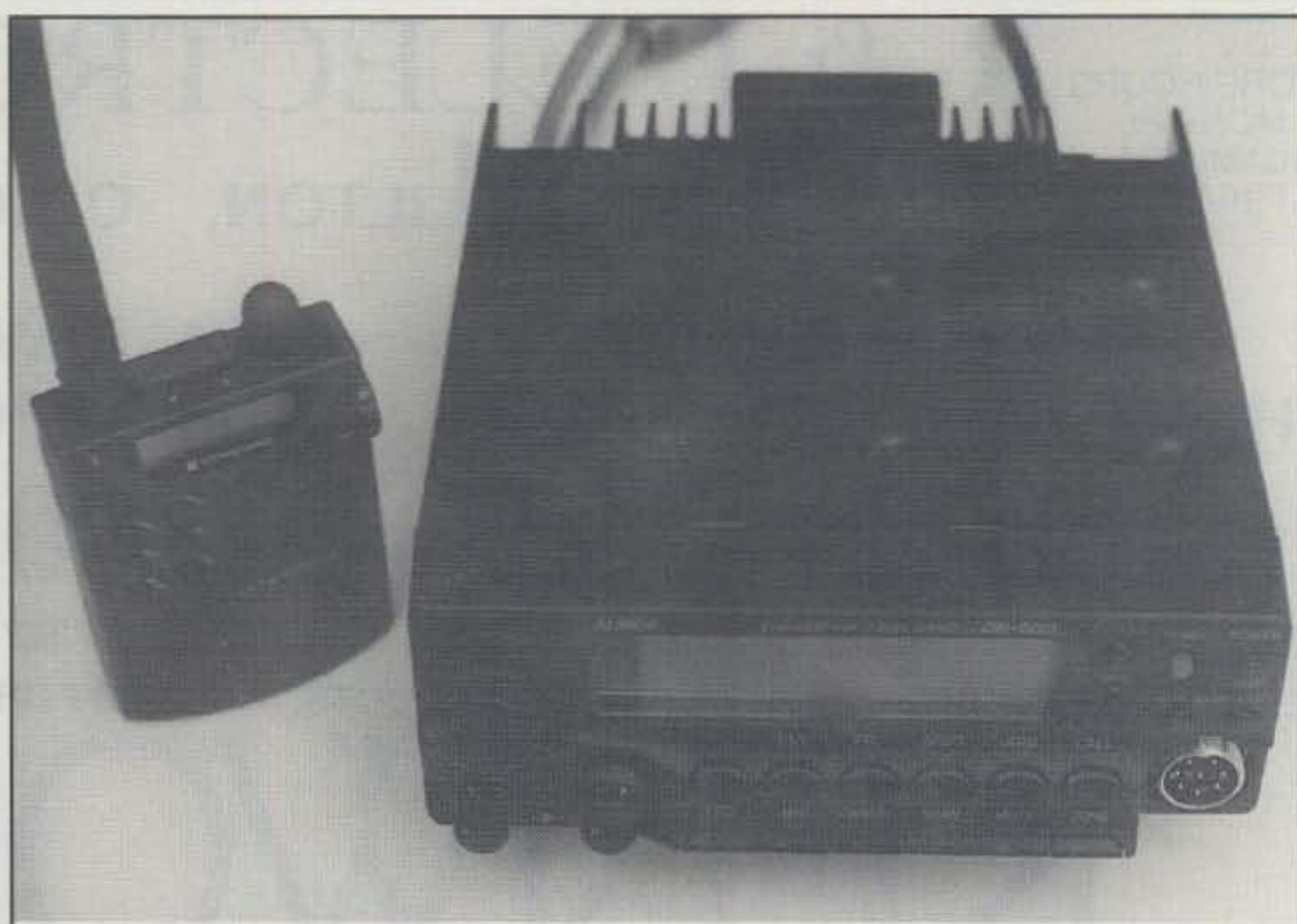
Photo 3—Main equipment used for crossband repeating: a good 2 meter/70 cm mobile FM transceiver and a trim FM handheld for 70 cm or 2 meters/70 cm. Handheld shown is Standard's new C-108, which is incredibly small (1" x 2" x 3") and available in 2 meter or 70 cm versions.
