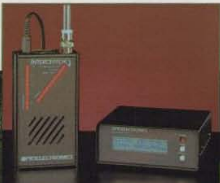
R10 checks coded squelch codes with DC440 Decoder
