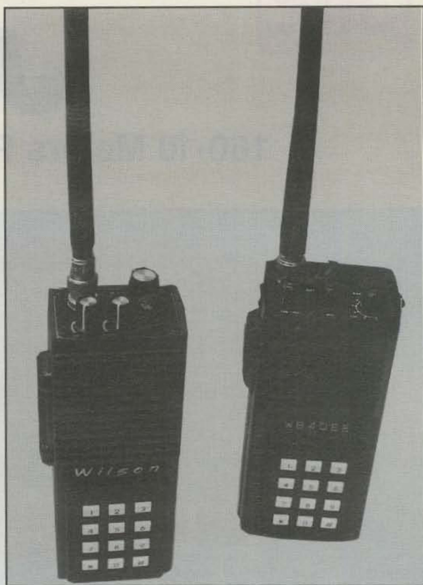
Photo 6— Two mid-sized talkies that bridged the size gap between early model "bricks" and modern miniature handhelds. Unit on the left is a Wilson Mark II, and on the right is the FDK Palm II. Both radios are crystal-controlled delights.
