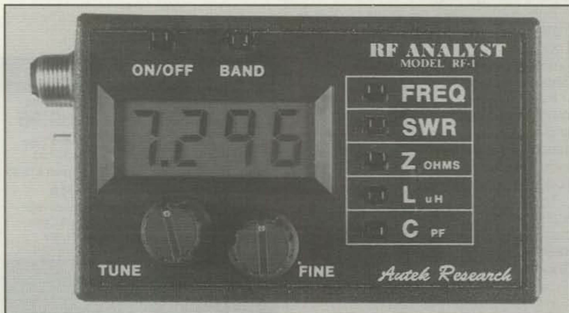
The Autek Research RF-1 RF Analyst is intended to be the only instrument you need to adjust any antenna. It greatly simplifies the construction, measurement, and adjustment of antennas, transmission lines, tuners, and RF networks from 1.2 to 35 MHz. Besides measuring SWR with its built-in "transmitter," it's reportedly the first affordable digital impedance (Z) meter. The RF-1 also calculates L (inductance) and C (capacitance). (Photo courtesy Autek Research)
