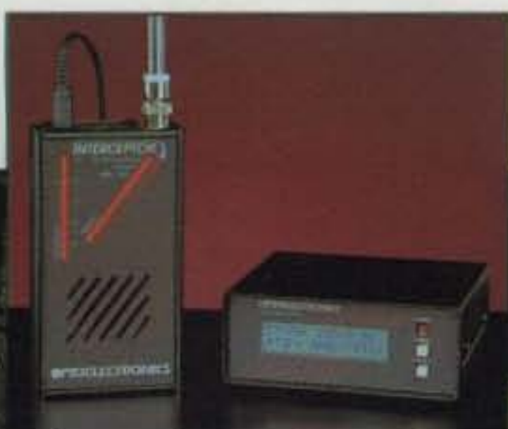
R10 checks coded squelch codes with DC440 Decoder
