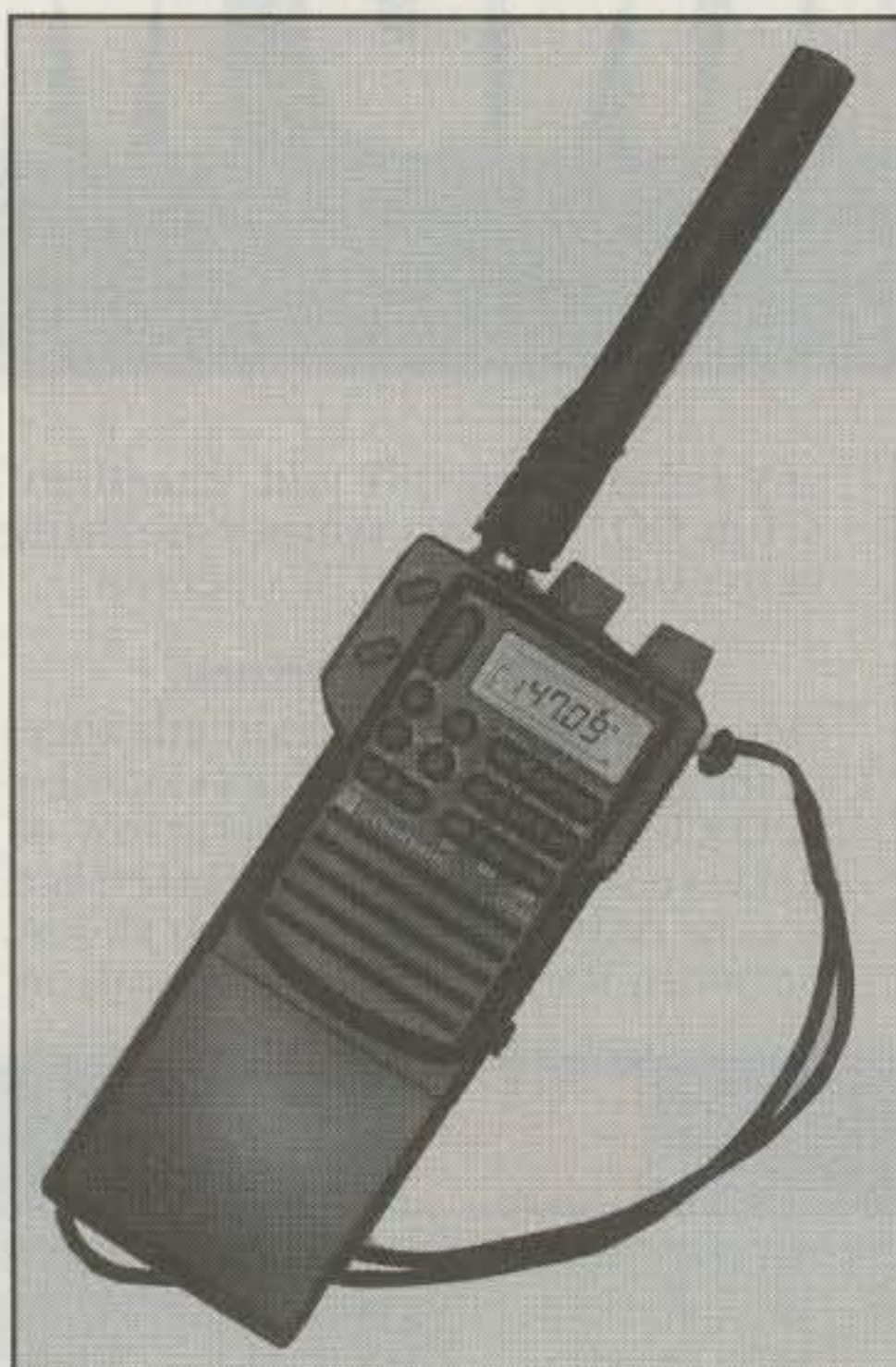
Standard C158A hand-held, shown with the provided 7.2 volt, 700 mA nickel-cadmium battery pack. Push-to-talk is on the raised portion of the left side of the case, with the Function key just above it.
