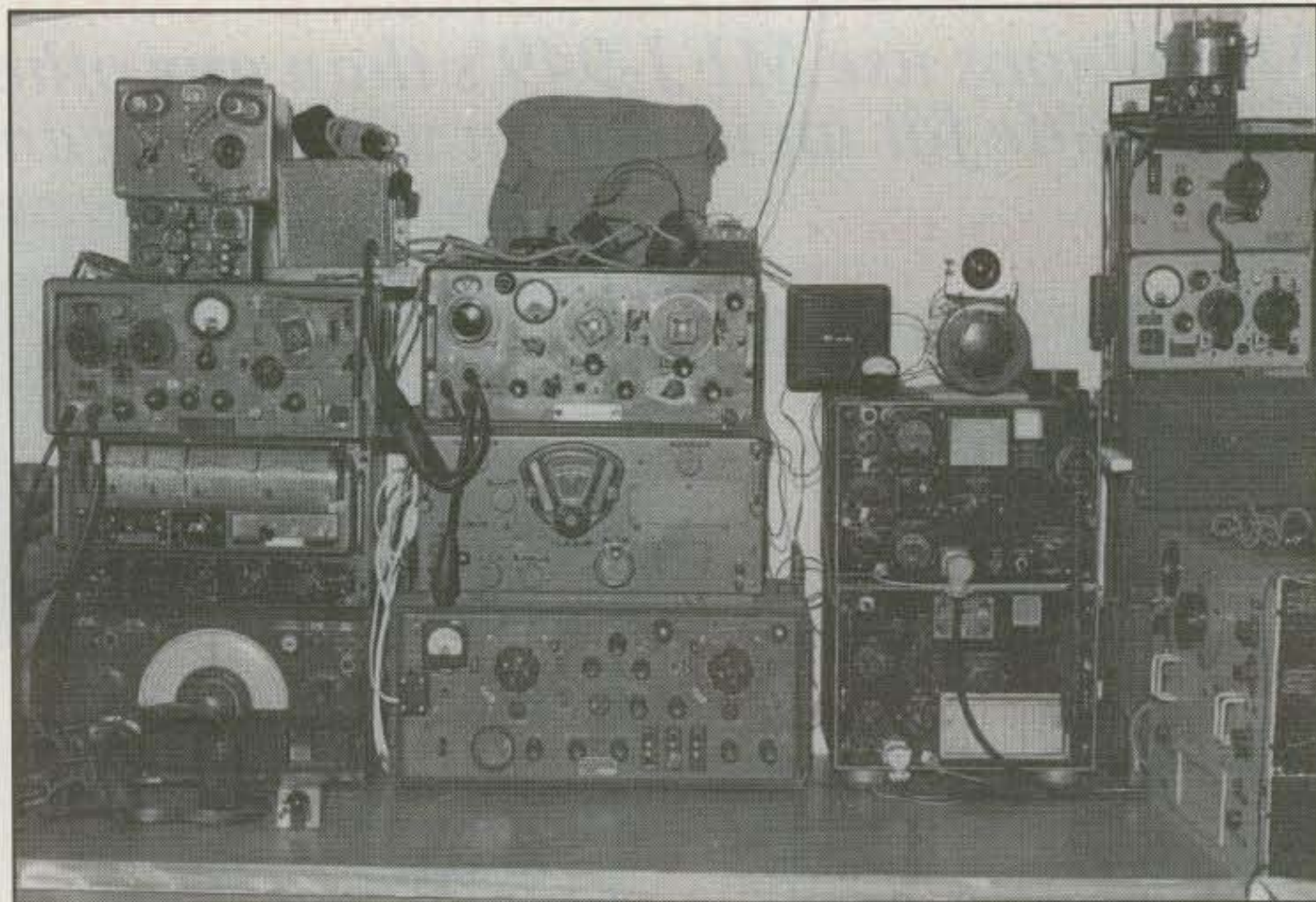
Units are described by stack, left to right. Left stack: Russian antenna tuner, below is the 46 set, then the 62 set, the R1475, and R1155. Stack second from left: top 22 set, then BC-348q, and ZC1 Mk II. Next stack: TCS 6 and 12 setup. Right stack: top 18 set, another 18 set, and HRO rack-mounted receiver and power supply.
