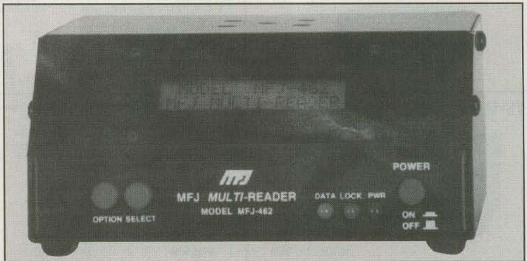
Photo 7— Need a "back-up assistant" for copying code (or RTTY!) off the air? Connect this new MFJ-462 to your transceiver's earphone socket and it prints incoming text right on its built-in screen. A discarded printer can even be plugged directly into it for a hard-copy readout!
