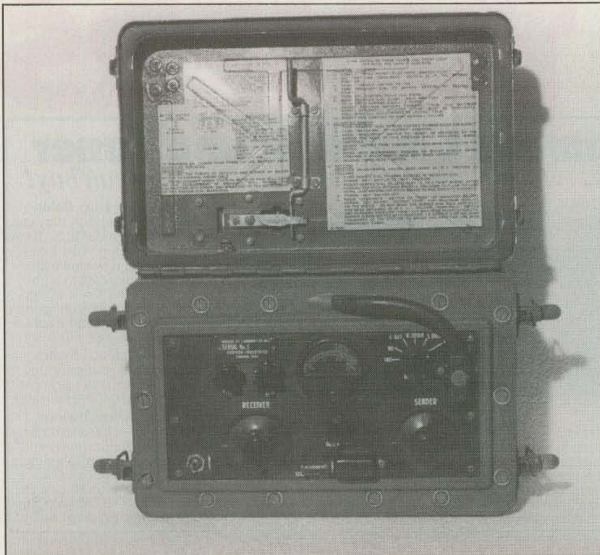
The CND 58 set. The rod on the lid pushes against the RX/TX switch located on the bottom center of the set when the lid is closed.
