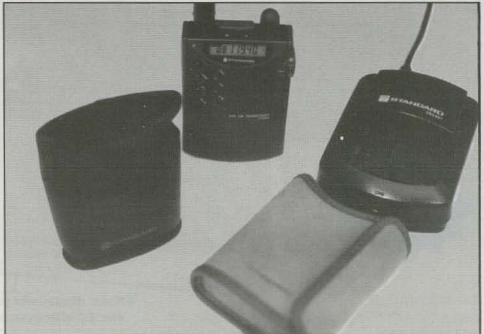
Photo 1— The world's smallest 2 meter handheld transceiver, Standard's C108A, is a heart-throb any amateur would love. Unit is easy to operate, has extended receive without modification, and hides in the palm of your hand. It is shown with optional charger, vinyl case, and quick-draw belt pouch.
