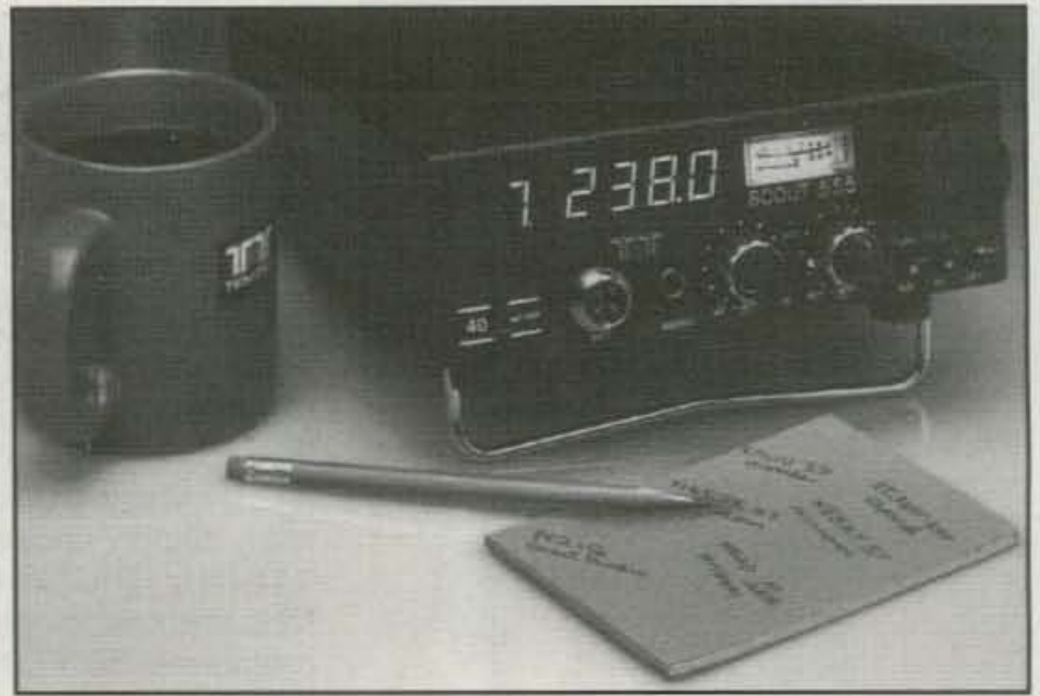
Photo 5— Gearing up for low-band fun need not be expensive: Ten-Tec's Scout proves that fact every day. The Scout runs 50 watts and has several impressive features. It is a real "fun rig!"
