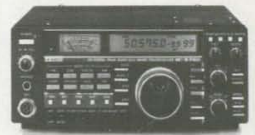
IC-575H • 100 W • Multi Mode • 28 MHz (10 M)/50 MHz (6 M)
