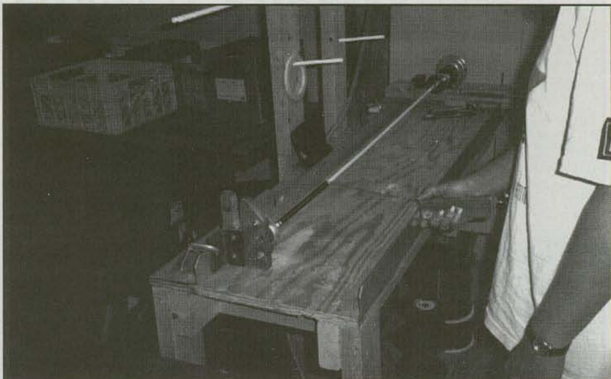
Here a Lakeview employee patiently winds a Hamstick, one of the company's most popular and most widely imitated products. Your columnist always wondered how they wound those things! (N4WHB photo)
