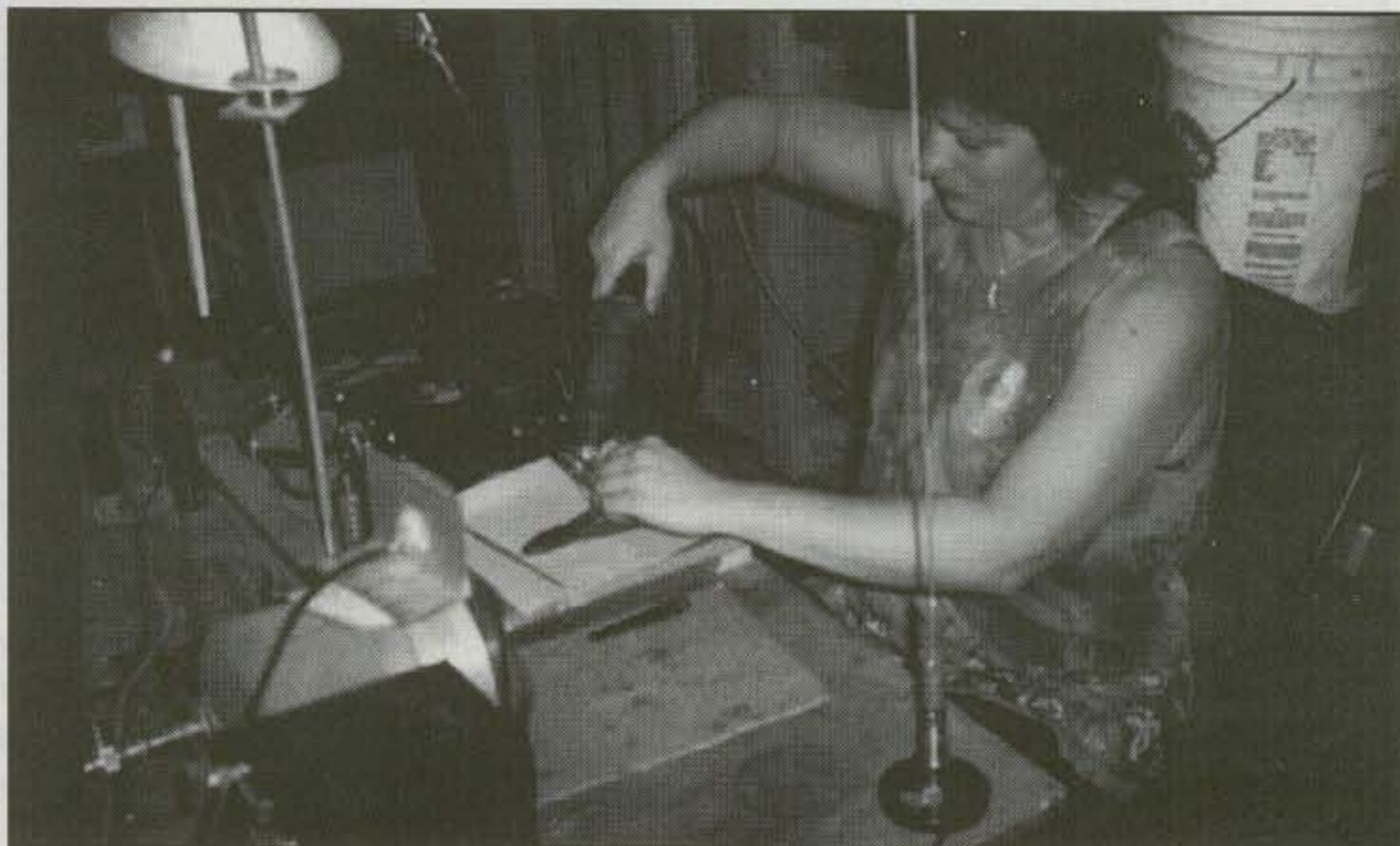
In this photo a Lakeview Company worker is shown busily hand-winding a VHF antenna coil. All the products are made in the Anderson shop using American-made parts. (N4WHB photo)
