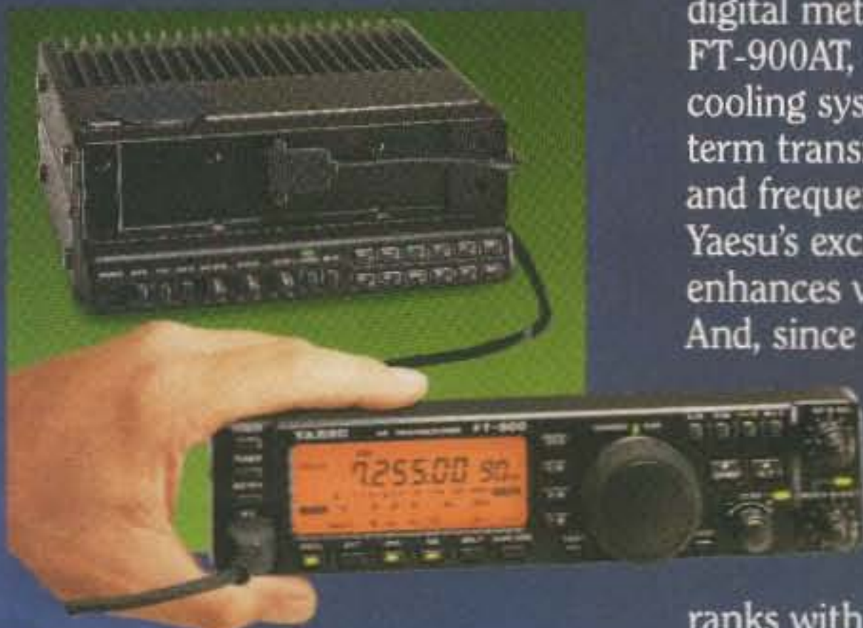
Remote front panel control head measures only 2-1/4"H x 9-1/8"W x 1-1/4" D.
