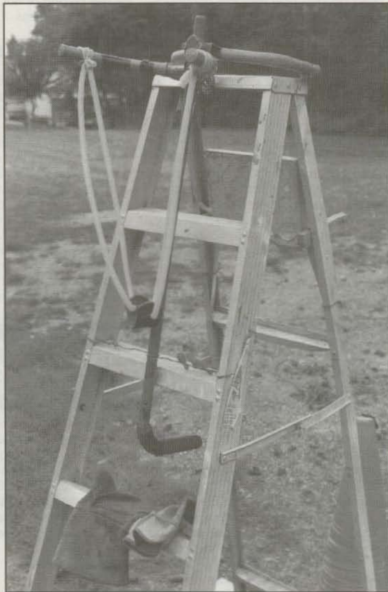
The A1M1 slingshot as described in the text. The highway cone in the front spools the monofilament line. Two of the weights can be seen on the second rung down of the ladder.
