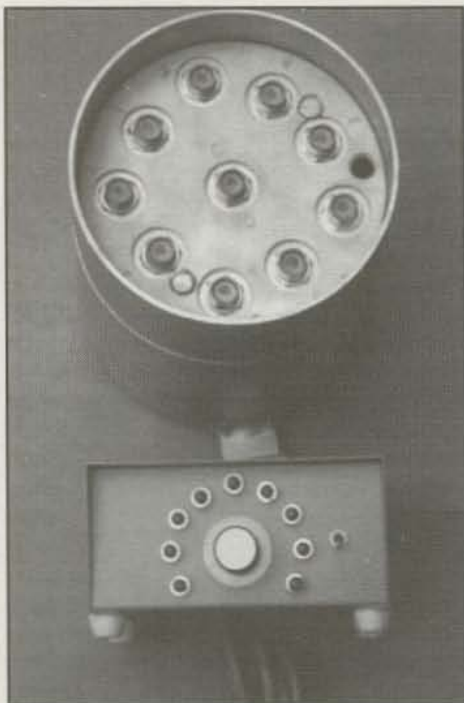
Photo 4- At the top is the tower mounting section of the nine-terminal antenna switch. This switch is extremely rugged, handling 7000 volt peaks, with a 20 ampere current-carrying capacity. At the bottom in this view is the control unit, which is installed at the operating location. Obviously, you can label the LED indicators to suit your own needs.
