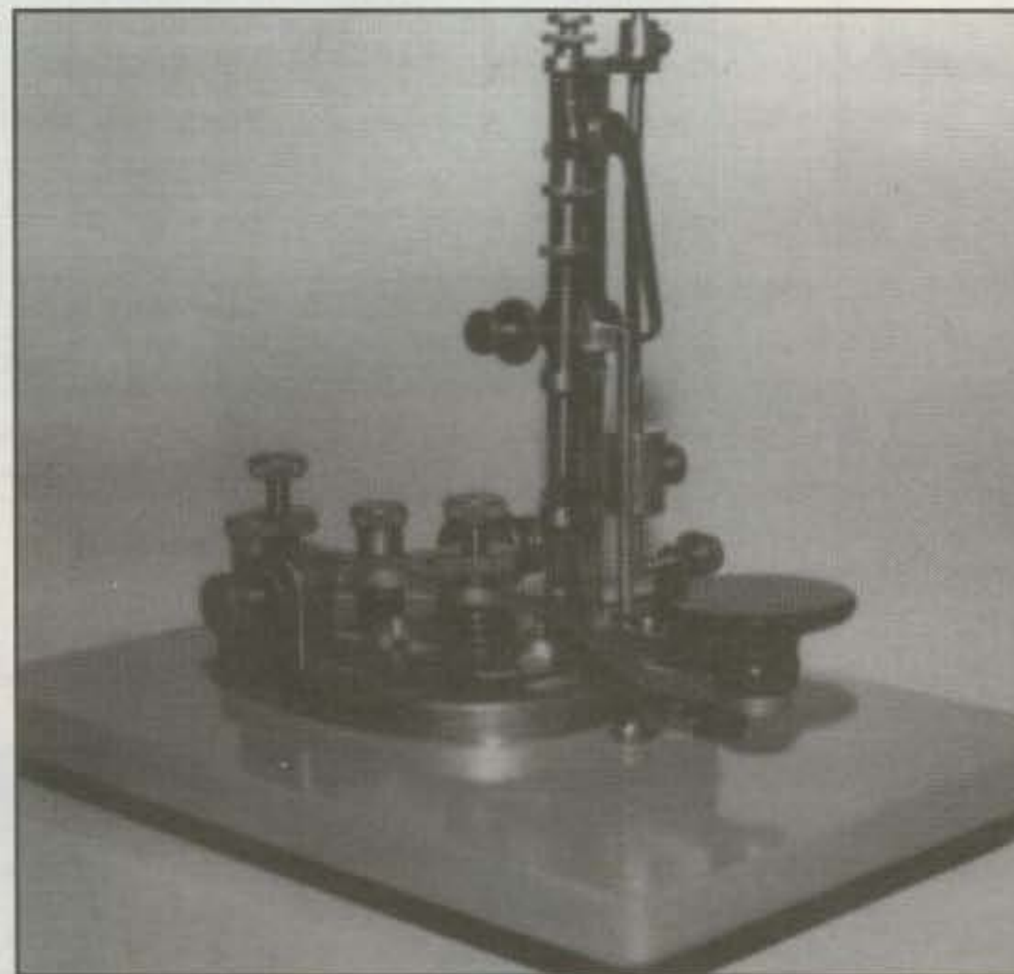
Photo 8- The stack of vertically standing rods attached to the hand key in this photo turns it into a bug. Honest! Pull up for dots; press down for dashes! Details in text. (Special photo thanks to owner Gil Schlehman, W9WDY)
