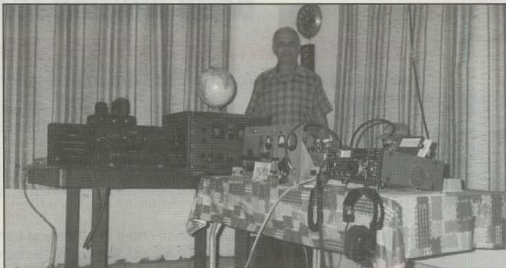
The shack of Giuseppe (Pino) Picataggi, YV7MB, of Los Altos de Santa Fe, Venezuela, includes an ICOM IC-740 transceiver. However, Pino's favorite transmitter is a homebrew unit featuring a pair of 807 tubes in the final RF stage and a Geloso variable frequency oscillator. He uses a Hammarlund Super Pro receiver and a war surplus BC-224 receiver with his homebrew transmitter.
