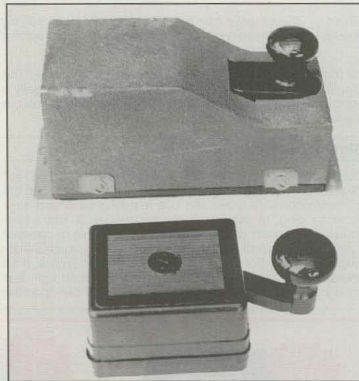
Photo 13— Two popular styles of Russian hand keys used a couple of decades ago. Items are designed to "take a licking and keep on ticking."
