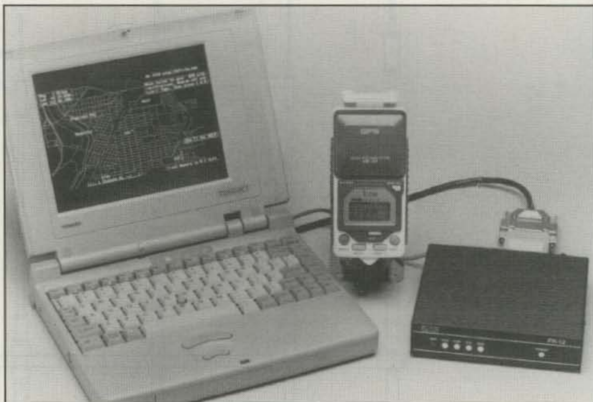
Photo A— The AEA PK-12 in a GPS system.
