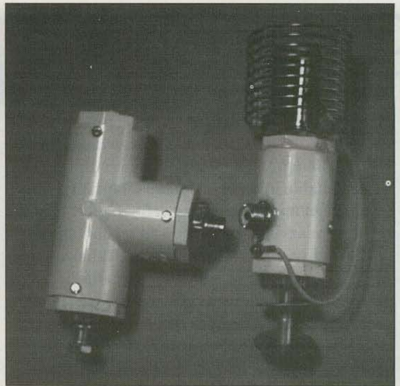
↑ In this variation a switch/capacitor assembly is readied for internal mounting.
