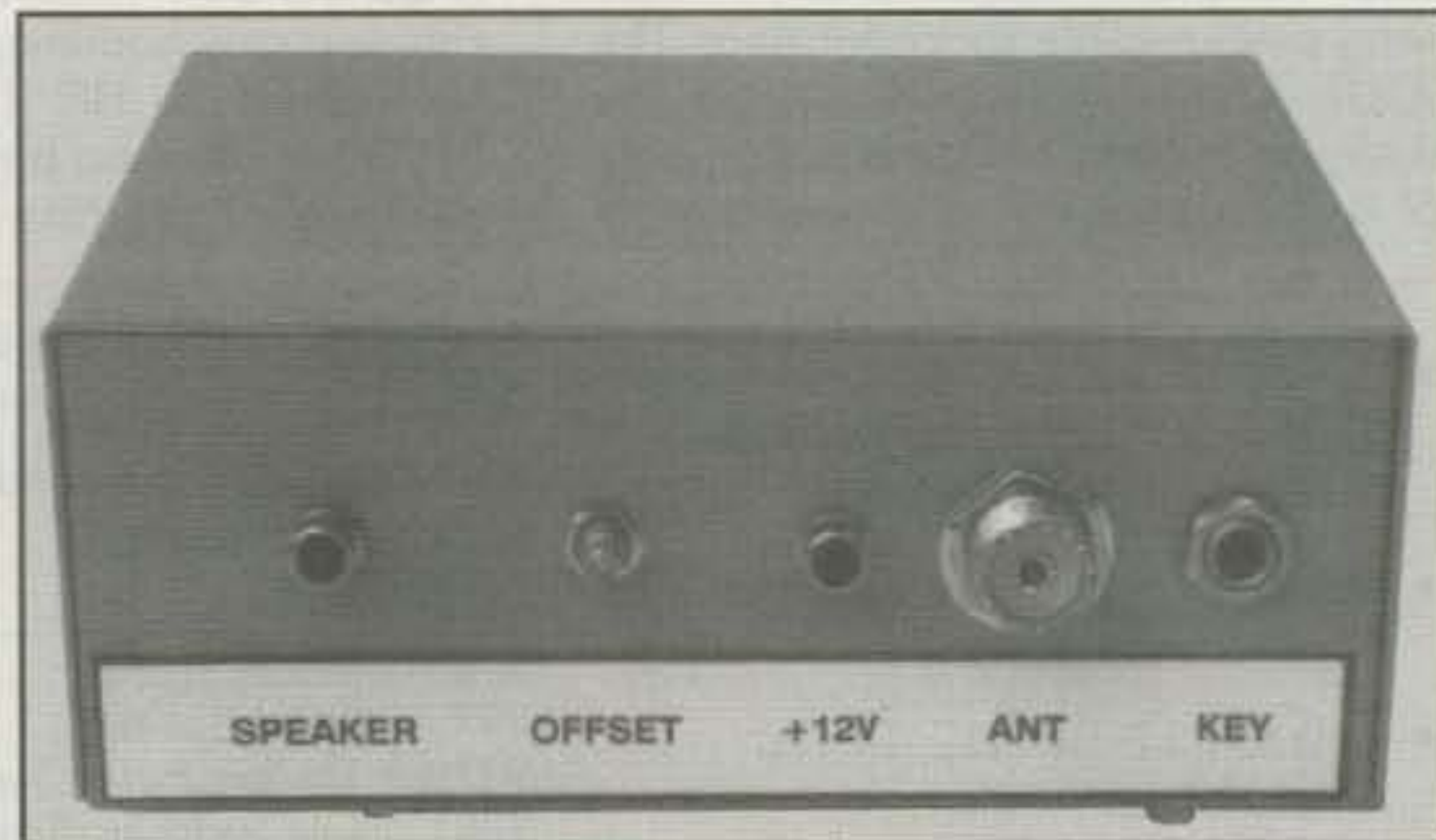
View of the rear panel of the transceiver. The offset control is for setting the BFO for the desired beat frequency tone. The front and rear panel paste-ons were computer-generated and printed on poster board with a laser printer.
