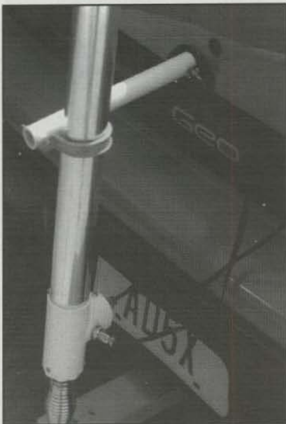
The mobile mount for the Big DK3 includes a matching transformer. The additional cables supply power for the motor.
