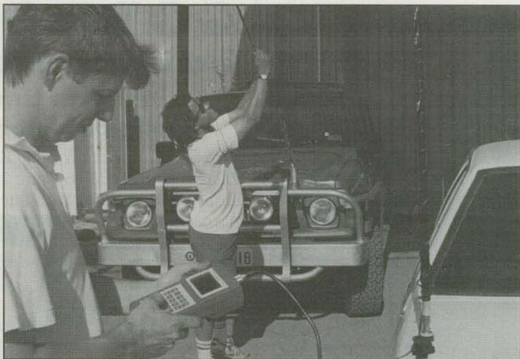
Photo 4—Terlin Aerial's outdoor tuning and test facility in western Australia. Note the Outbacker mobile antennas are being checked for low SWR and wide bandwidth with an AEA Antenna Analyzer. (Photo via Don Arnold, WD4FSY)
