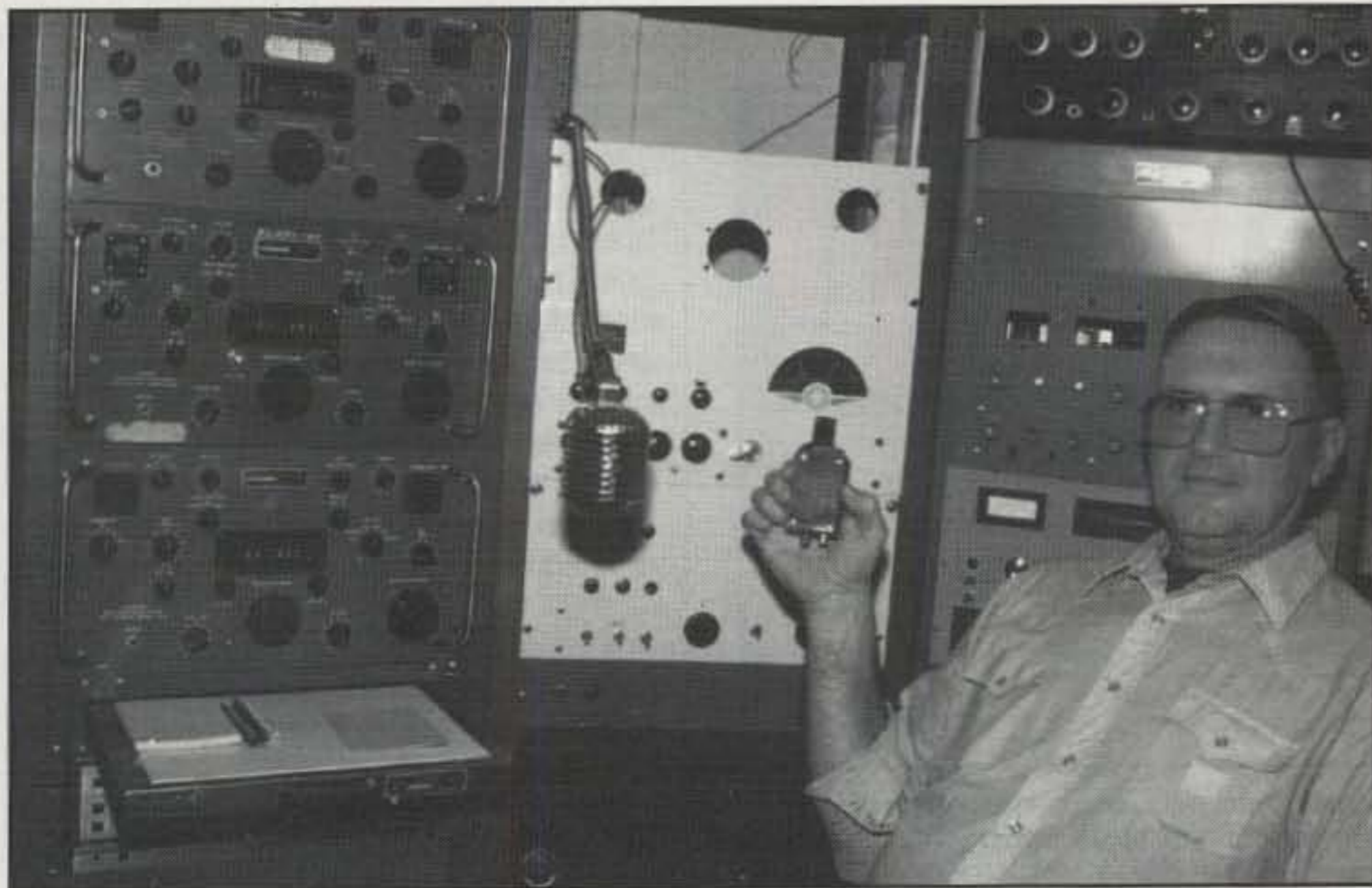
"Radio Free Larksville," aka Joe Hilenski, WA3WMI, sits in front of his AM rig (a rack of four R-390 receivers and a Hallicrafters HT-37 transmitter, modified to fit in a 19 inch rack panel). Joe is holding his homebrew 40 meter QRP rig. Joe and his son, Lou, KA3ICD, share an immaculate shack that features many rigs from the 1950s and '60s, not to mention several homebrew QRP creations. (Photo by K7YHA)
