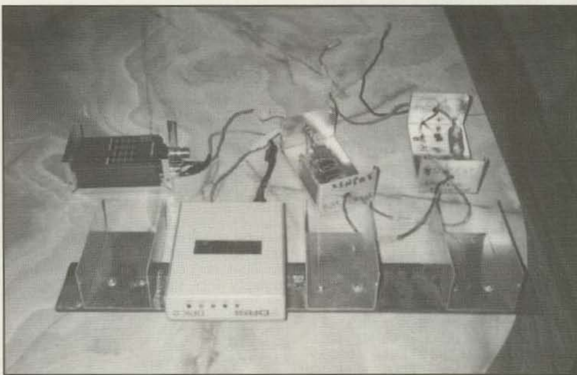
The basic VE7PMR packet node: an HT, a TNC, and some control boxes. These components plus three heavy-duty solar-powered batteries keep it operating flawlessly.
