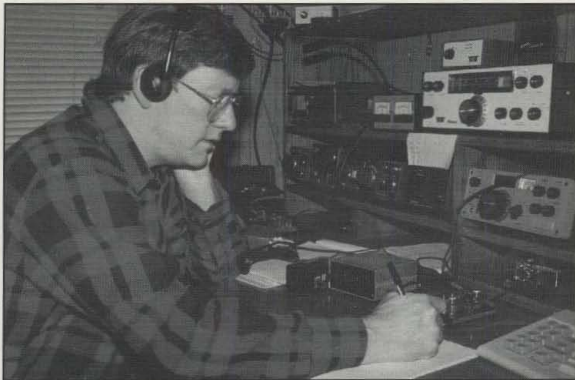
Paul Stroud, AA4XX, sits at the controls of K7YHA and uses a NorCal-40 to work the Michigan QRP Club QSO Party, January 9, 1995. Other station equipment: left to right, bottom shelf, a complete Kenwood TS-130V station and a Ten-Tec Century-22; top shelf, rotor control box, wattmeter, and a Ten-Tec Argonaut 509 with audio filter. Antennas consist of full-size dipoles for 80, 40, 30, and 20 meters and a TH7DX at 52 feet. (Photo by K7YHA)
