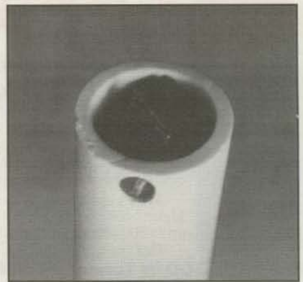
Photo F- Close-up view of the top of an antenna showing the 1/4 inch plastic rod supporting the twin-lead.
