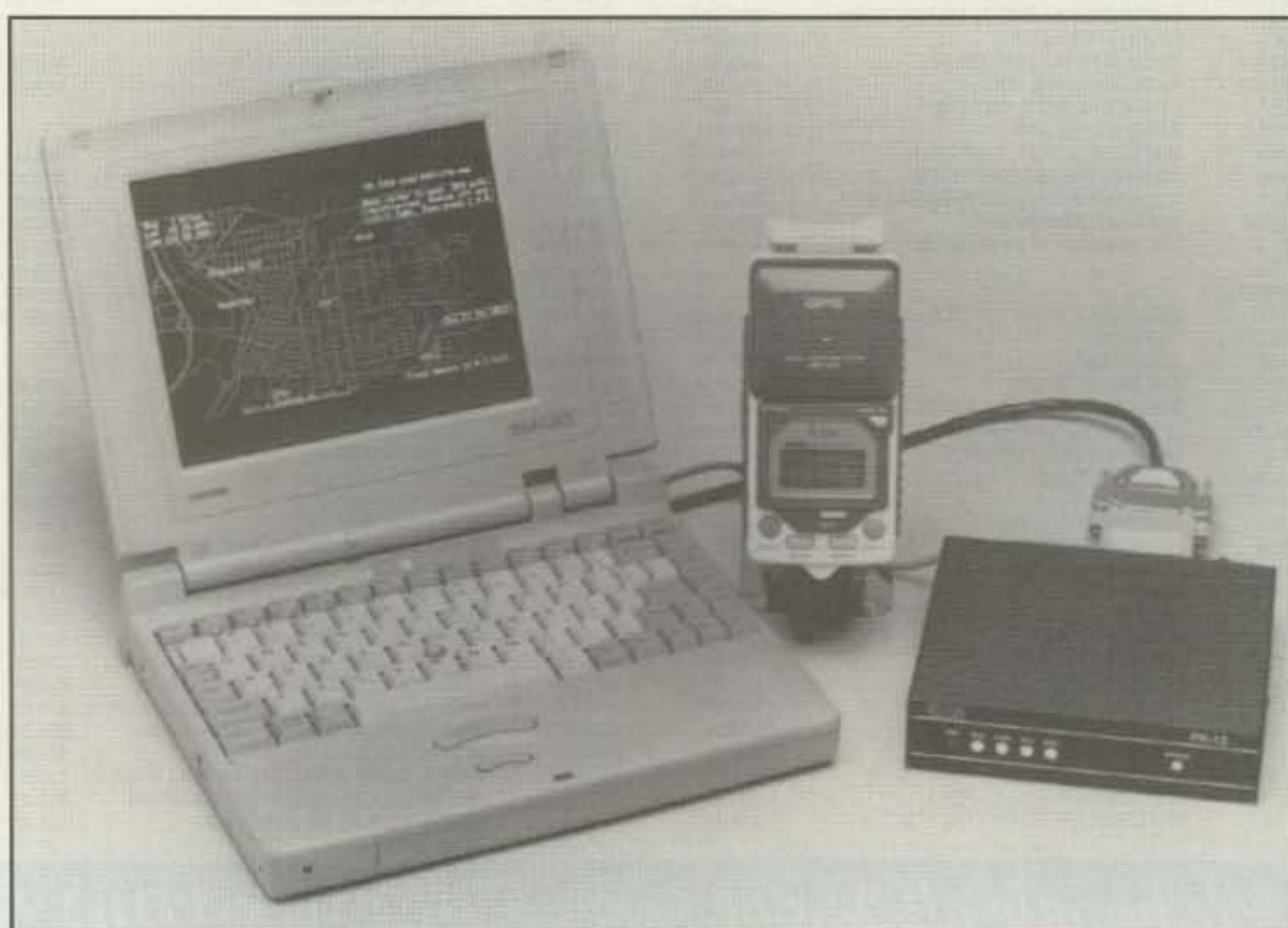
Photo 6- A full Global Positioning System capable of determining your location, plotting it on a related map, and automatically reporting it to others via packet radio. Units in the photo are a lap top computer, GPS receiver, and new AEA PK-12 packet controller with built-in APRS software.
