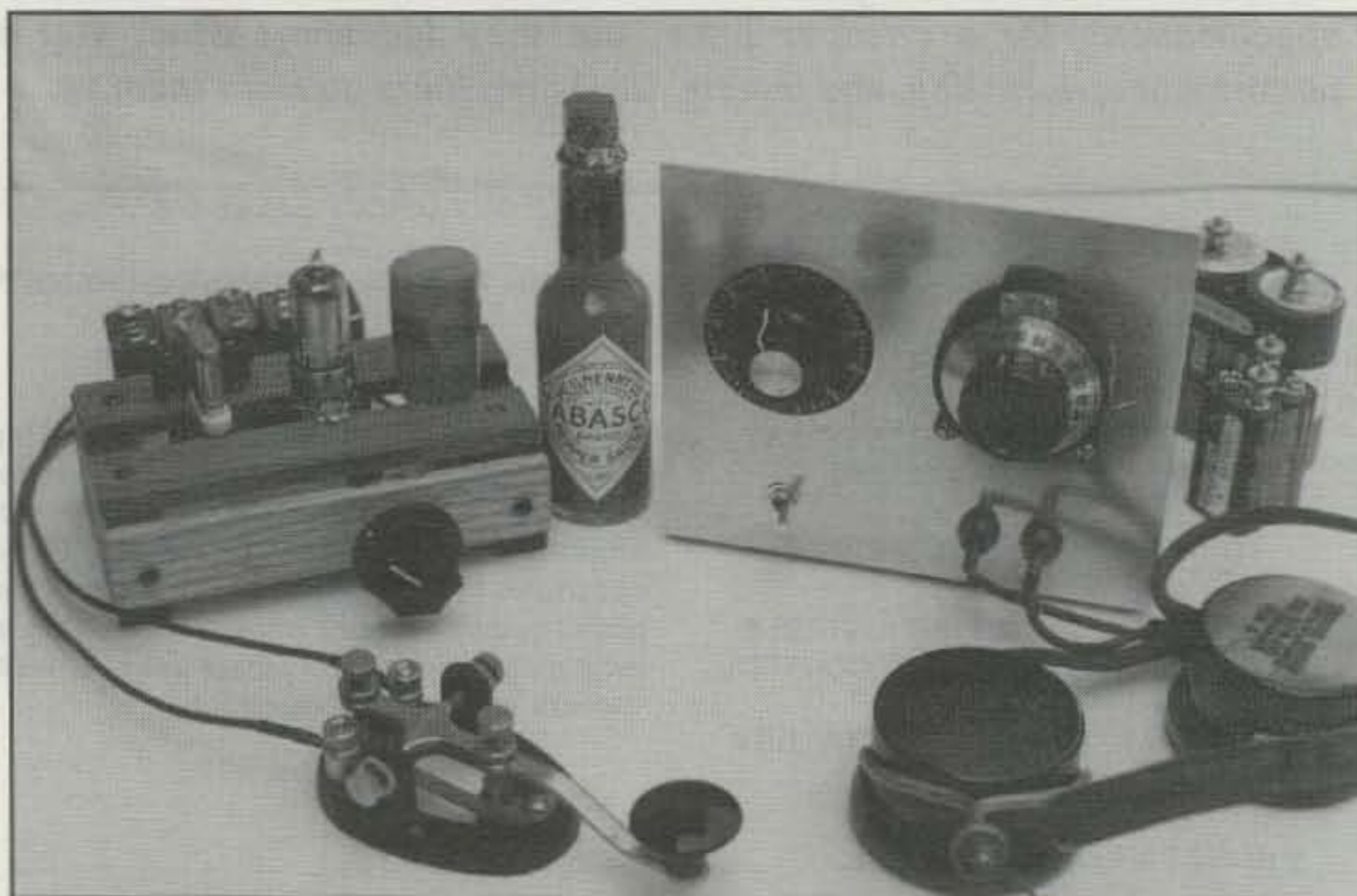
Fig. 1—Red-hot radio for sure! This zestful QRP setup consists of a one-tube regenerative receiver, Baldwin earphones, 500 milliwatt 1S4 transmitter, Speed-X key, and genuine Tabasco® sauce for flavor. Station is completely battery powered. (Thanks to Paul McIlhenney for permission to reference McIlhenney Company's famous Tabasco® brand pepper sauce.)
