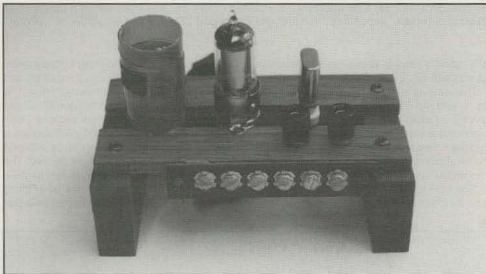
Fig. 7—Rear view of 1S4 transmitter showing layout of main parts. Photo was shot before unit was completely assembled.
