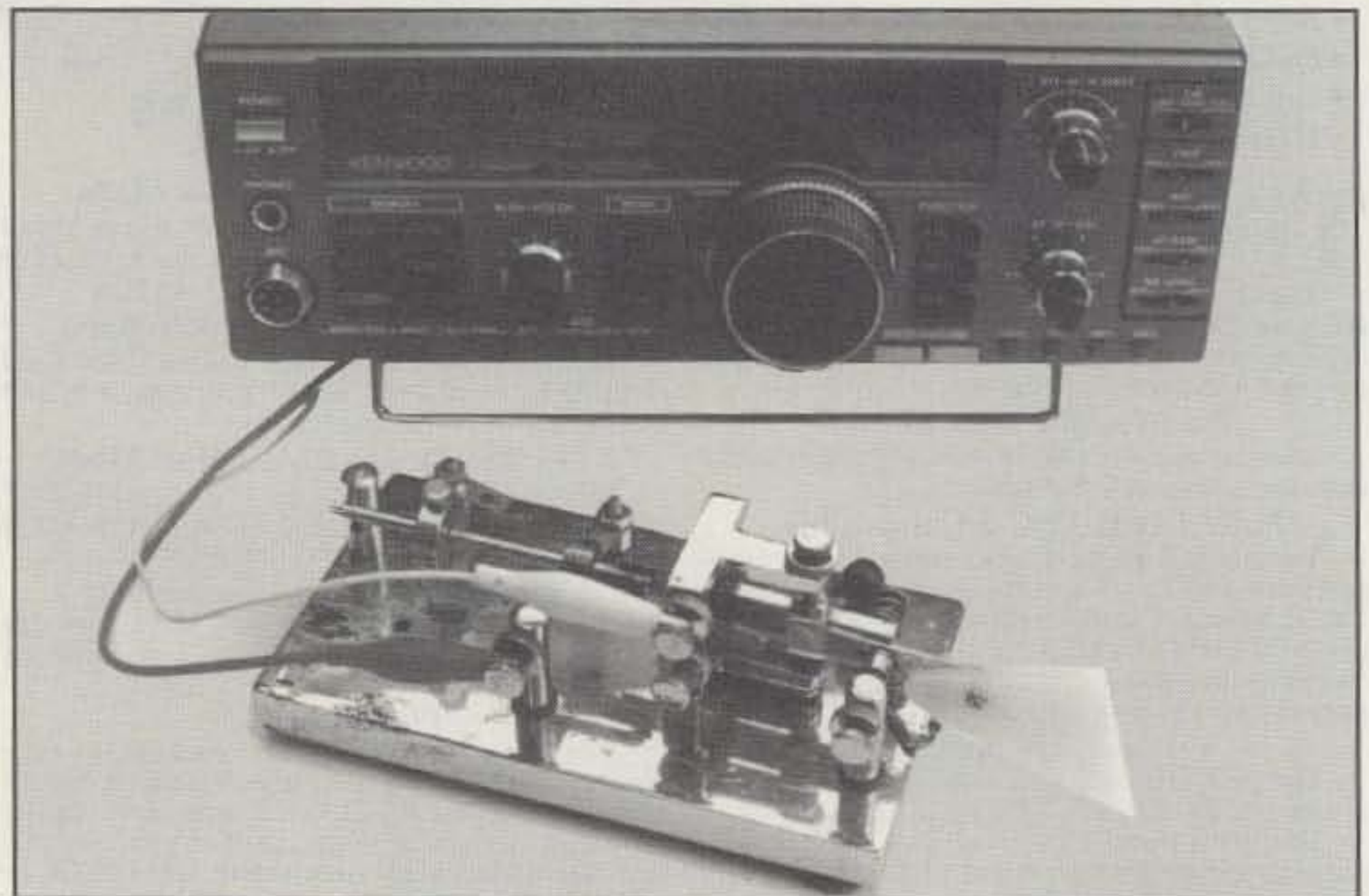
Photo 1—Clip leads are convenient for quick-checking a bug and troubleshooting bad connections. The Deluxe Speed-X shown here was an absolute basket case I thought would never clean up or work again. Now it is a delight to use (but still needs rechroming).
