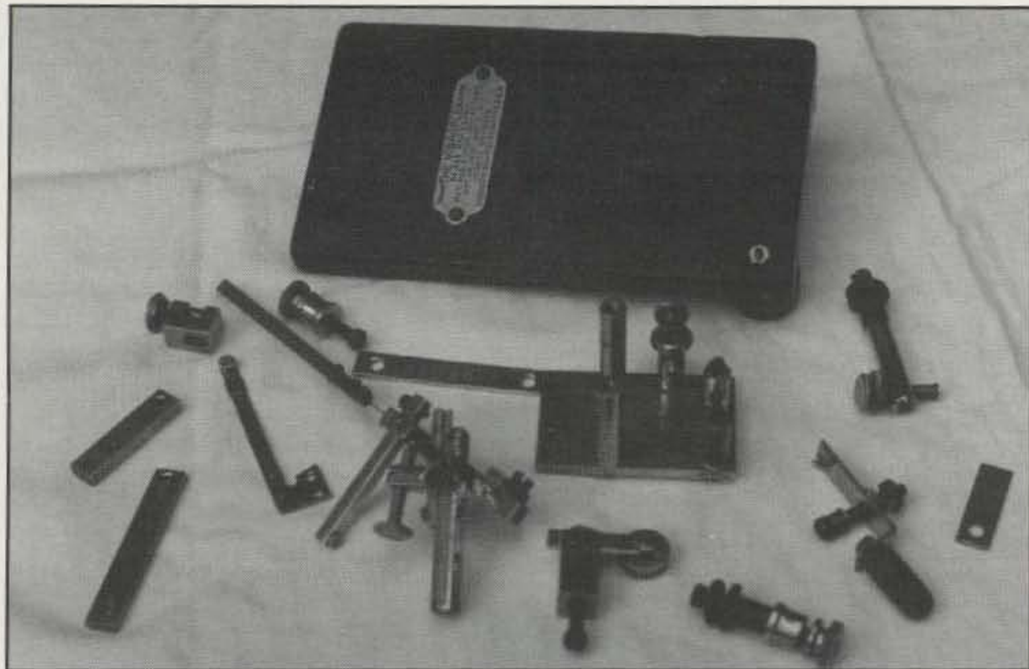
Photo 5- The Vibroplex model "X" shown disassembled here has just undergone refurbishing as described in text.
