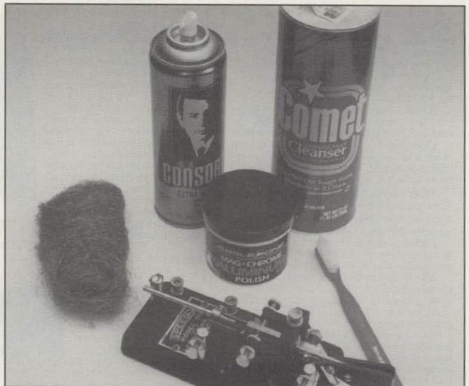
Photo 4— Main items/products used in "light refurbishing" of bugs, as discussed in text. I prefer retaining all possible authenticity, so except for springs, few parts are replaced/substituted.
