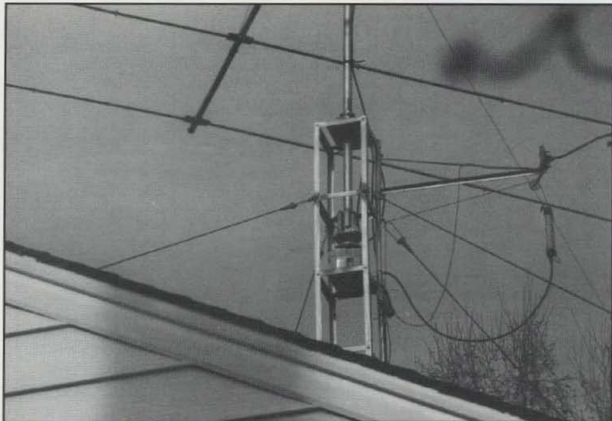
The rotator mounts to a standard 3" x 3" bolt pattern to fit inside many commercial towers.
