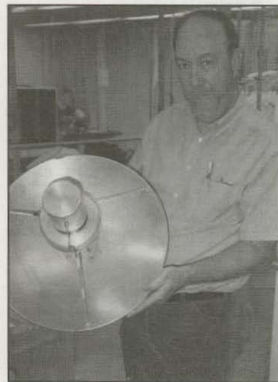
Photo B— In this AMSAT-NA photo Mike Garrity, N4OZC, displays a flight model prototype of the Phase 3D's S-band antenna. The new satellite will have a large array of transmitters, receivers, and antennas onboard for frequencies from 21 MHz to 24 GHz. (AMSAT-NA photo by Keith Baker, KB1SF)
