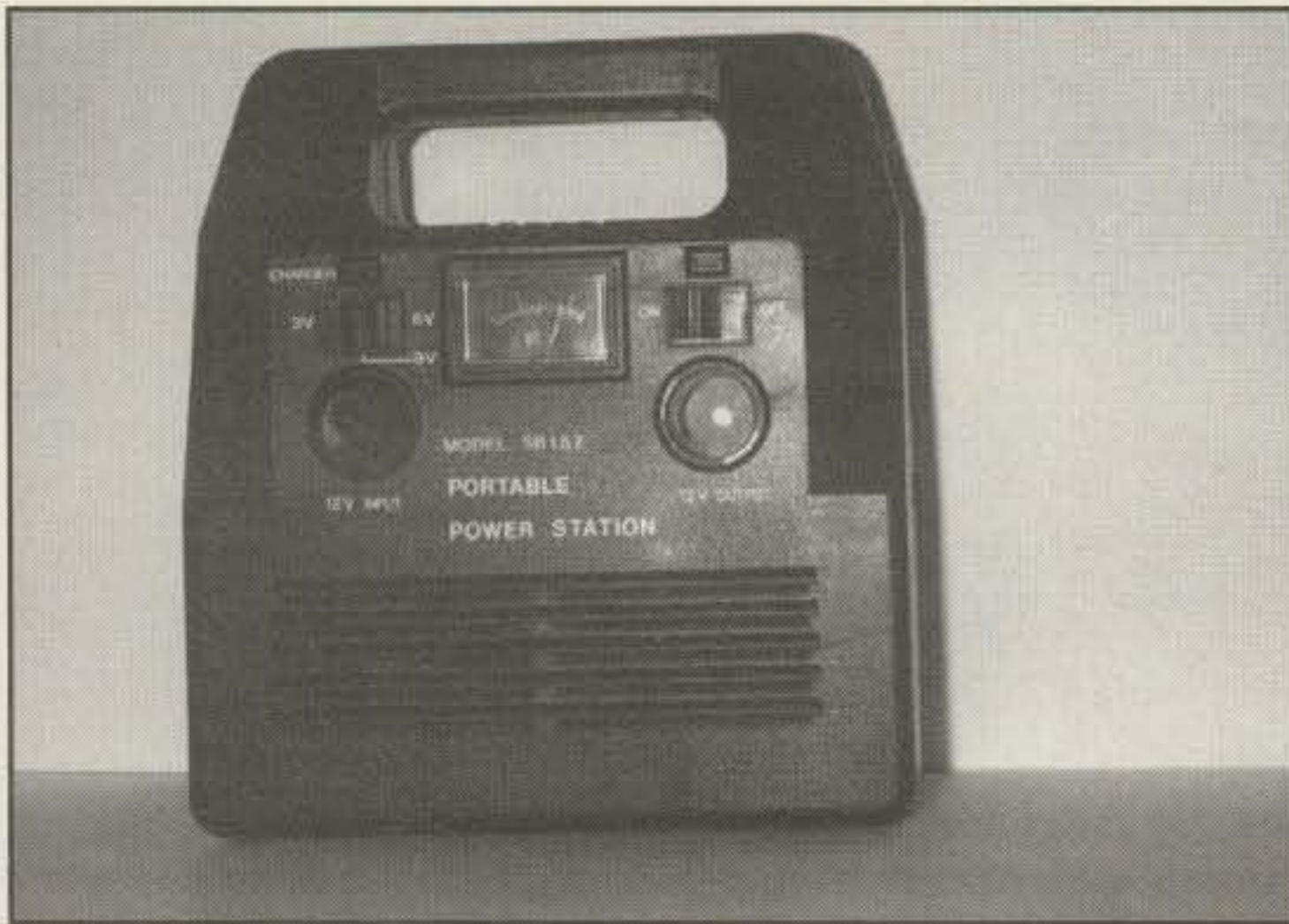
Photo 7— This fully self-contained 12 volt/7 amp battery pack is called the "Power Station," and it is hefty! See text discussion of combining it with a big mobile transceiver to make a super-power 2 meter portable rig.
