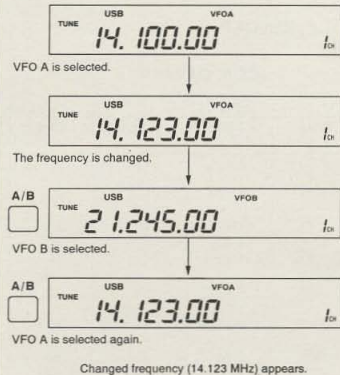
Fig. 1- From the instruction manual, these are the details on the VFO and MEMORY modes.
