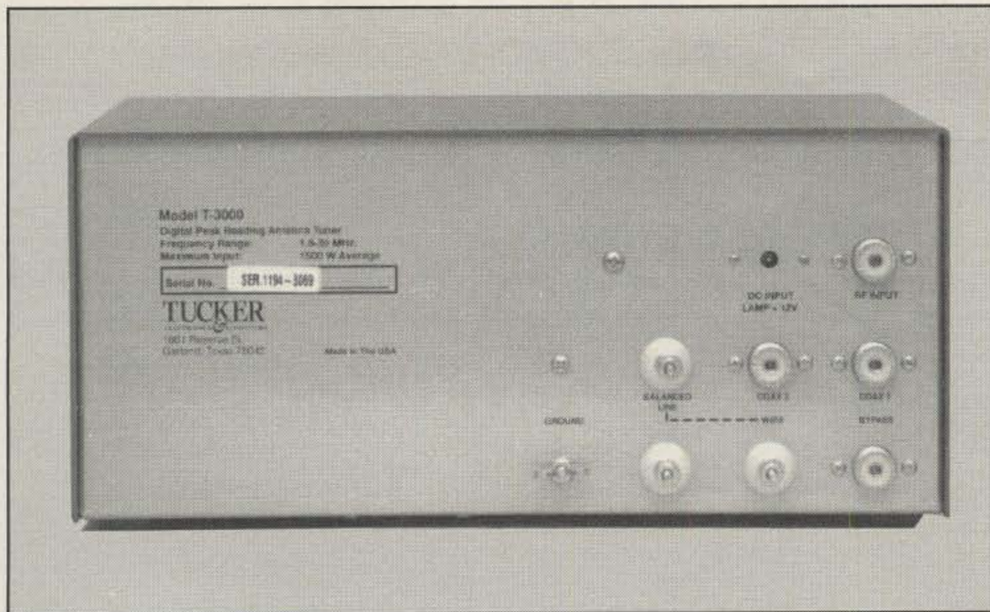
This back view shows the various antenna connectors. All of these terminals are capable of being switched from the front panel.
