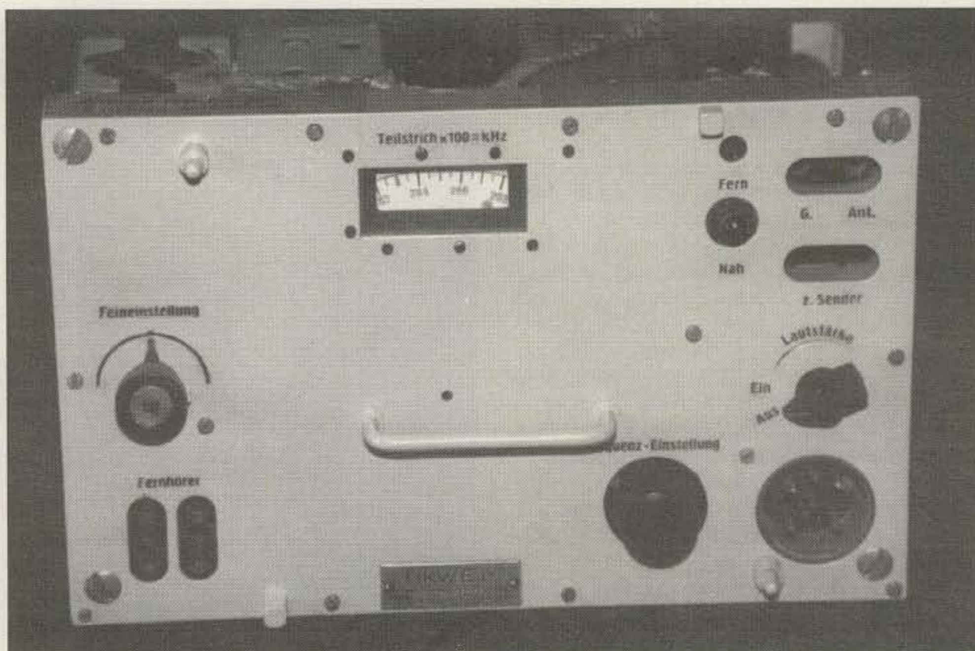
Fig. 2— Front view of the 10 meter German WW II Panzer tank receiver.
