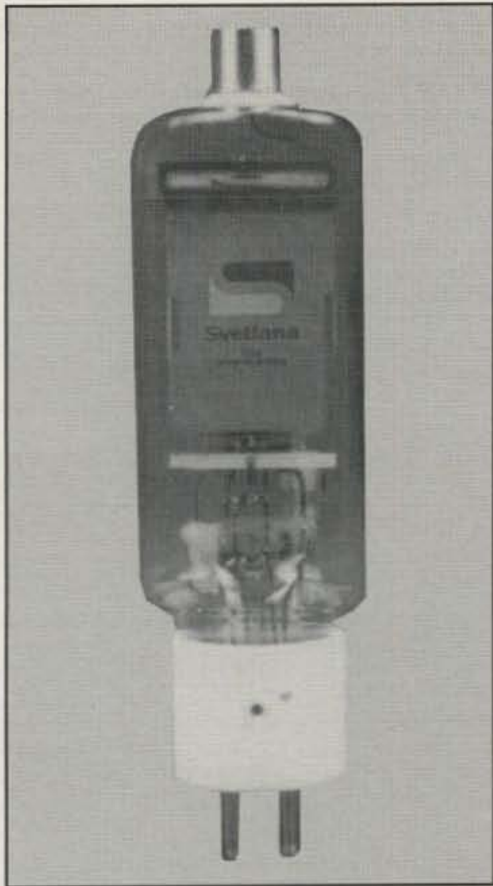
The Svetlana 572B, an updated version of the original 572B. It has a carbon anode plus a hard-glass envelope, intended for high-temperature operation.
