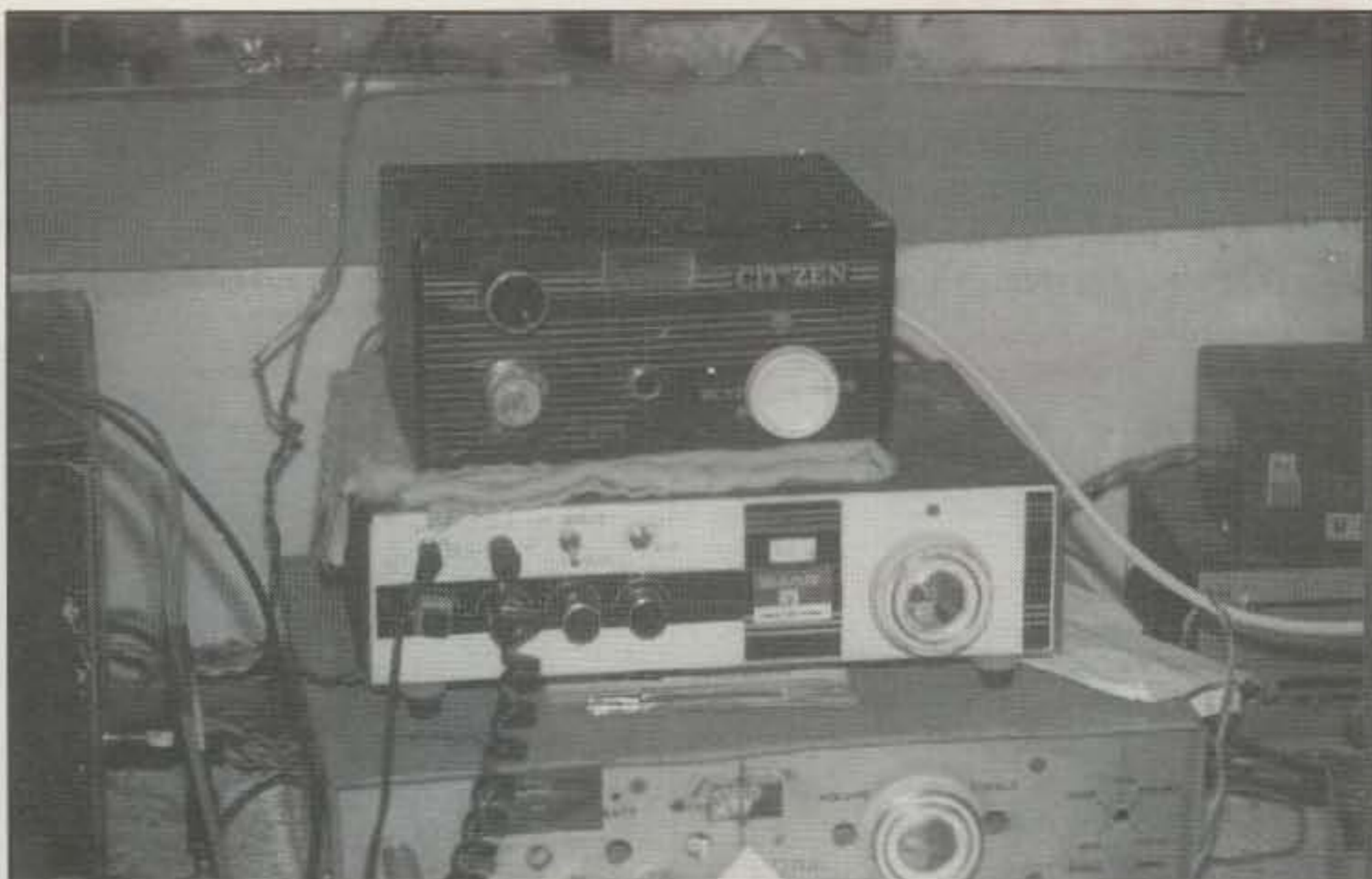
The 20 meter transceiver, AM/CW with direct-conversion receiver.
