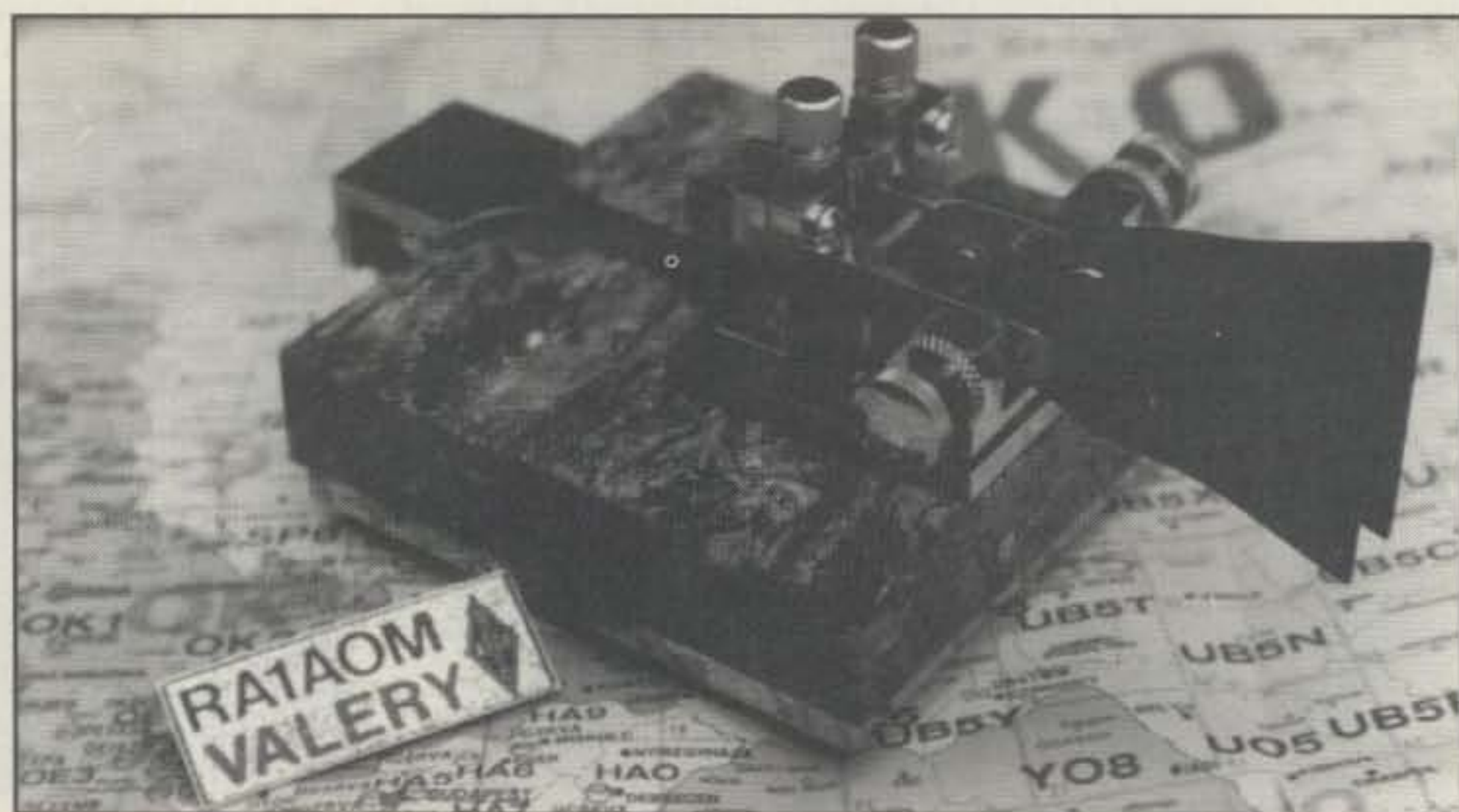
Photo 7— This remarkably smooth, precise paddle is made by Valery Pavlov, RA1AOM, and is a delight. Dot/dash contacts are in the middle (between levers), and adjustments on each side of the levers set travel/gap. Output connections are via a rear-mounted DIN socket.
