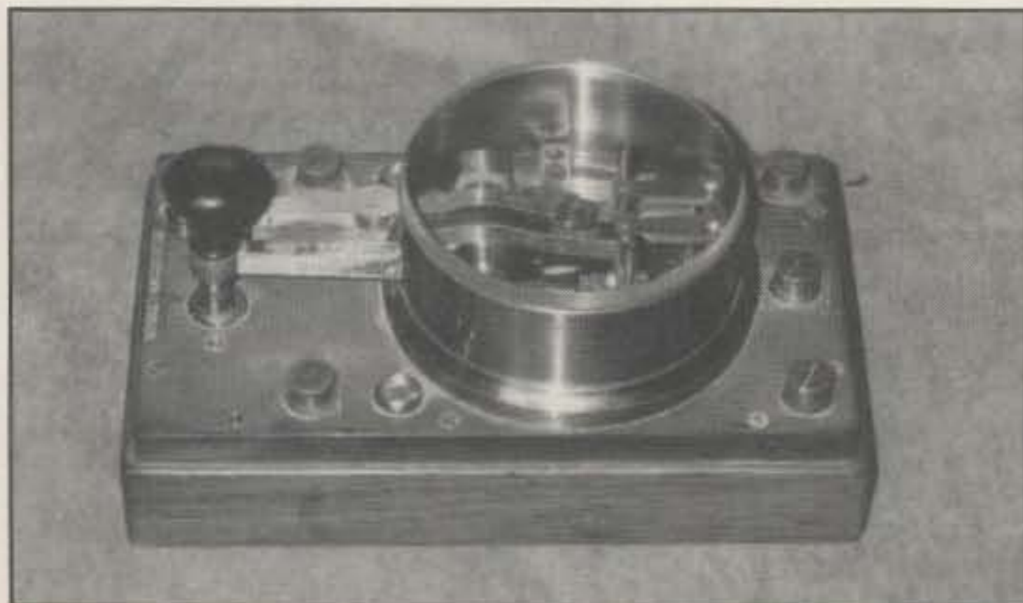
Photo 12—Unusual and quite rare Double Current Morse Key made by Silvertown Telegraph Works in the U.K. during the 1920s. This dazzler was used on two polarity landline setups (see text). (Photo courtesy Gustavo A. Coll of Uruguay) ▼
