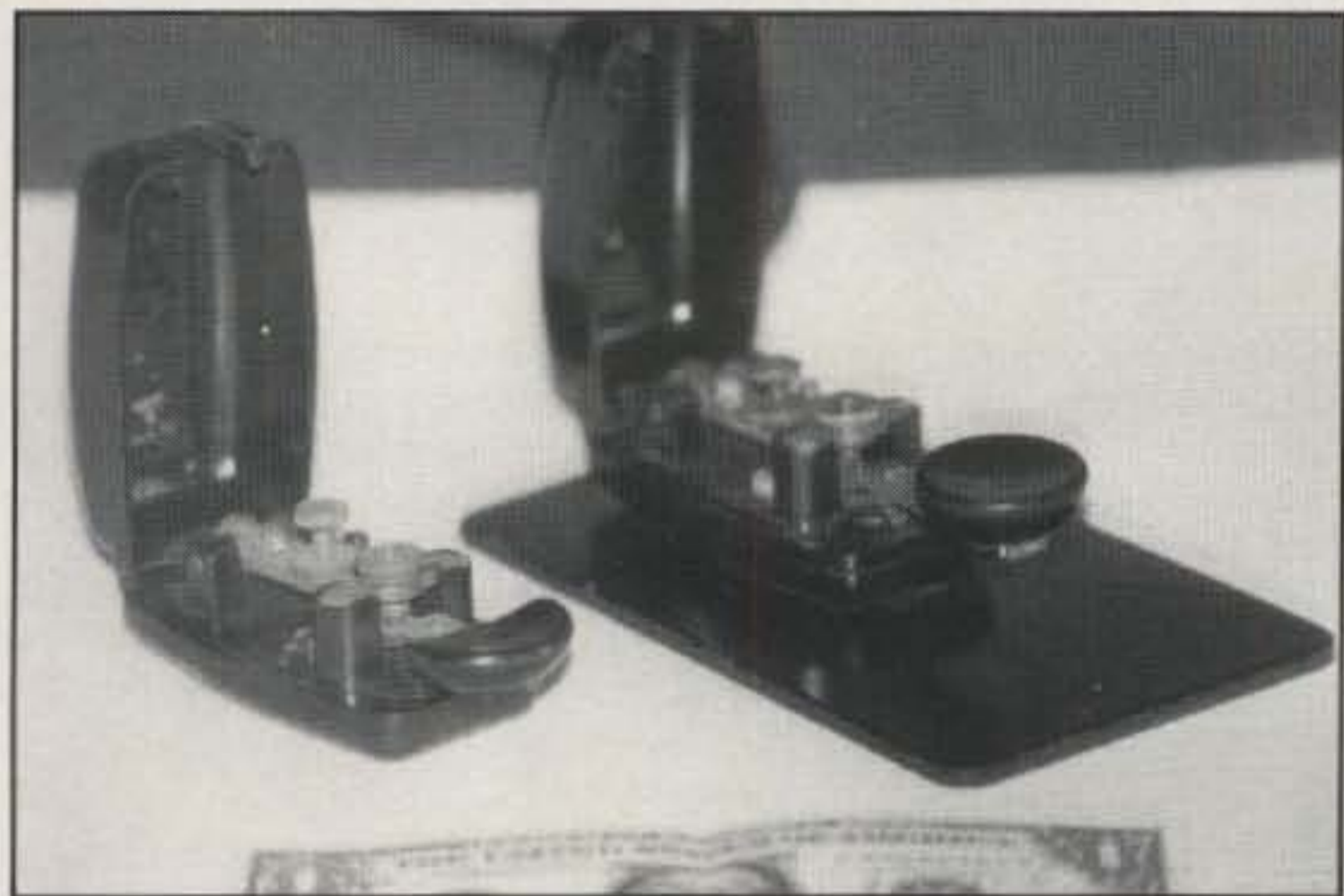
Photo 4— Two fine mice! Two popular varieties of German mouse keys are the half-knob and full-knob versions shown. Protective covers have been raised so you can study their mechanisms. The value of these collector's prides is rising every month. (Photo courtesy Peter, OK1CZ.)
