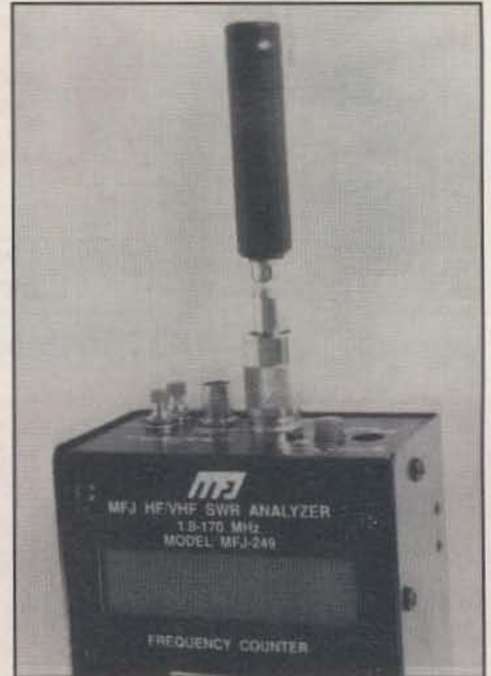
The MFJ-66 Dip Meter Adapter lets you turn your MFJ SWR Analyzer into a sensitive and accurate dip meter just by plugging in a coil. It also can be used to determine resonant frequencies of tuned circuits and measure the Q of coils. A set of two coils covers 1.8-170 MHz, depending on your analyzer. Here it's shown installed on an MFJ-249 HF/VHF SWR Analyzer. (Photo courtesy MFJ Enterprises, Inc.)
