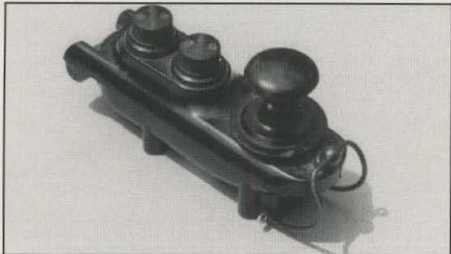
Photo 10- Captivating British-made Bathtub key (so named because of its appearance). Item reportedly was used on British aircraft during WW II. Two top screws (in front of knob) are binding posts for key cable. (Photo via W4PC.)
