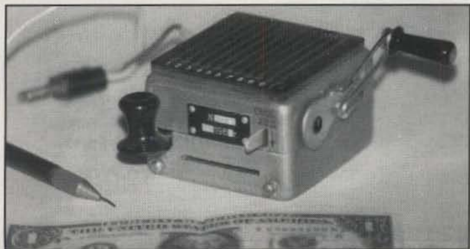
Photo 5— You are familiar with push-to-talk. Now meet crank-to-send! This little device was loaded with a prerecorded "Morse message on film," and used with a small spy transmitter. The faster the user turned the handle, the faster it sent CW. Note built-in key for sending impromptu messages. (Item owned and photographed by Peter, LK1CQ.)
