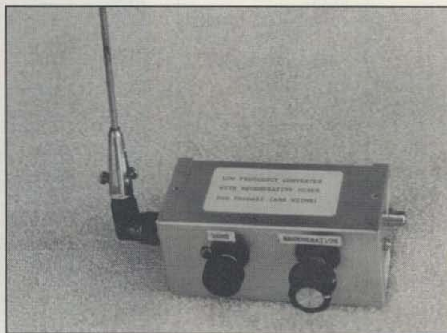
Most equipment used on the LowFERS and MedFERS bands is home-brew, and some easily constructed transmitting and receiving gear is described in The Low and Medium Frequency Radio Scrapbook offered by Ken Cornell, W2IMB. Shown here is an experimental LowFERS converter with a regenerative mixer and varactor tuning. It uses a short vertical whip antenna. (W2IMB photo)
