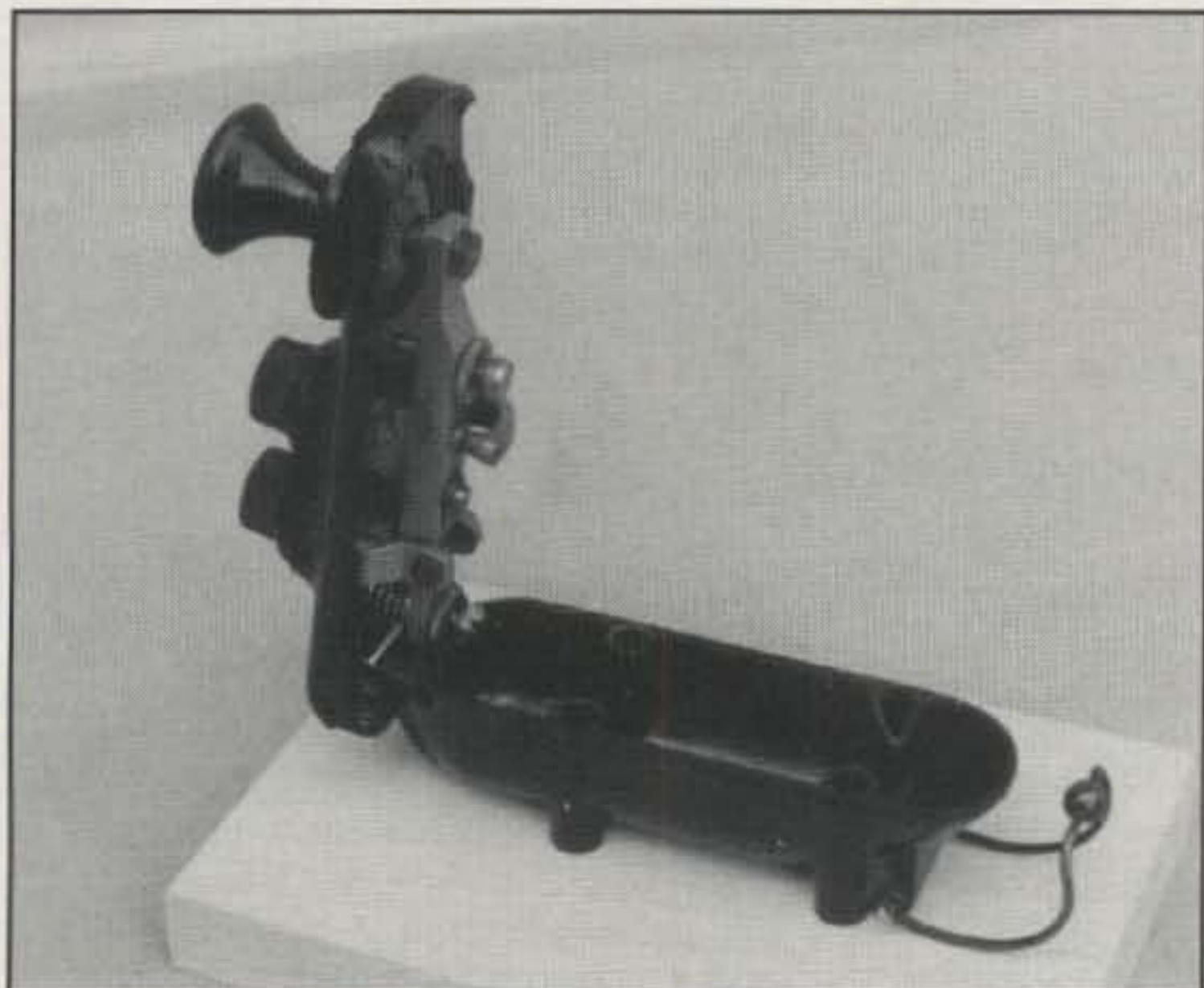
Photo 11- Interior view of Bathtub key. Mechanism is mounted upside-down on lid. Rubber grommet passing rod from knob to arm is also visible in this photo.
